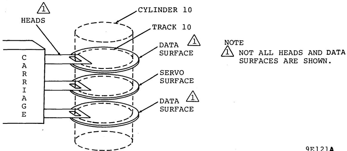
Figure 3-33. Cylinder Concept
