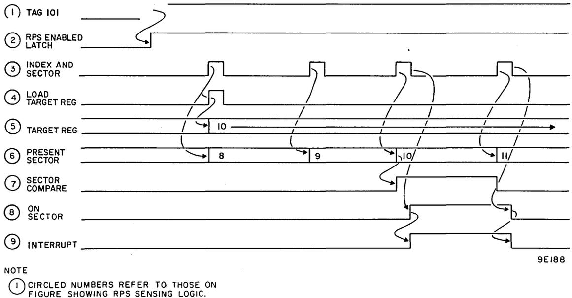
Figure 3-64. Rotational Position Sensing Timing
