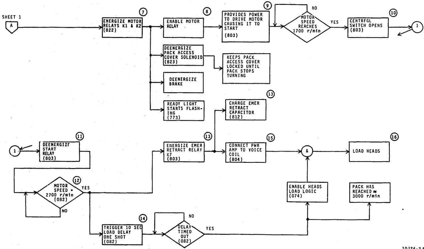
Provided all circuit breakers are closed, a pack is installed, and the access cover is closed, pressing the START switch:
