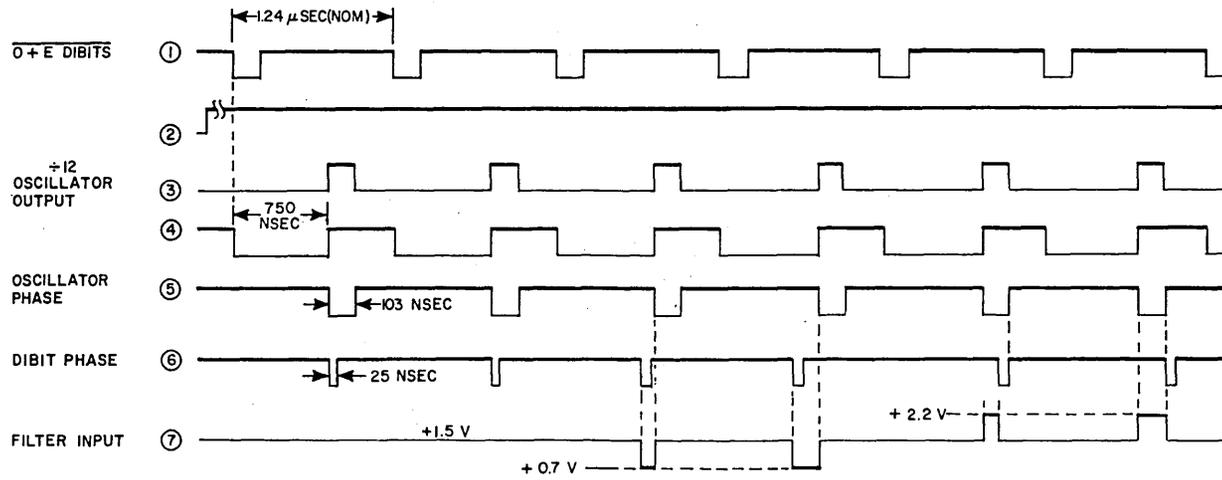
is used to enable the feedback pulses from the loop output to the input of the phase and frequency detector. The 1.6 us pulse is longer than the period of the nominal dibit frequency (806 KHz); therefore, the feedback pulses are continuously gated as long as dibits are present. The outputs from the detector are fixed amplitude pulses which are a function of the time (or phase) difference between the positive going edges of the two inputs (refer to figure 3-55).
