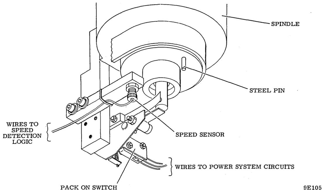
Figure 3-16. Speed Sensor and Pack On Switch Assemblies
