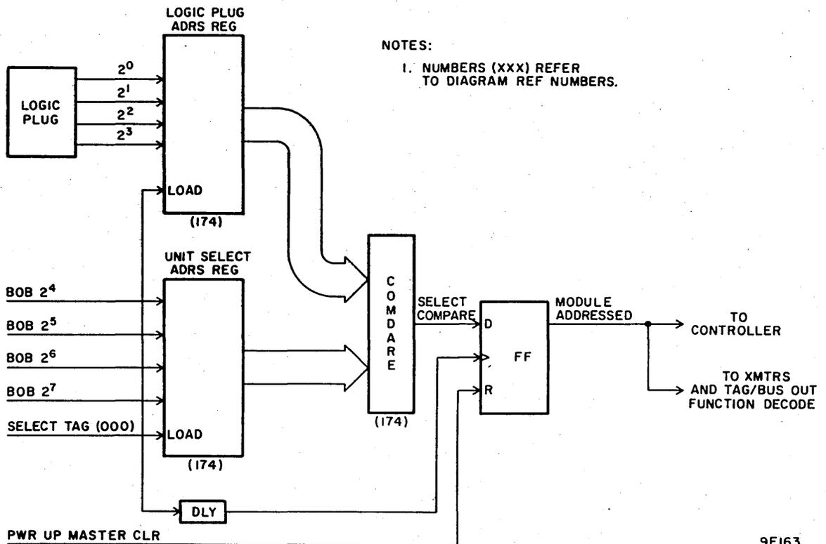
Figure 3-29. Unit Select Logic
