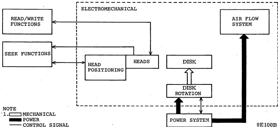
Figure 3-11. Electromechanical Functions Block Diagram
