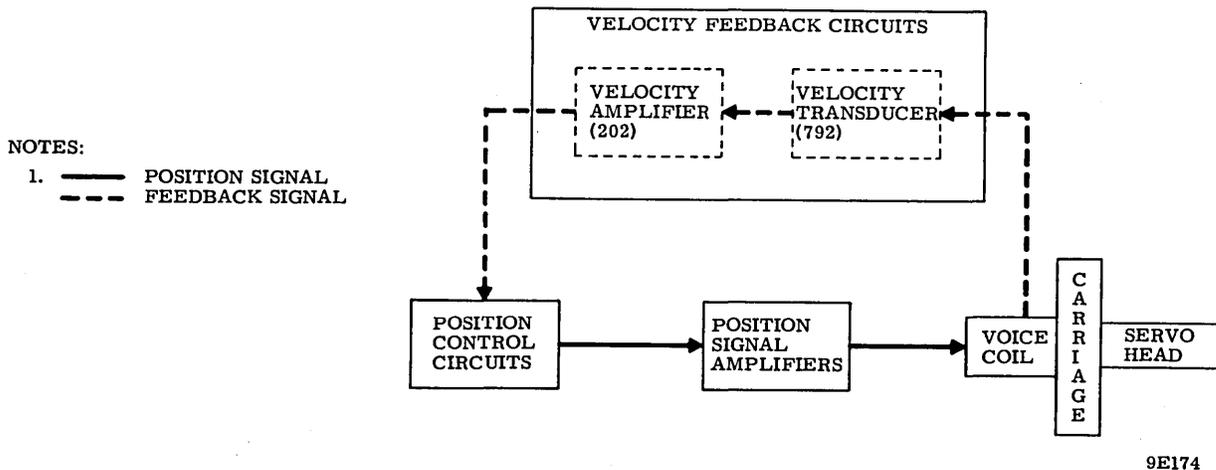
Figure 3-41. Velocity Feedback Circuits
