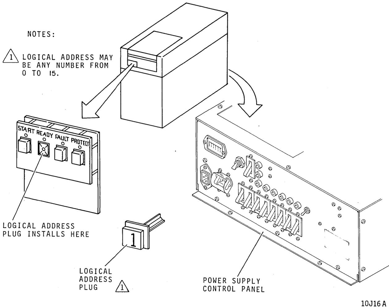
Figure 2-2. Controls and Indicators (VDE)
