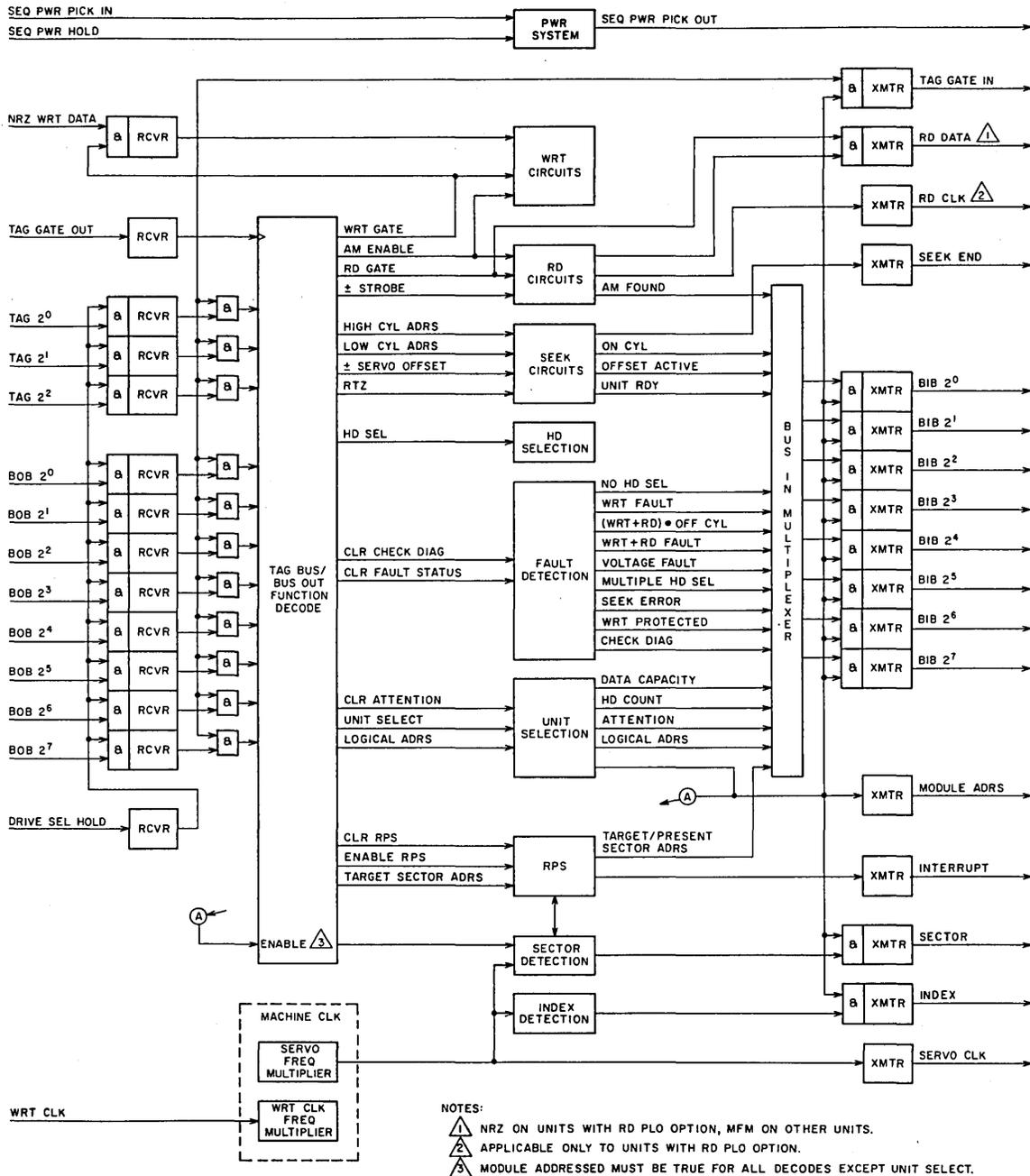
Figure 3-27. I/O Signal Processing Logic
