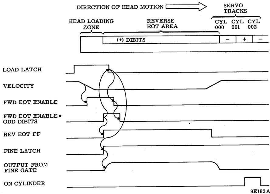
Figure 3-51. Load Seek Timing
