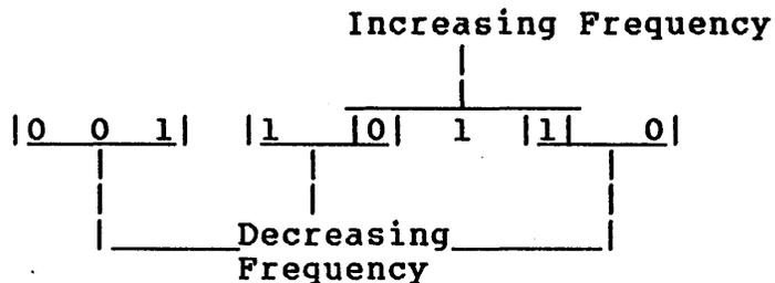
The outputs from the pattern decode logic enable either the Early, Late or Nominal gate (depending on the input frequency) to provide compensated Write data as follows:
