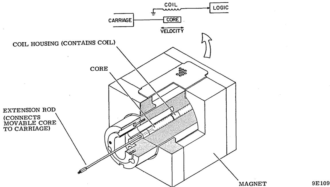
Figure 3-20. Velocity Transducer Assembly
