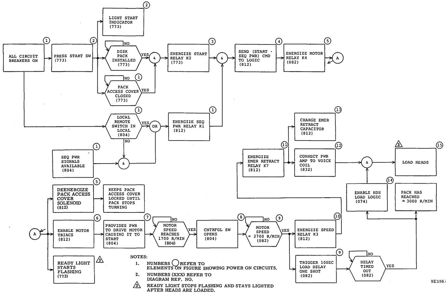
The sequence begins when either the START switch is pressed or the Sequence Power relay (K1) is de-energized. In either case the Start relay (K2) deenergizes and the RTZ logic is enabled (refer to discussion on Return to Zero Seeks). This causes the heads to move in the reverse direction and the READY light to start flashing.
