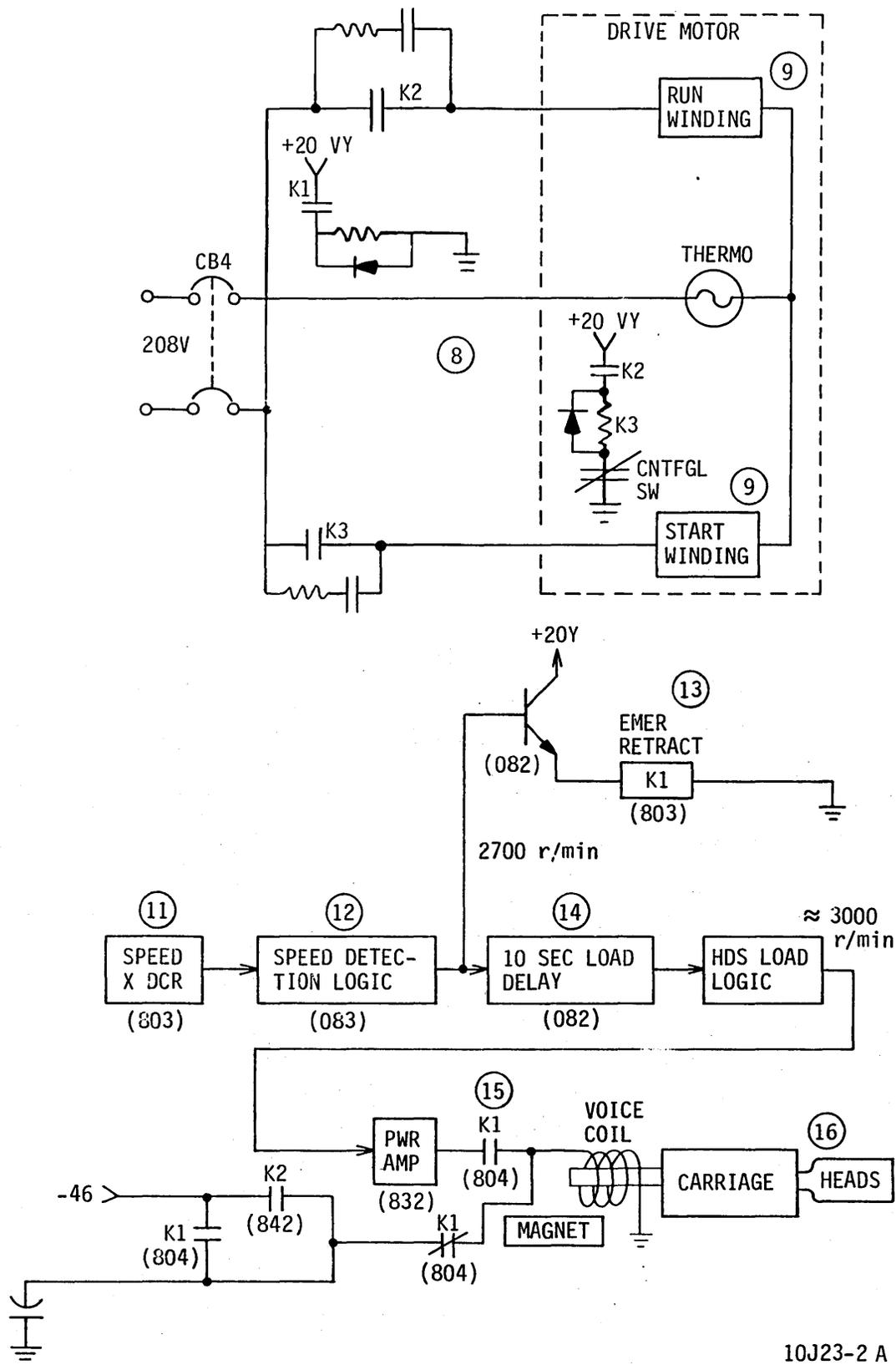
Figure 3-81. Power On Circuit (Sheet 2)
