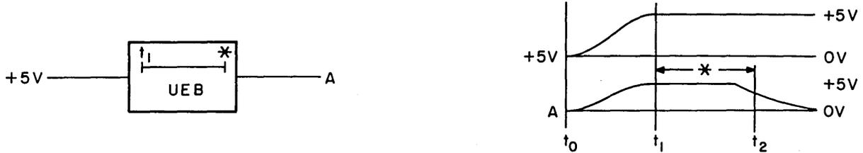
\* DELAY TIME VARIES WITH COMPONENT VALUES, SEE LOGIC DIAGRAMS FOR SPECIFIC DELAY TIME.
