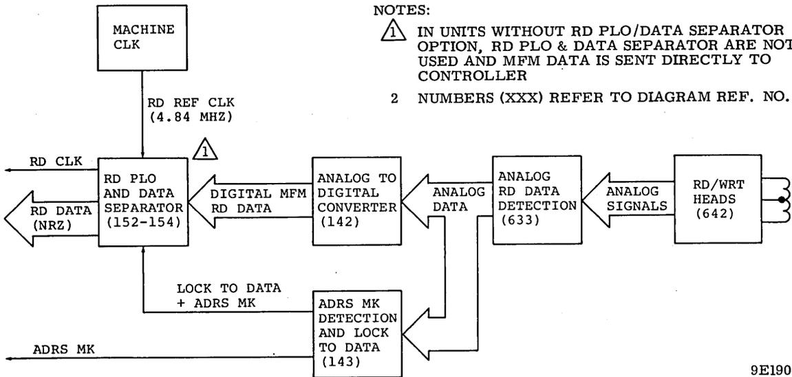
Figure 3-71. Read Circuits Block Diagram
