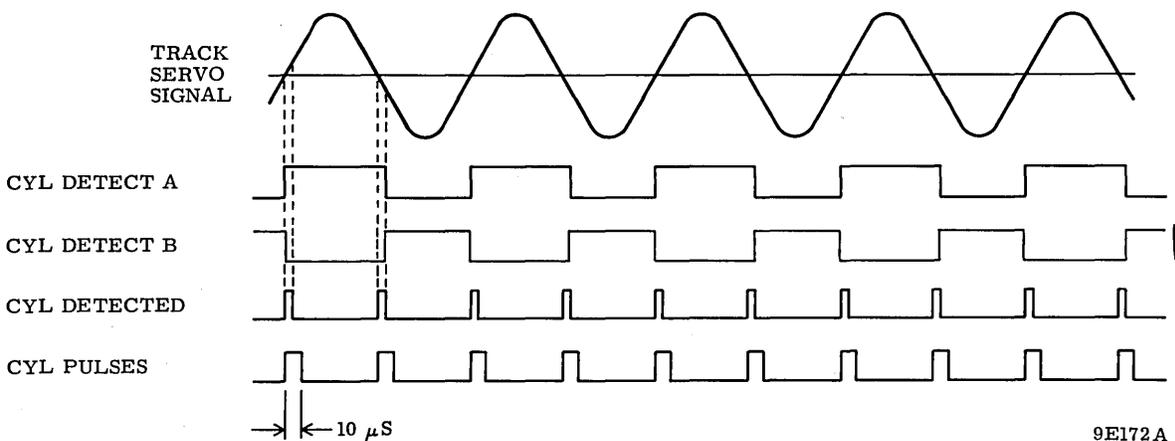
Figure 3-39. Cylinder Pulse Detection
