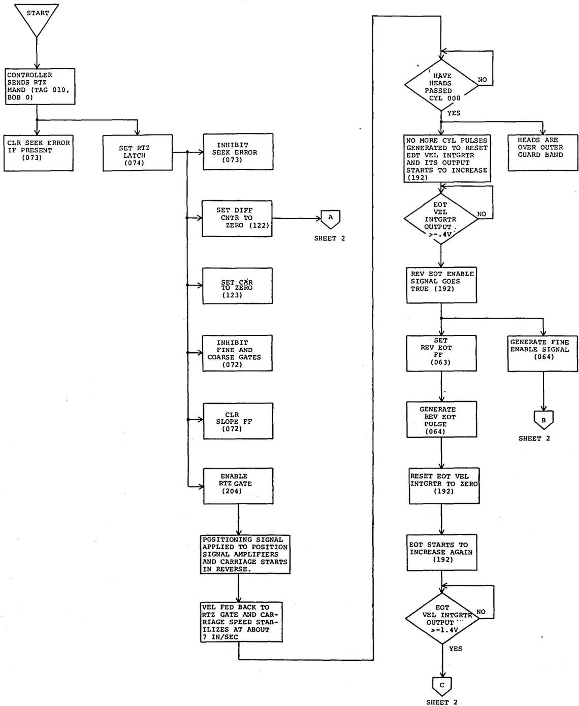
Figure 3-53. Return to Zero Seek Flow Chart (Sheet 1 of 2)
