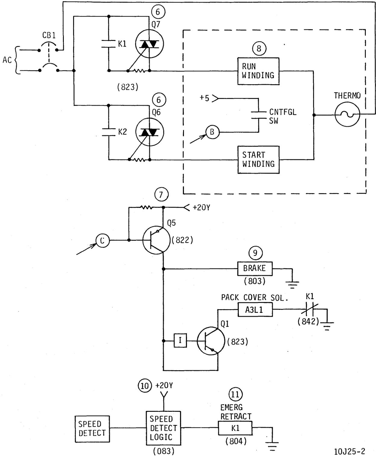
Figure 3-83. Power Off Circuits (Sheet 2)
