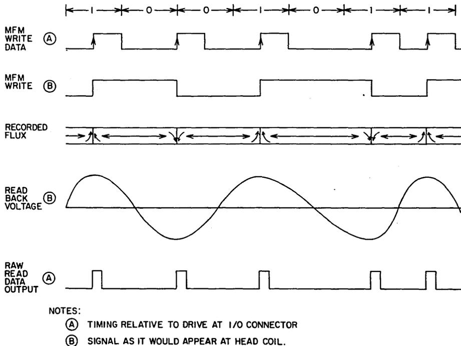
Figure 3-67. MFM Recording - Waveforms and Timing
