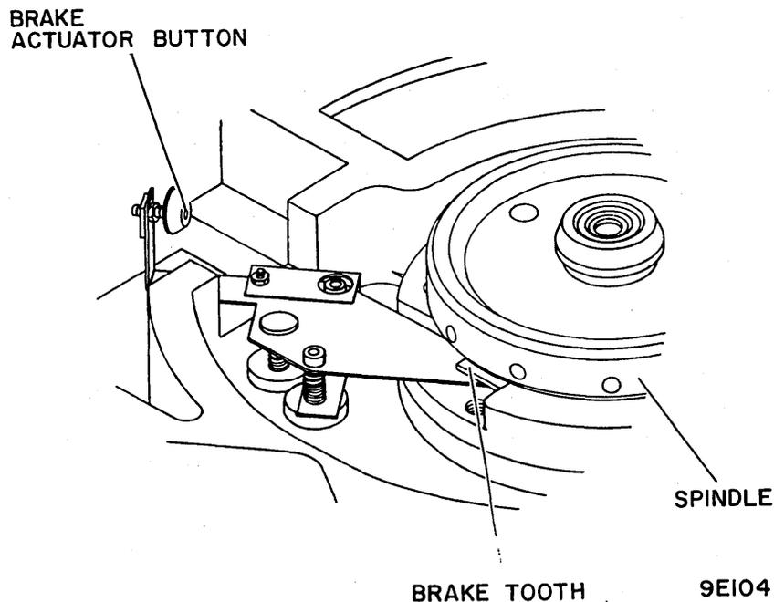
Figure 3-15. Parking Brake Assembly
