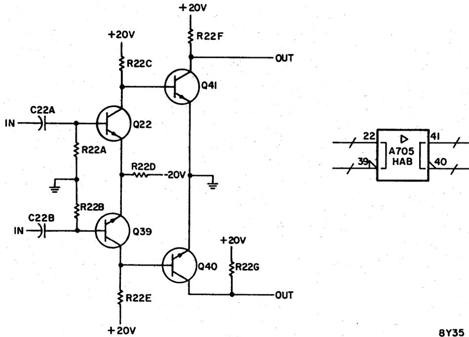
Figure 4-1. Typical Discrete Component Circuit Schematic
