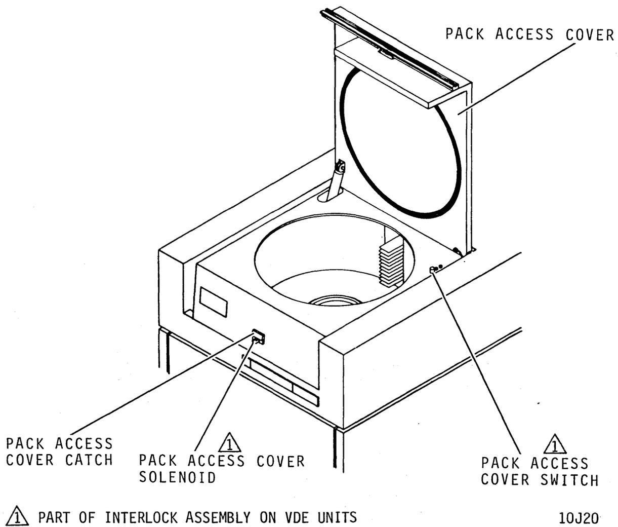
Figure 3-17. Pack Access Cover Switch and Solenoid
