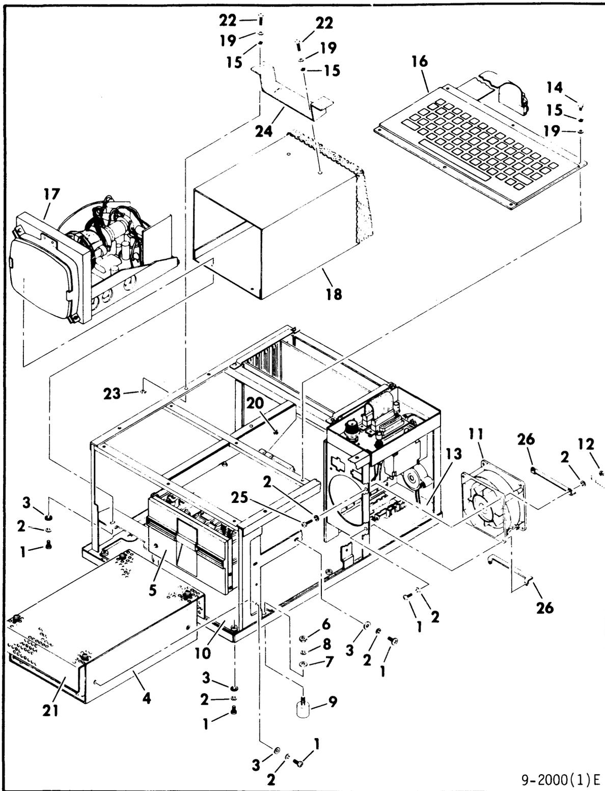
Figure 3A-2. Chassis Assembly (Sheet 1 of 5)
