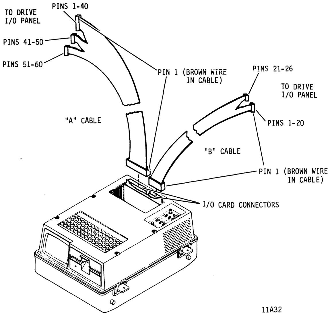
Figure 2-3. I/O Cable Attachment
