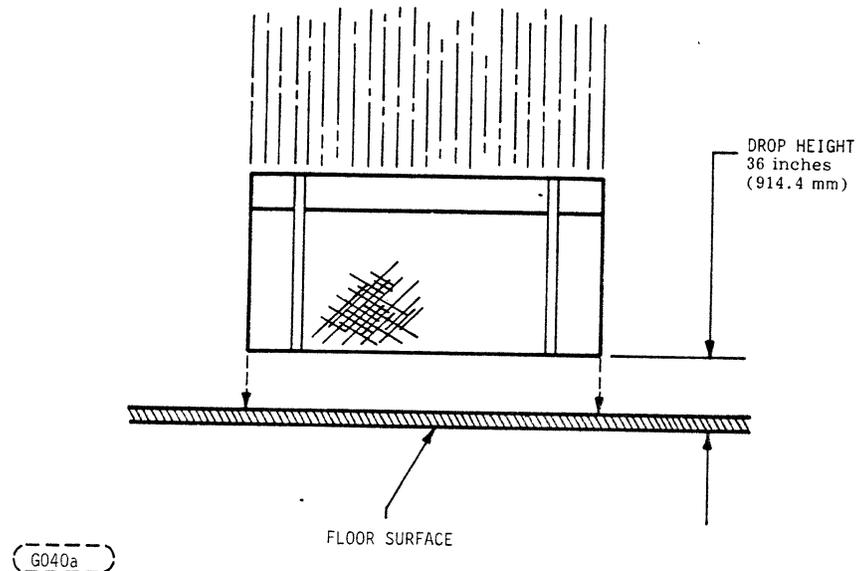
Figure 6. Flat Drop Test
