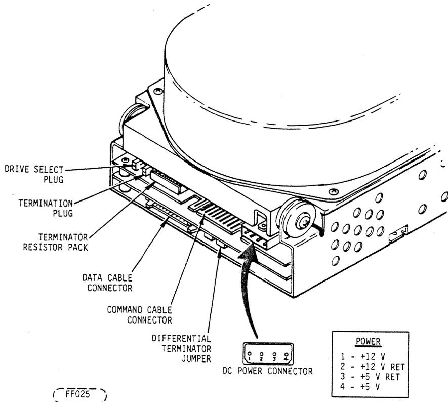
Figure 10. WREN I/O Connection
