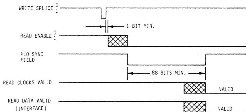
READ ENABLE MUST BE DEACTIVATED PRIOR TO THE WRITE SPLICE. READ ENABLE MAY BE REINITIATED AT LEAST ONE BIT AFTER THE WRITE SPLICE AND WITH AT LEAST 11 BYTES OF PLO SYNC REMAINING IN THE SYNC FIELD. THE 12 BYTE EXAMPLE CONSISTS OF ONE BYTE OF WRITE SPLICE AND 11 BYTES FOR PLO SYNC.
