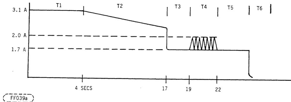
Figure 4. Typical 9415-3 WREN +12 V Current Profile
