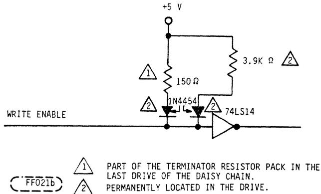
Figure 13. Write Enable Termination
