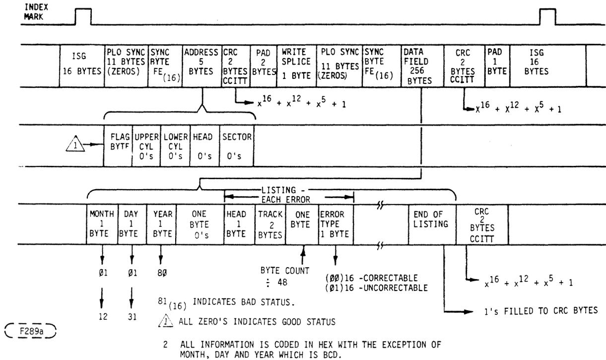
Figure 8. Format for Surface 0, Track 656, Sector 0--
