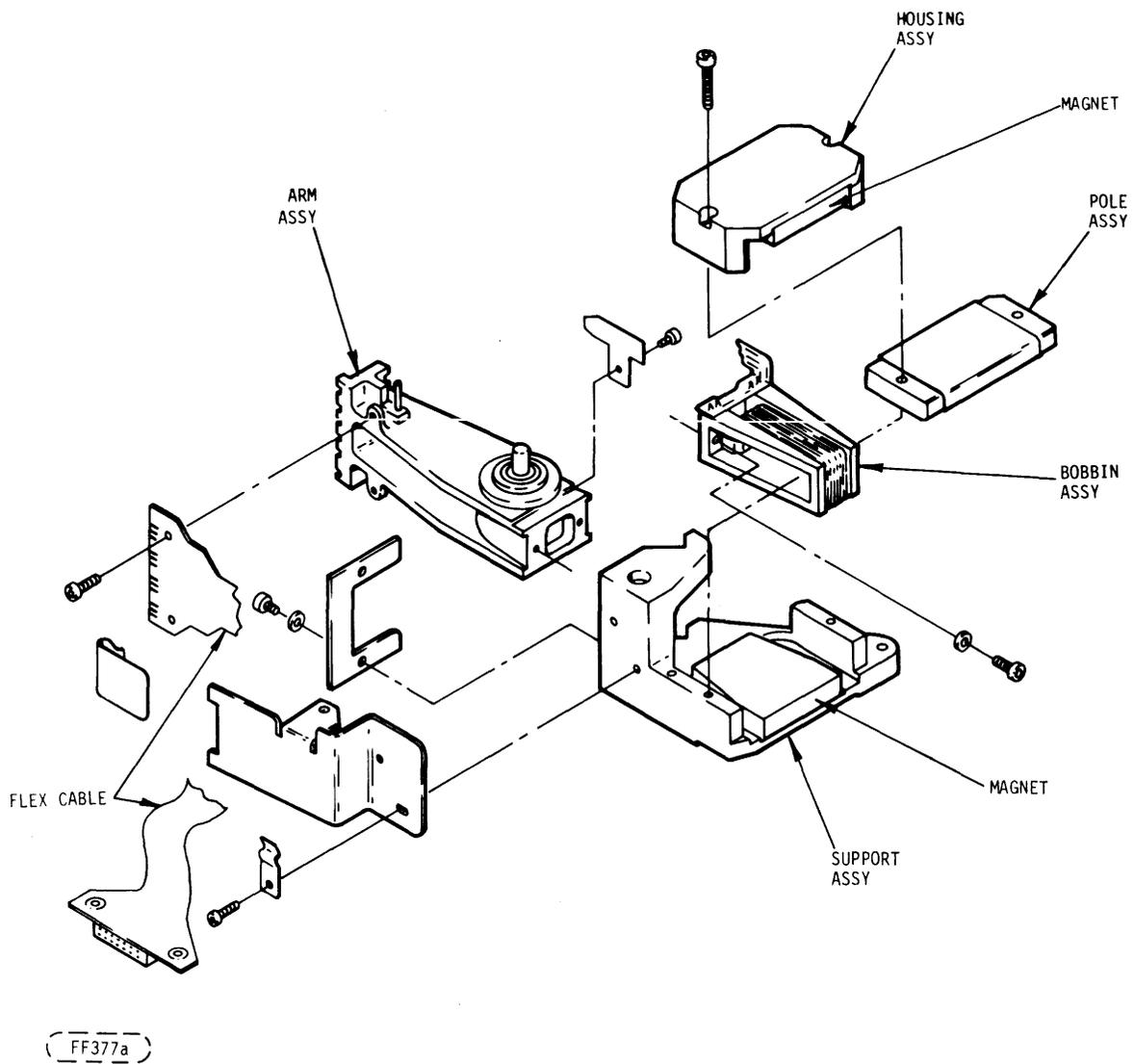
FIGURE 4-3. WREN ACTUATOR ASSEMBLY
