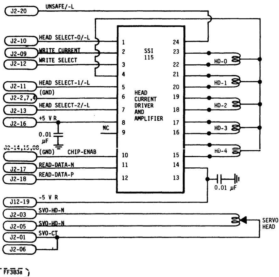
FIGURE 4-29. HEAD PREAMP AND DRIVER (AT THE FLEX CABLE)
