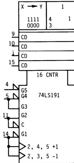
THE 74LS191 IS A SYNCHRONOUS UP/DOWN COUNTER. EACH STAGE HAS AN INPUT AND AN OUTPUT PIN AS FOLLOWS:
