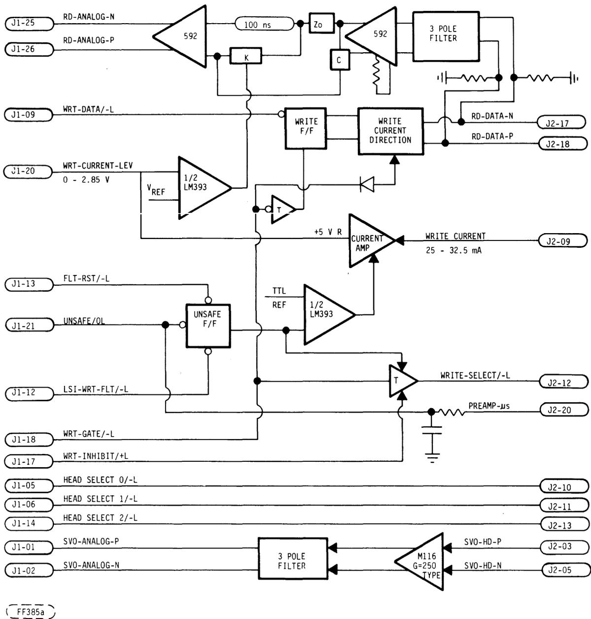
FIGURE 4-25. PRE-AMP BLOCK DIAGRAM
