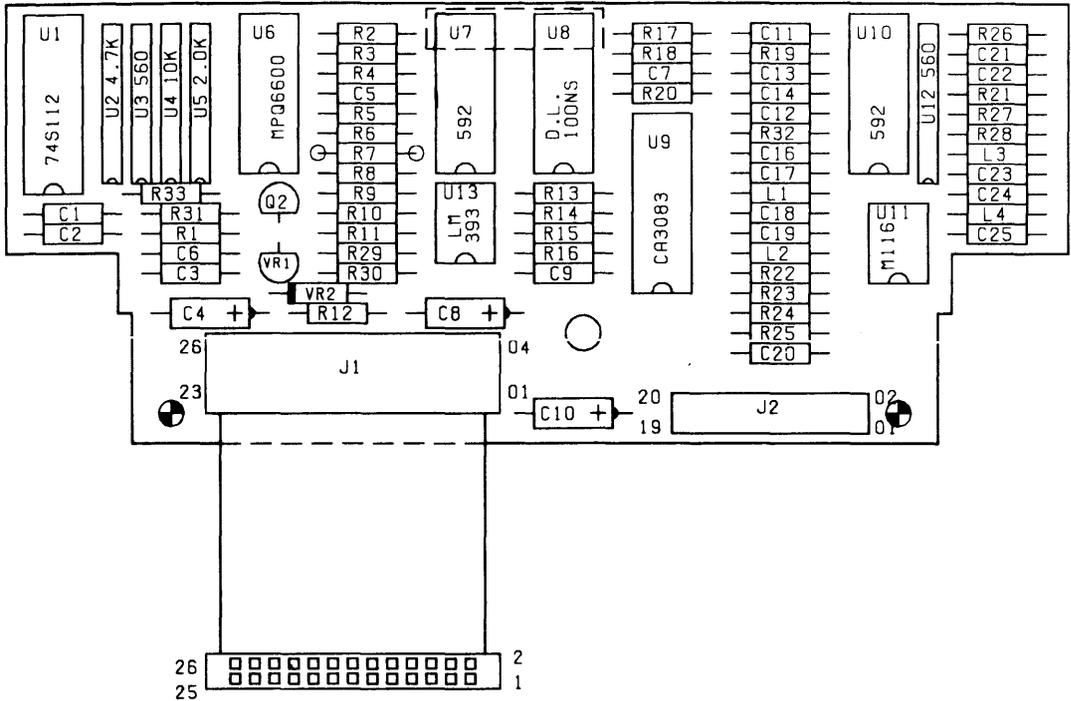
FIGURE 5-7. R/W PREAMP PWA (SHEET 3 OF 3)
