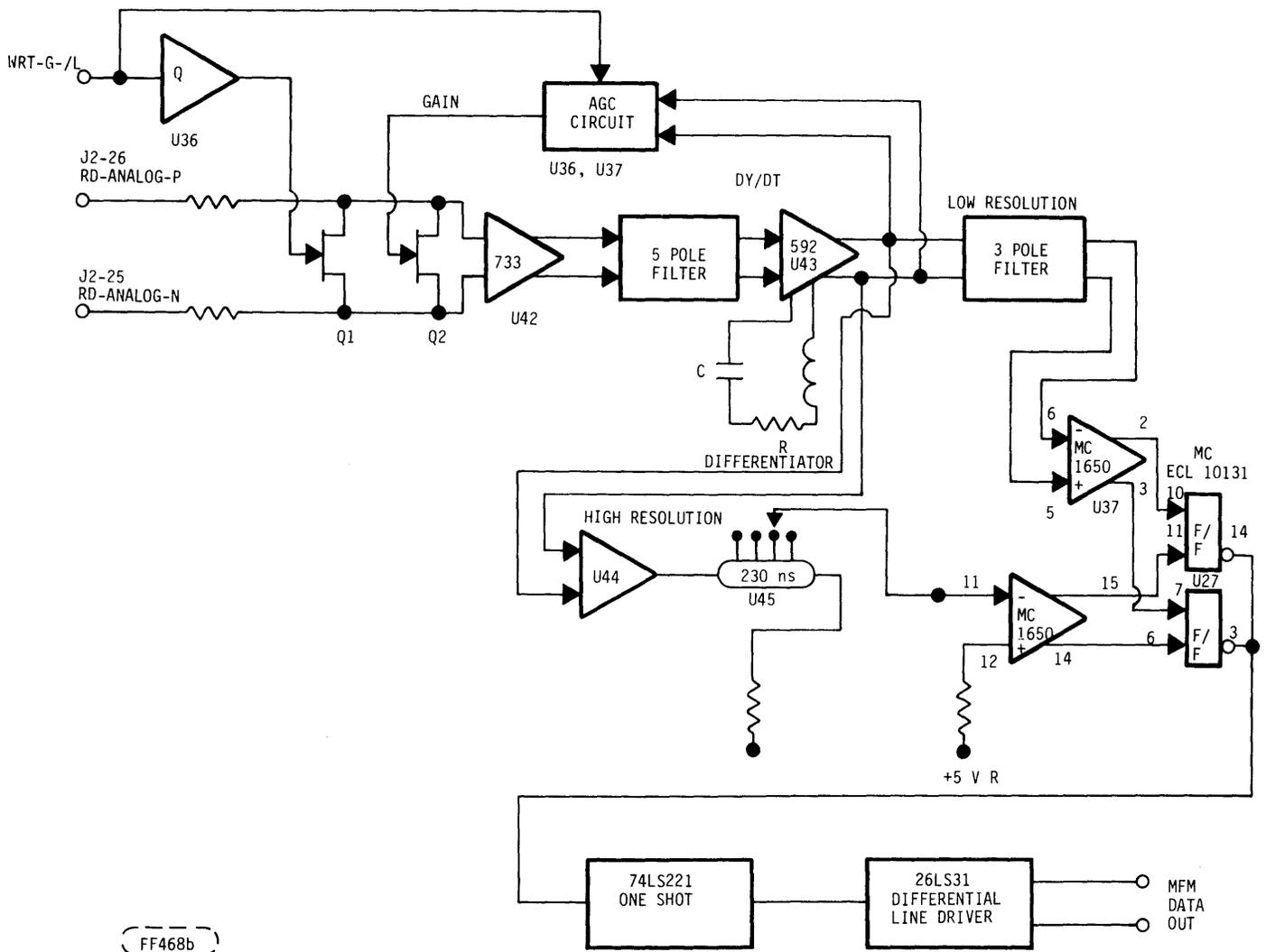
FIGURE 4-26. DATA PWA READ ANALOG FUNCTION
