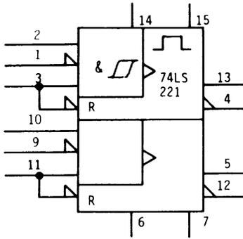
THE 74LS221 IS A DUAL MONOSTABLE MULTIVIBRATOR WITH SCHMITT TRIGGER INPUTS. THE TWO SECTIONS ARE INDEPENDENT EXCEPT FOR A COMMON POWER SOURCE.
