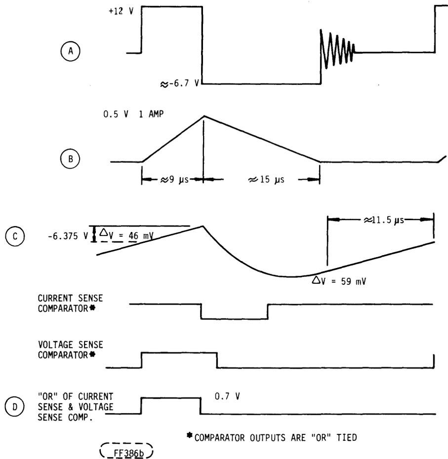
FIGURE 4-32. DC-DC CONVERTER WAVEFORMS
