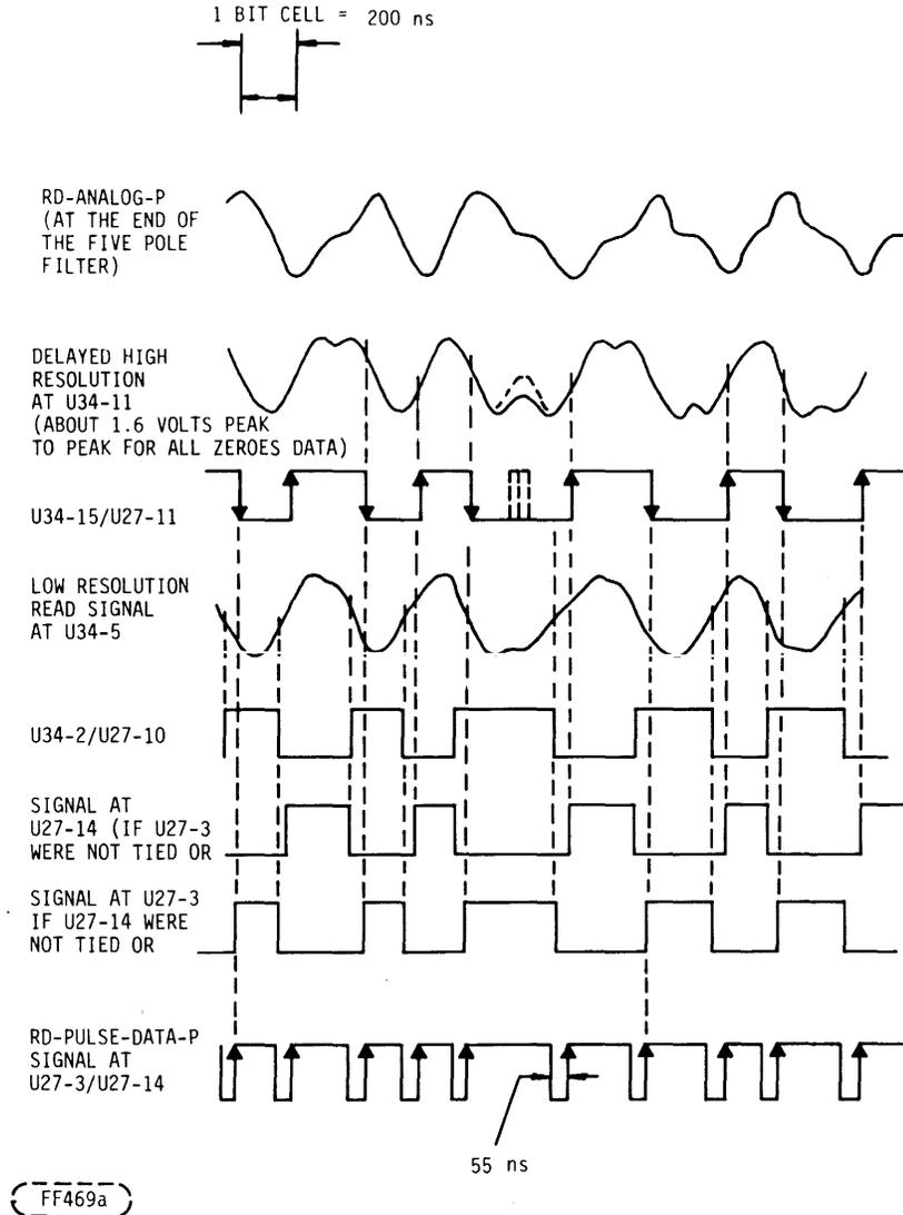
FIGURE 4-27. READ ANALOG TIMING DIAGRAM
