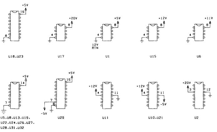
FIGURE 5-5. SERVO SCHEMATIC (SHEET 2 OF 9)
