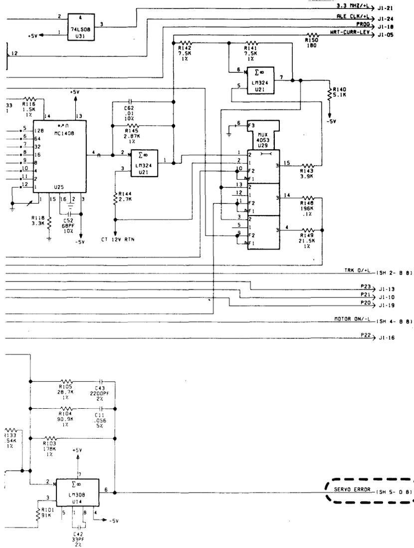
FIGURE 5-2. SERVO SCHEMATIC (SHEET 3)
