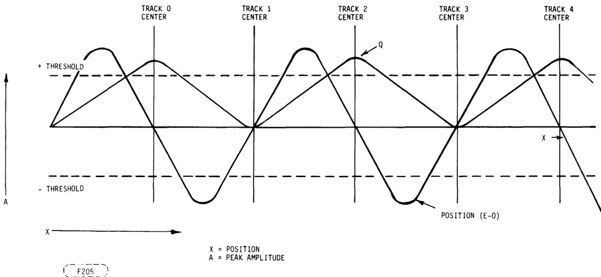
FIGURE 4-22. DERIVED POSITION AND QUADRATURE SIGNALS
