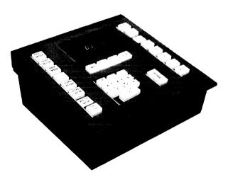
The operator keyboard is a switch-actuated data entry device. Each time a numeric key is depressed, the octal code for that key enters the lowest octal position of the keyboard register. The operator keyboard enables storing data in memory by supplying the initial memory address and data for storage.
