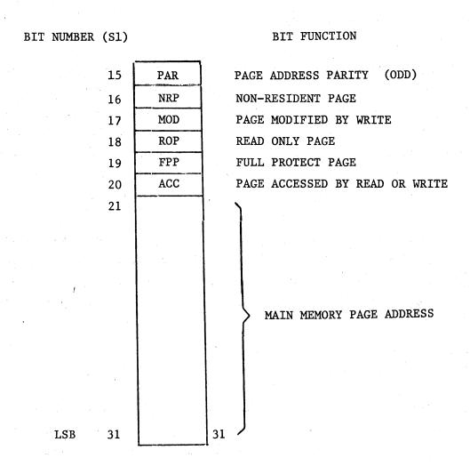
Figure 5-2. Page Index File Entry Bit Assignments
