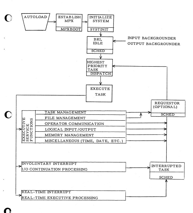
FIGURE 3-1. MPX System Flow
