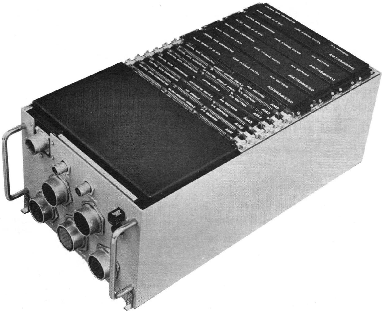
The CONTROL DATA Advanced Microprogrammable Processor (AMPP) provides a versatile solution to advanced processor requirements of the mid-1970's and beyond. The AMPP combines microprogrammed control with state-of-the-art circuit construction and a 750-nanosecond core memory in a MIL-E-5400 Processor, capable of executing more than 1,000,000 instructions per second.
