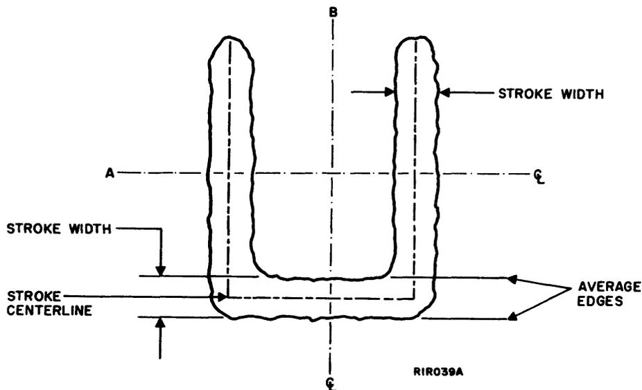
Figure 5-2. Stroke Width
