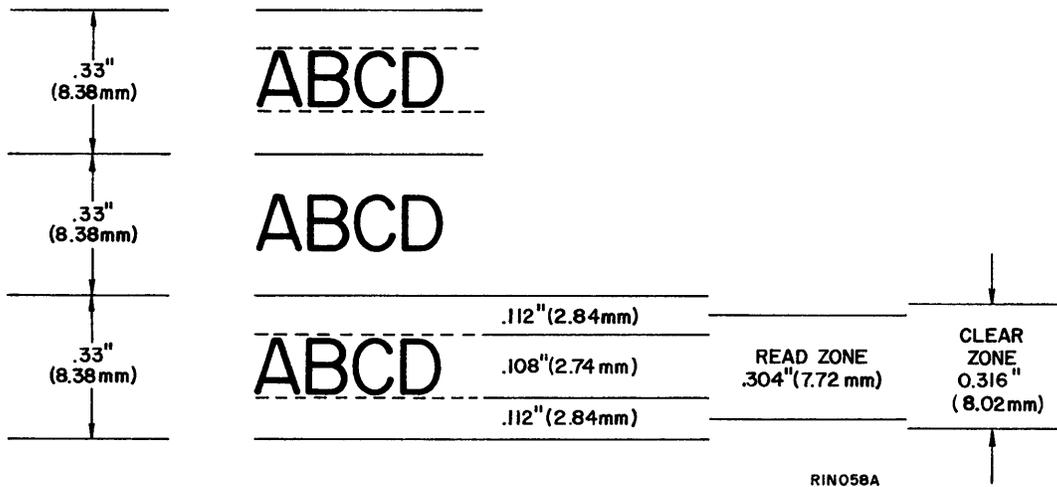
Figure 5-9. Scan 3. Maximum Line Density {Three Lines per Inch}
