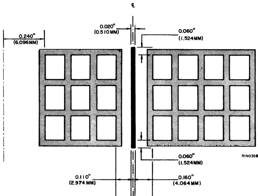
Figure 3-9. Multiple Line Handprint and Spacing Requirements
