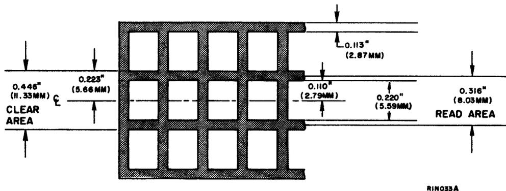
Figure 3-14. Vertical Clear Area for Multiple Lines
