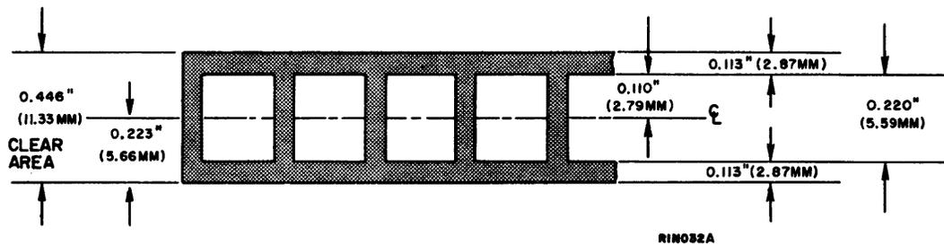
Figure 3-13. Vertical Clear Area for Single Line
