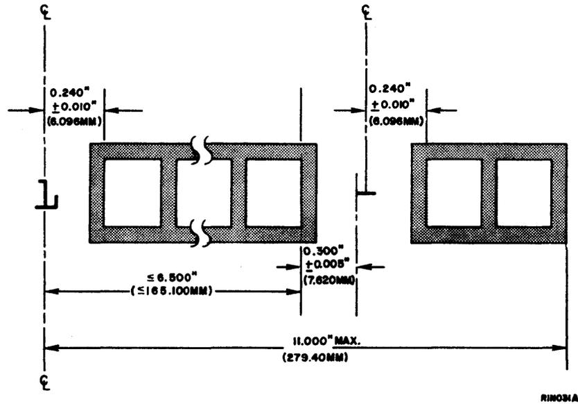
Figure 3-7. Reference Character Positioning for Line Longer than 6.5 Inches {165.1 mm}
