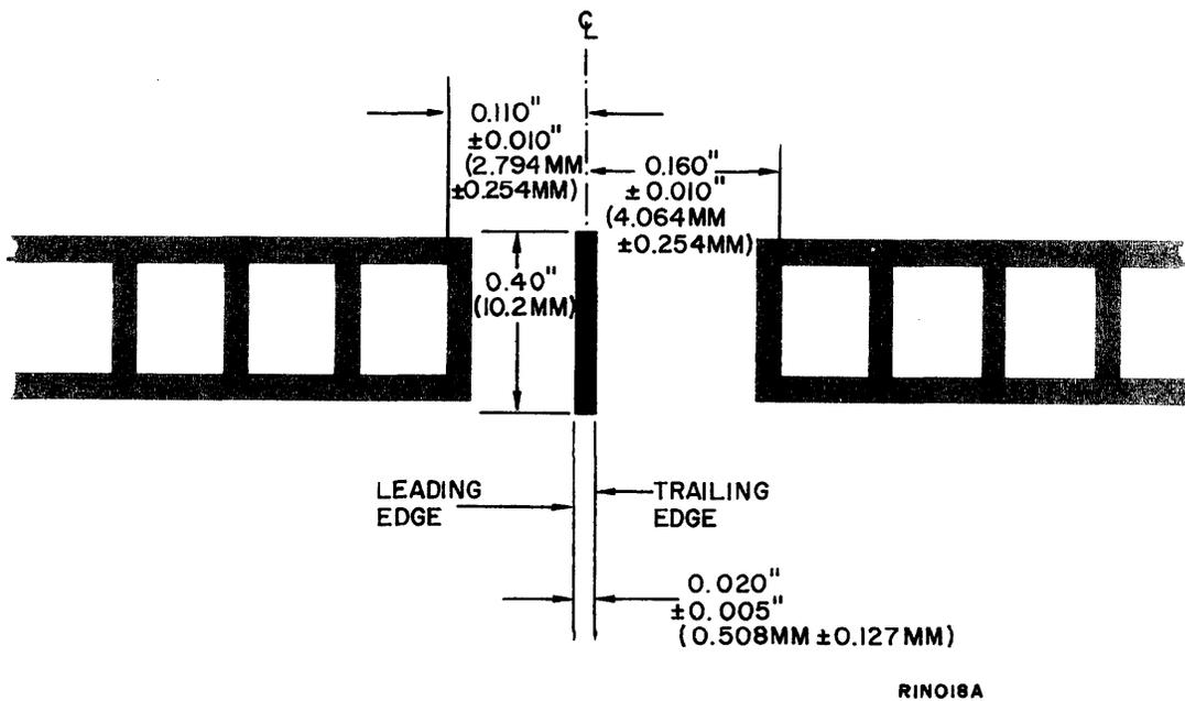
Figure 3-8. Field Mark Dimensions {for Vertical Line Spacing Densities of Two Lines per Inch or Less}
