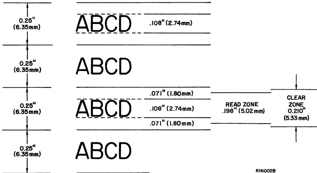
Figure 5-8. Scan 2. Maximum Line Density {Four Lines per Inch}
