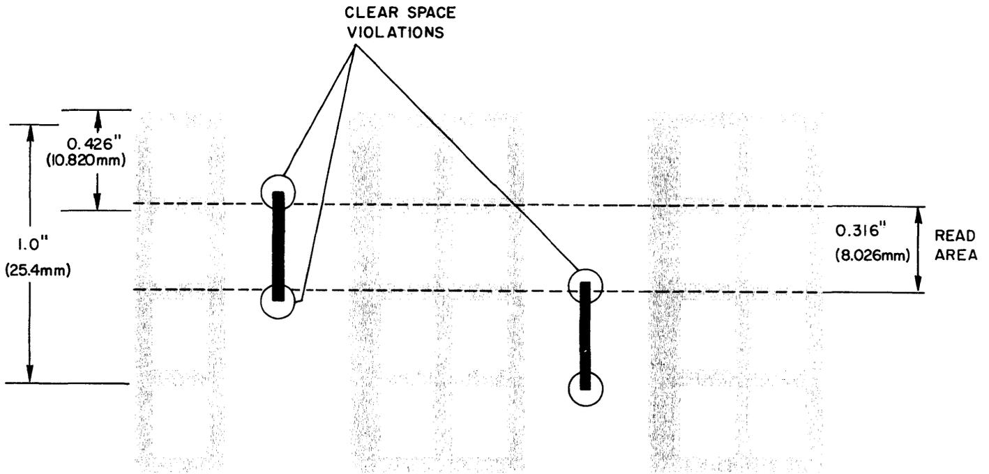
**A. IMPROPER PLACEMENT OF FIELD MARKS**
