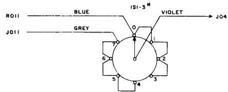
\* ON SWITCH SECTIONS 1, 2, AND 3, NUMBERING REFERS TO SWITCH POSITION, NOT PIN NUMBERS.
