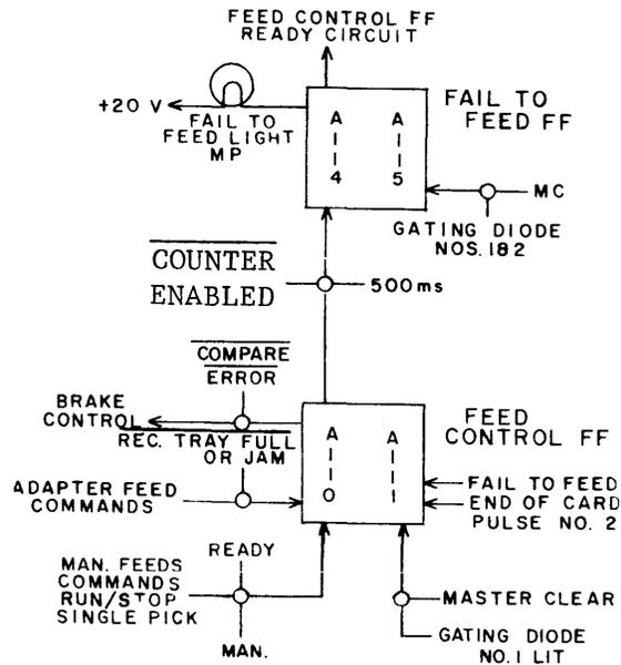
Figure 12 Feed Control Circuit
