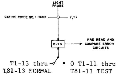
Figure 7 Compare Pulse Timing Circuit
