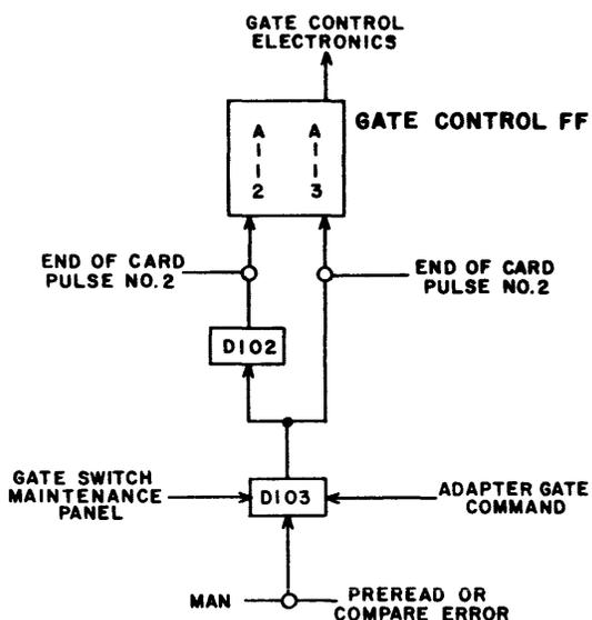
Figure 13 Gate Control Circuit
