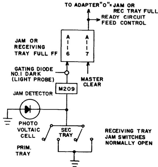
Figure 15 Jam or Receiving Tray Full Circuit
