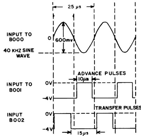
Figure 4 CLOCK ADVANCE AND TRANSFER PULSES
