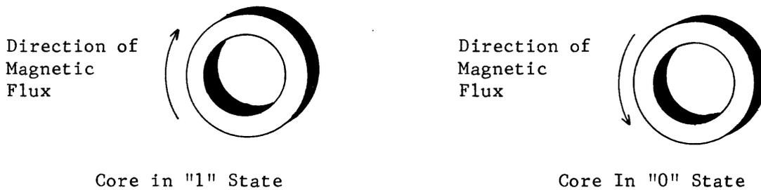
Figure 8-18. Magnetized Cores
