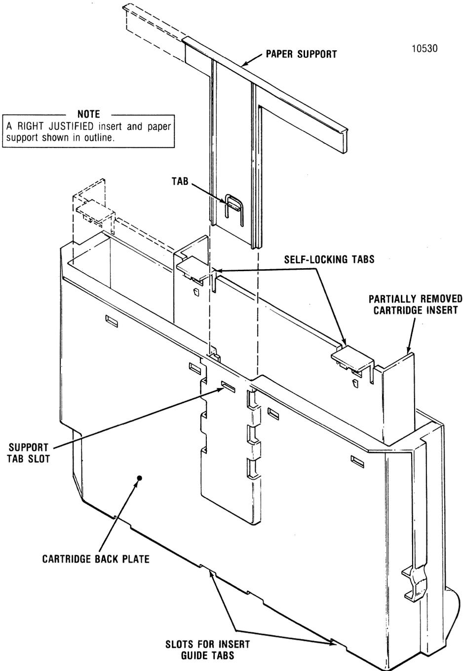
**Figure 4-5 Removal/Replacement, Cartridge Insert (Fixed-Width Cartridge Shown: Insert and Support Justified Left)**
