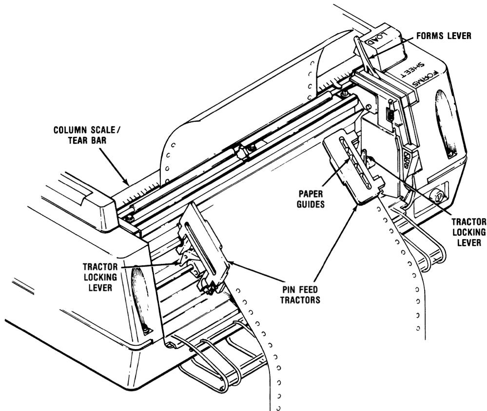
Figure 3-1 Preliminary Adjustments
