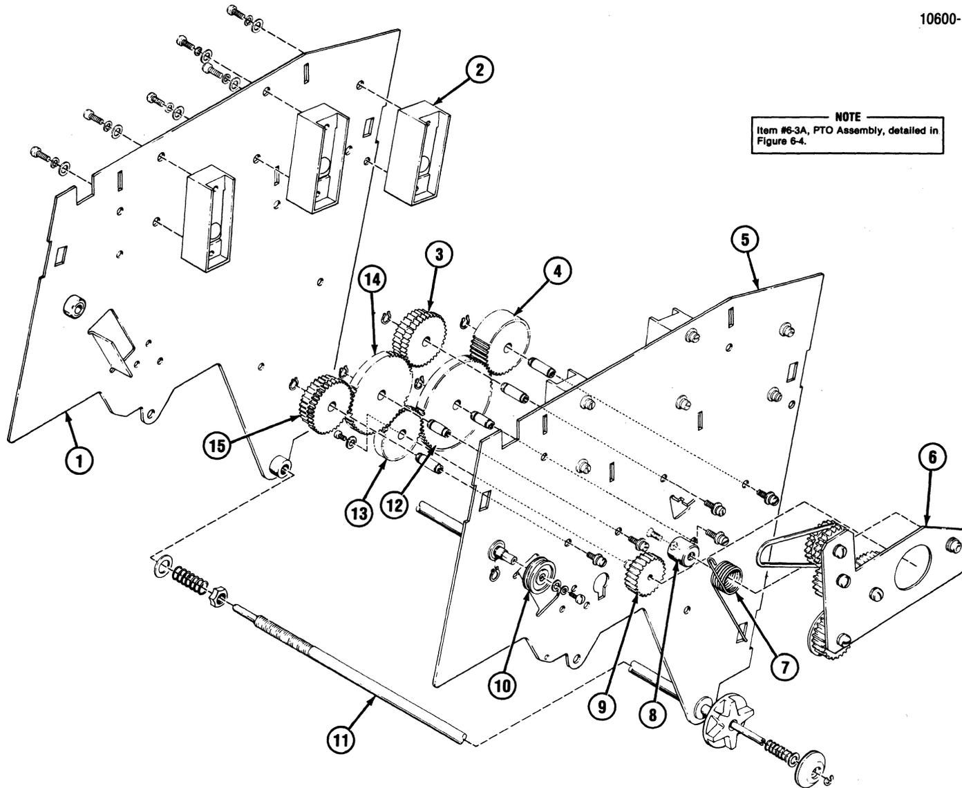
Figure 6-3A Sheet Feeder, Mechanism
