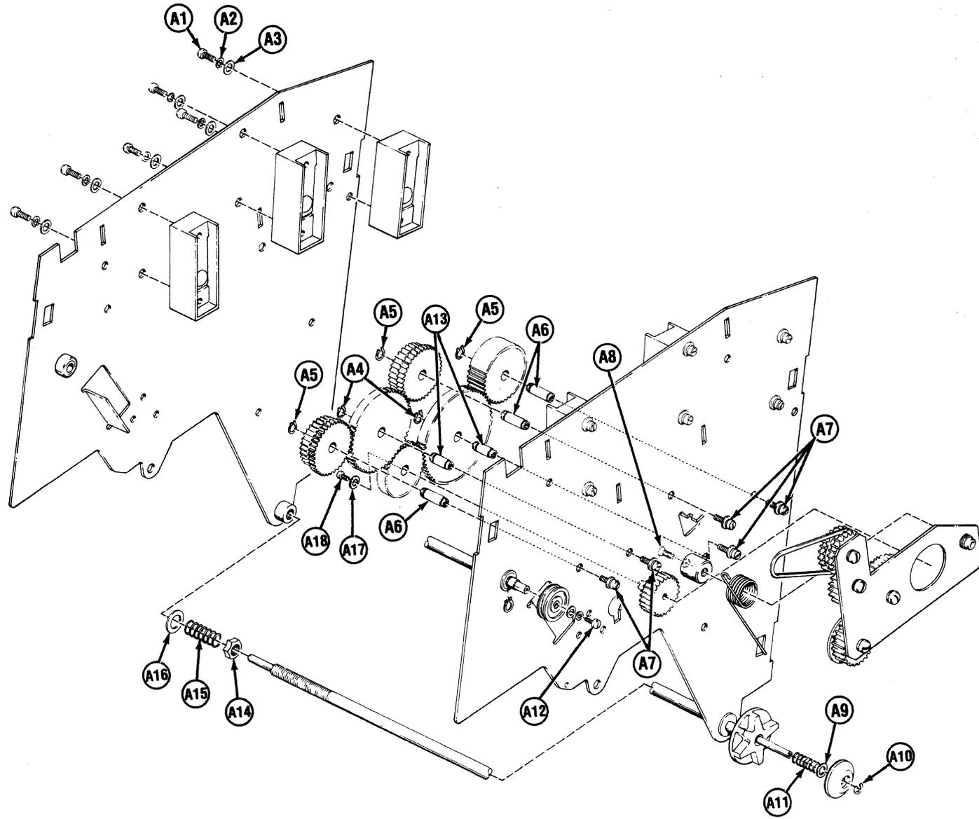
Figure 6-3B Sheet Feeder, Mechanism
