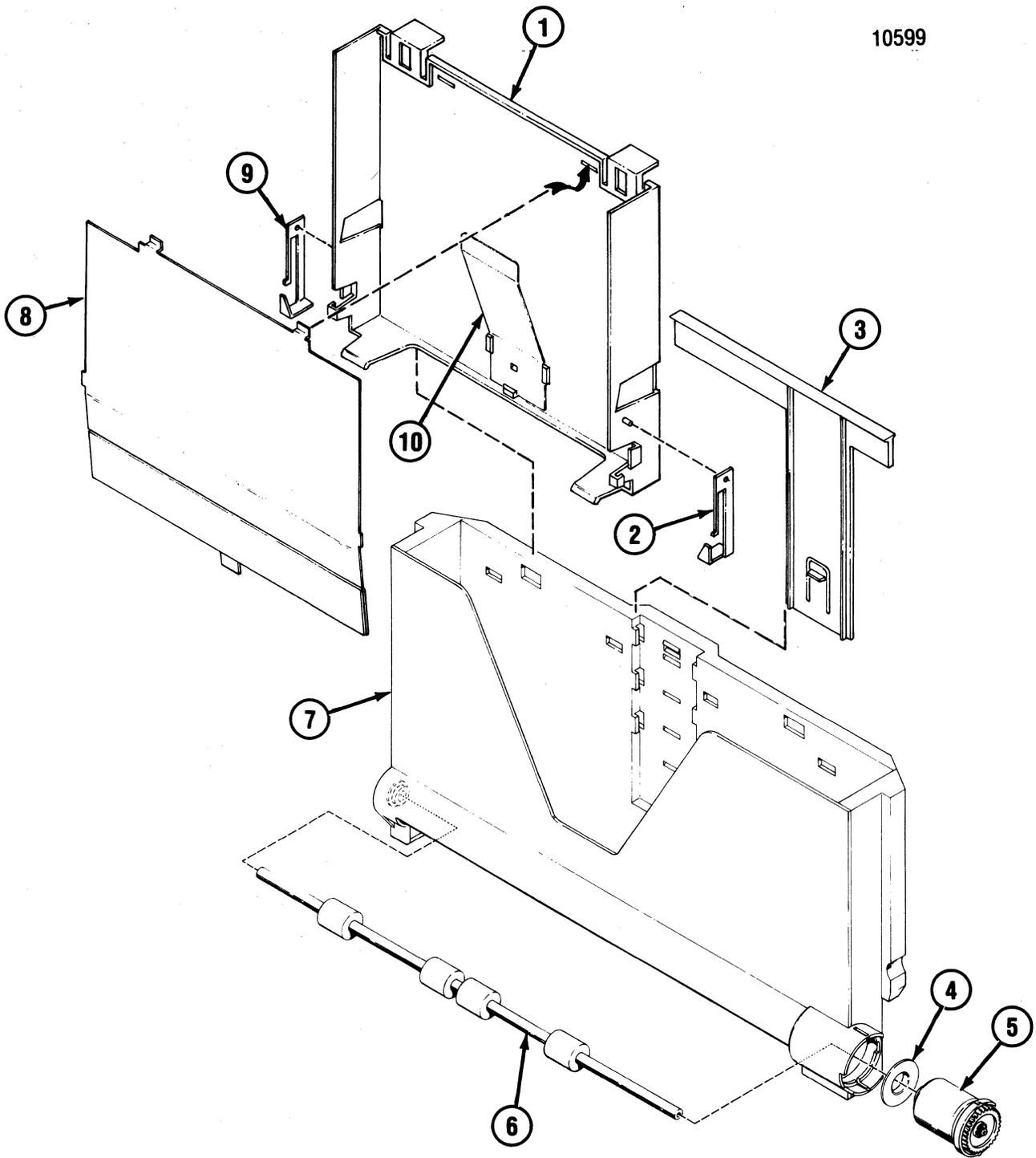
**Figure 6-5 Fixed-Width Paper Cartridge (Figure valid for both the 8.5" cartridge and the 21 cm cartridge)**
