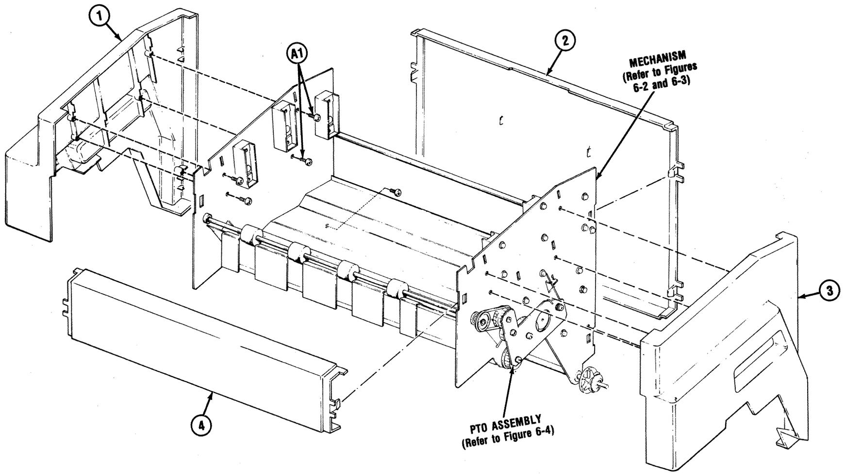
Figure 6-1 Sheet Feeder Cover Panels
