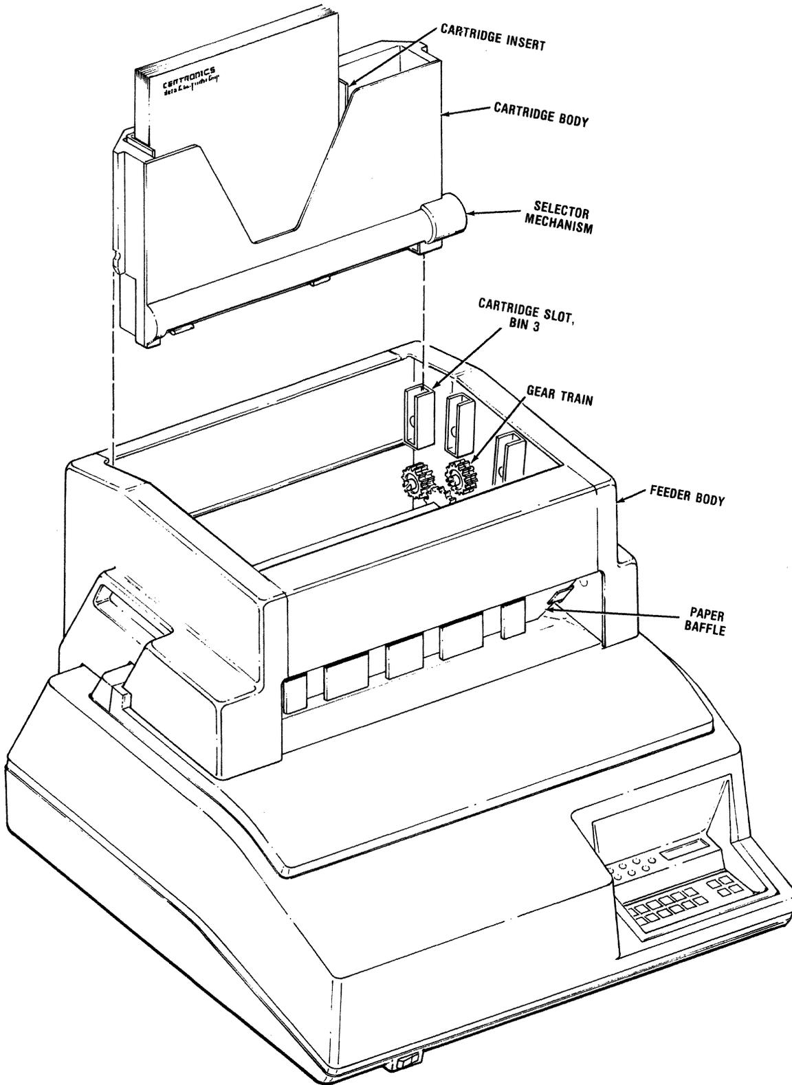
Figure 2-1 Feeder Components
