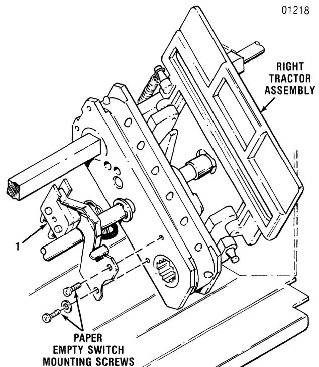
**Figure 5-18 Removal/Replacement,
