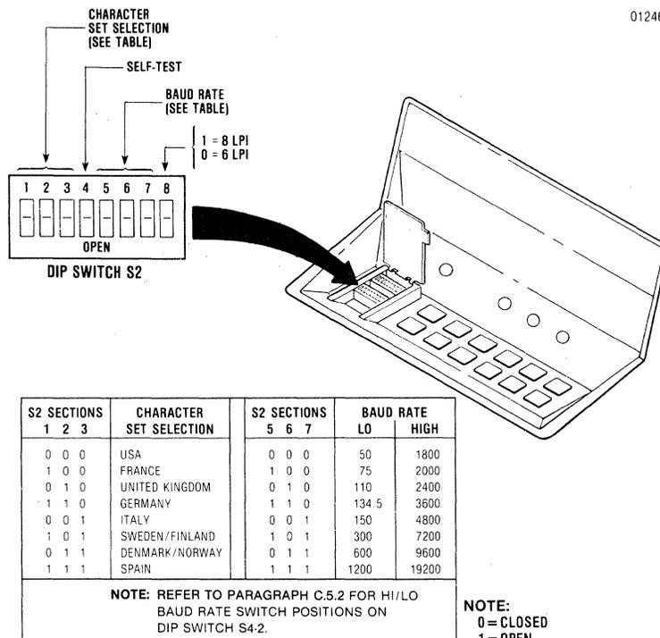
**Figure C-5 Printer Features Dip Switch S2**
