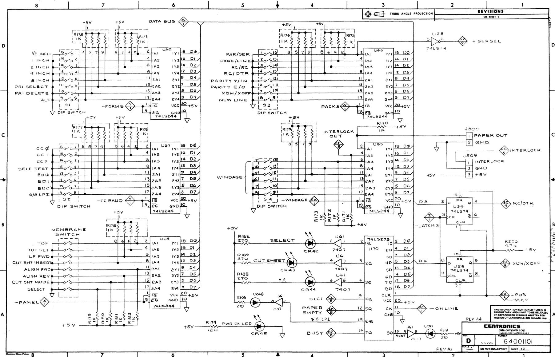
Figure A-1 Schematic Diagram, Formatter/Controller, 64001101-9001 (Sheet 10 of 11).
