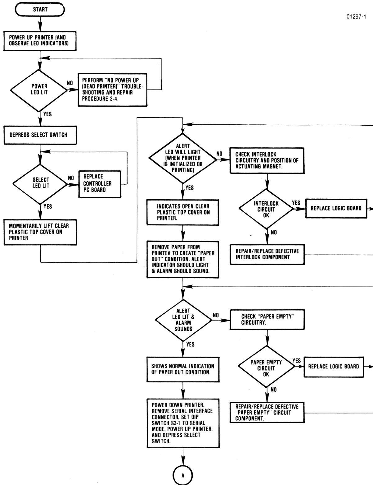
Figure 3-6 Control Panel Switches and Indicators Troubleshooting Flow Chart (Sheet 1 of 3)
