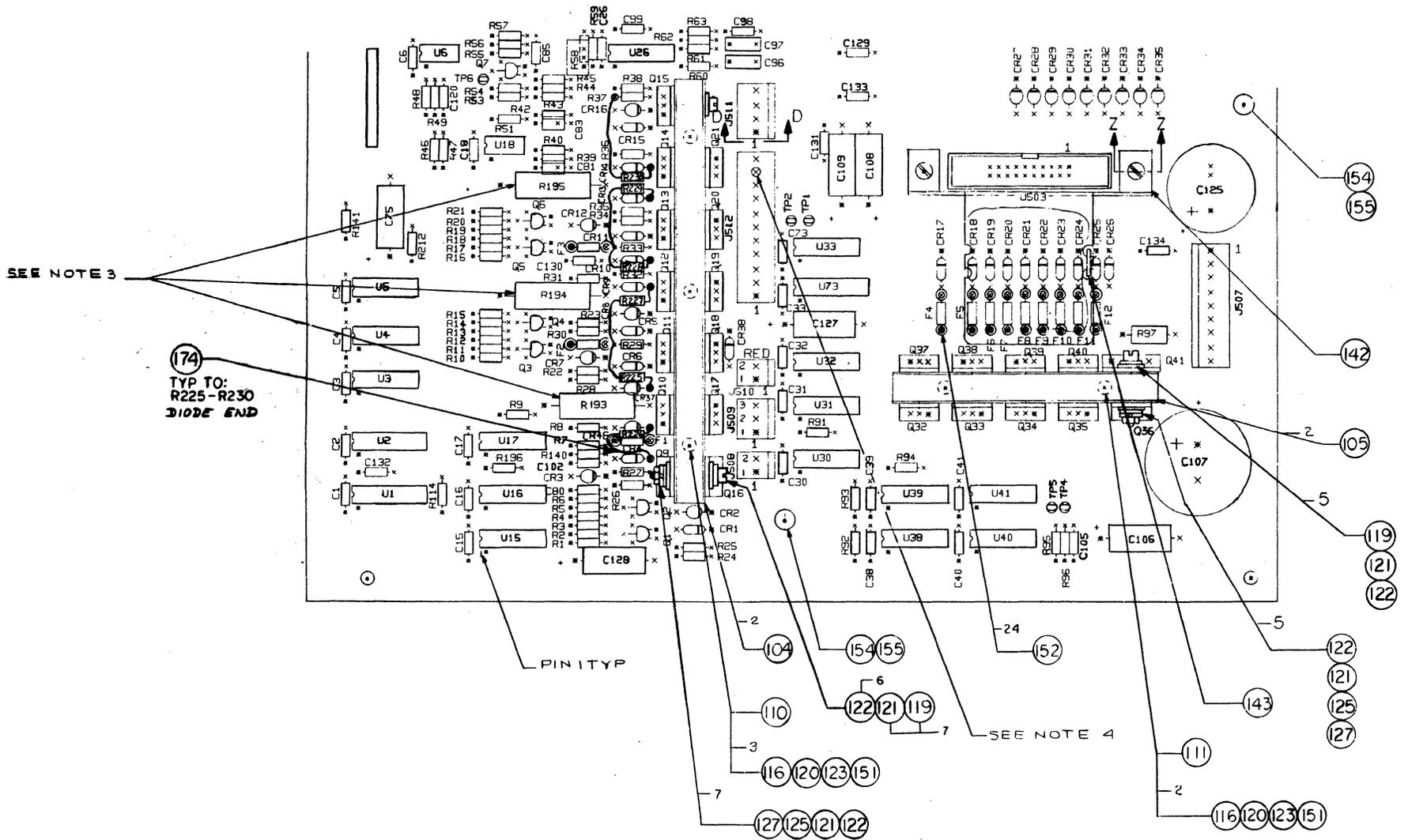
Figure A-6 Assembly Drawing, Print Head Driver and D.C. Power Entry Section, Formatter/Controller PCB Assembly
