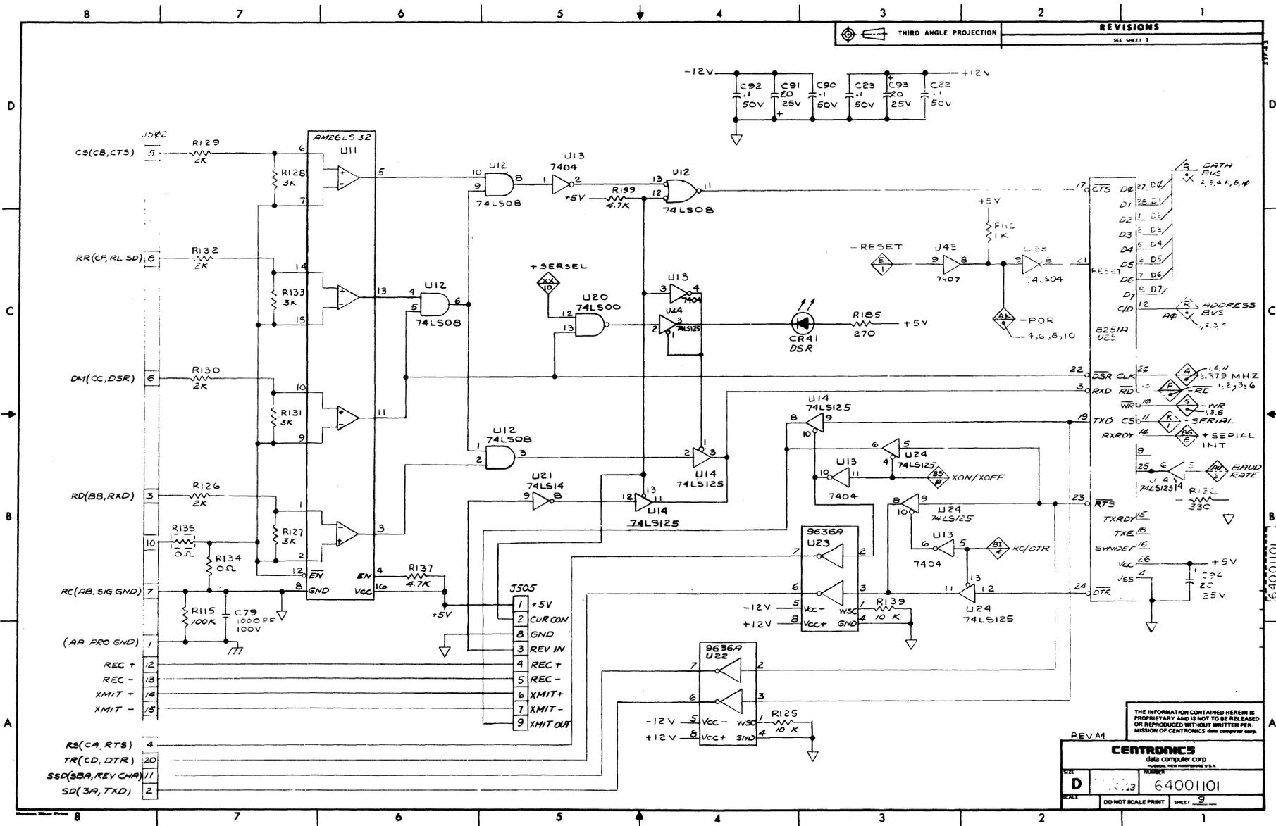
Figure A-1 Schematic Diagram, Formatter/Controller, 64001101-9001 (Sheet 9 of 11).
