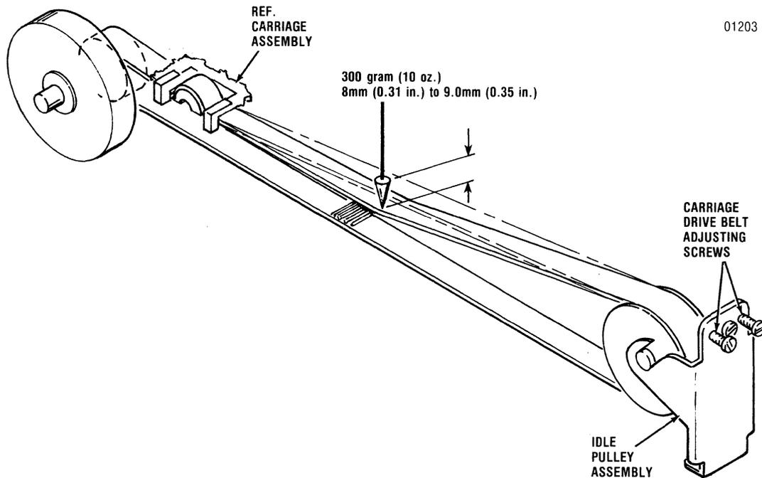
Figure 4-1 Carriage Drive Belt Adjustment
