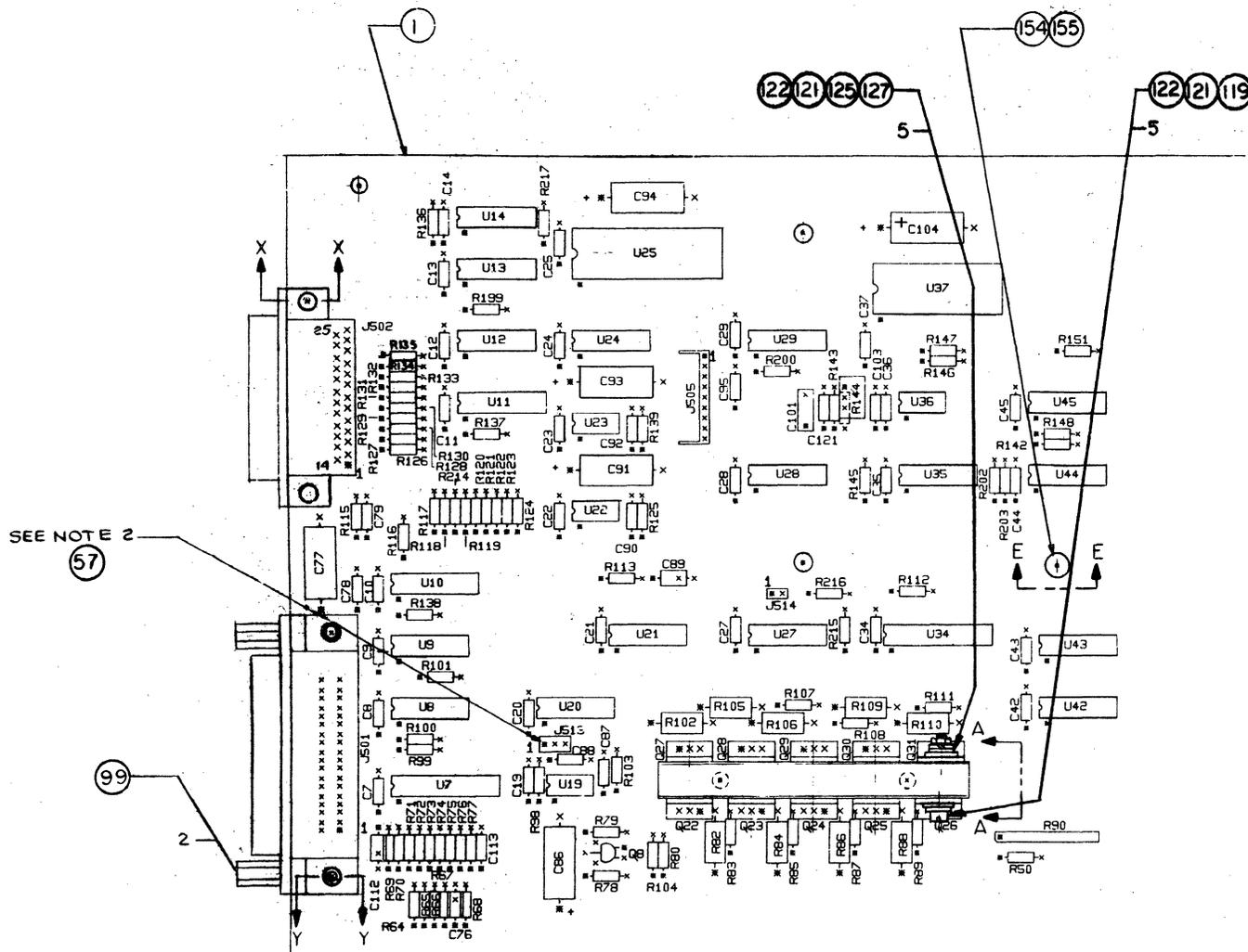
Figure A-5 Assembly Drawing, Serial and Parallel Input Section, Formatter/Controller PCB Assembly
