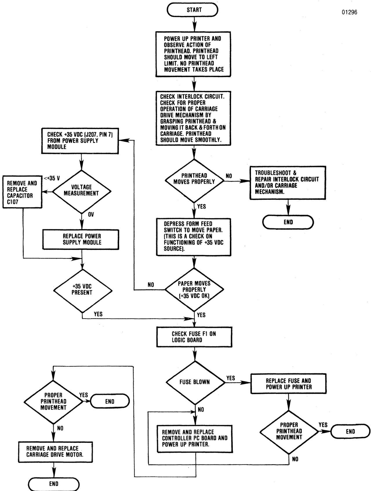
Figure 3-5 No Print Head Movement on Power-Up Troubleshooting Flow Chart
