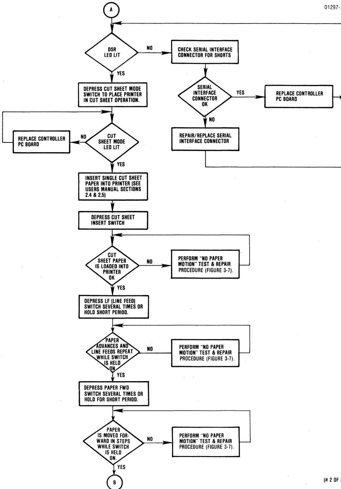
Figure 3-6 Control Panel Switches and Indicators Troubleshooting Flow Chart (Sheet 2 of 3)
