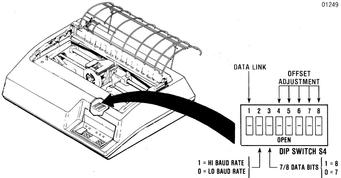
Figure C-7 Printer Features Dip Switch S4
