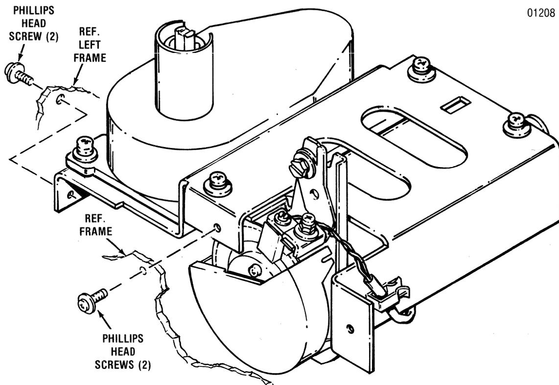
Figure 5-13 Removal/Replacement, Ribbon Drive Motor Mounting Bracket
