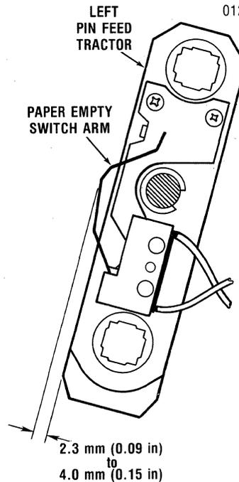
Figure 4-5 Paper Empty Switch Adjustment
