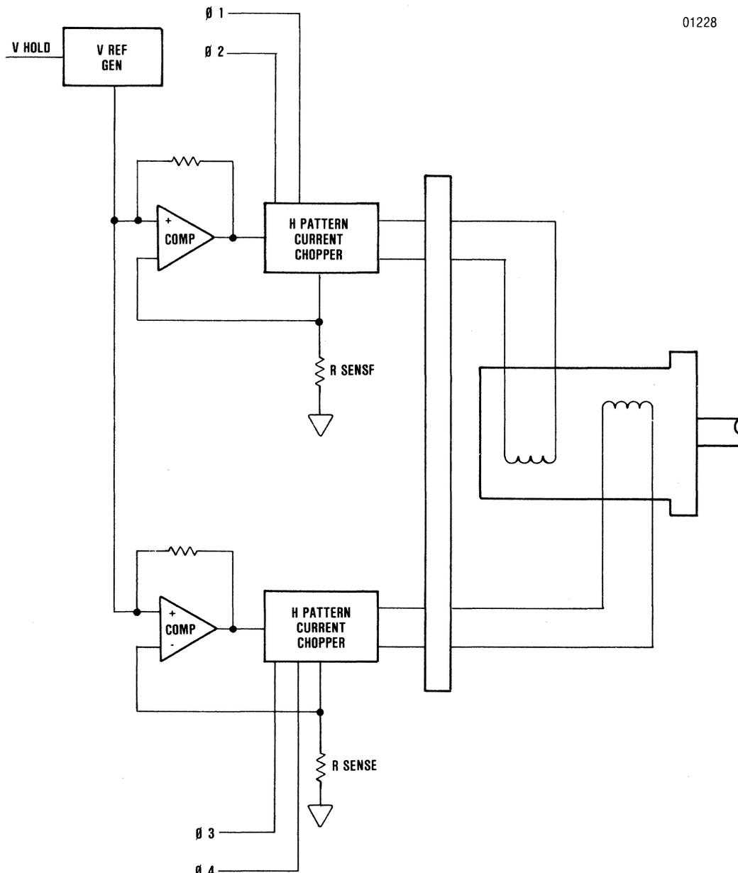
**Figure 2-5 Paper Feed Stepper Motor Driver**
