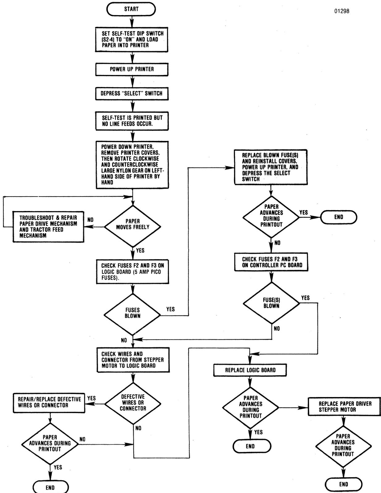
Figure 3-7 Printout, No Paper Motion (No Line Feeds) Troubleshooting Flow Chart
