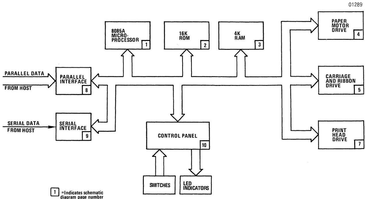
**Figure 2-1 Model 351 Basic Functional Block Diagram**
