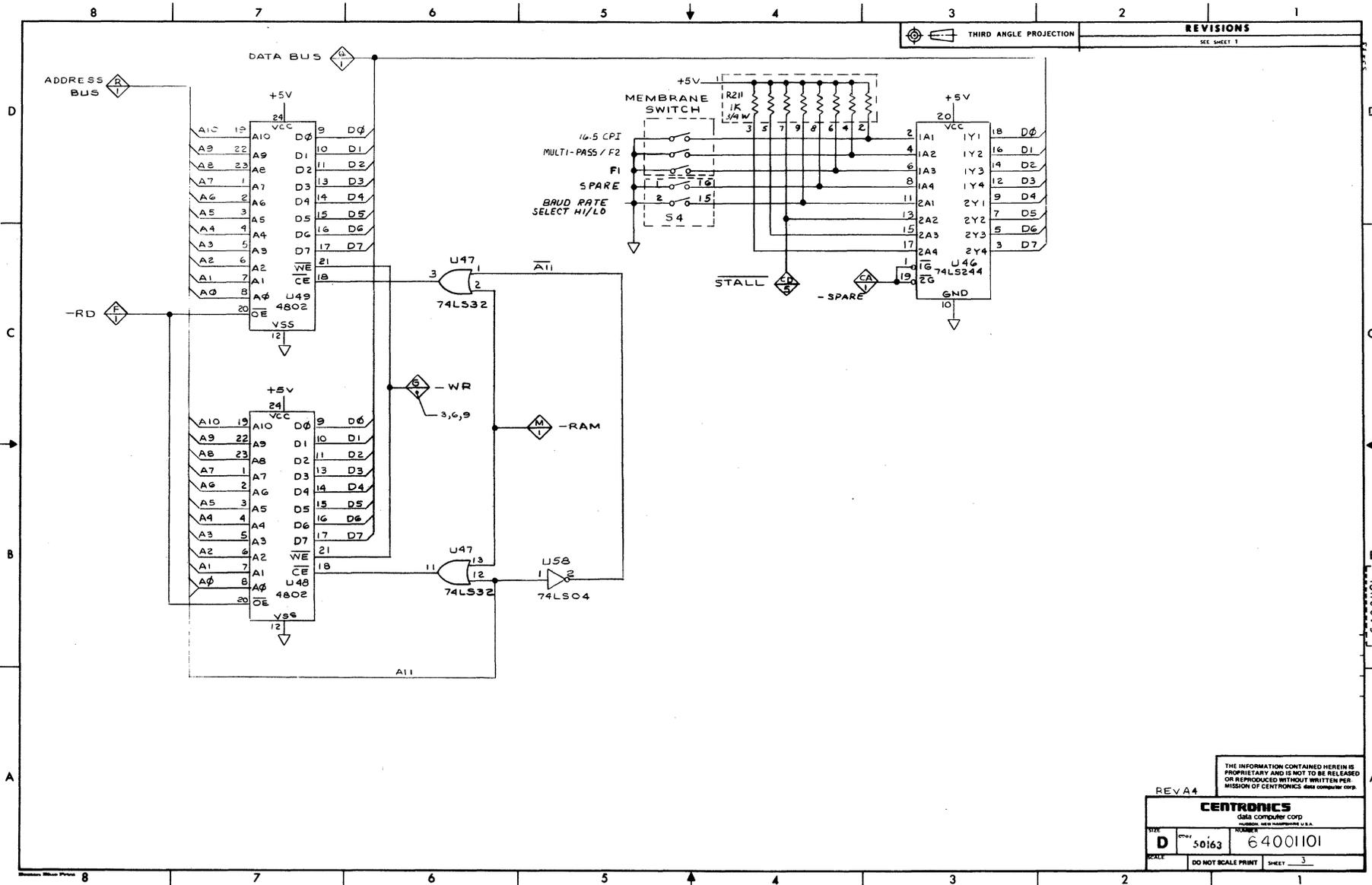
Figure A-1 Schematic Diagram, Formatter/Controller, 64001101-9001 (Sheet 3 of 11).
