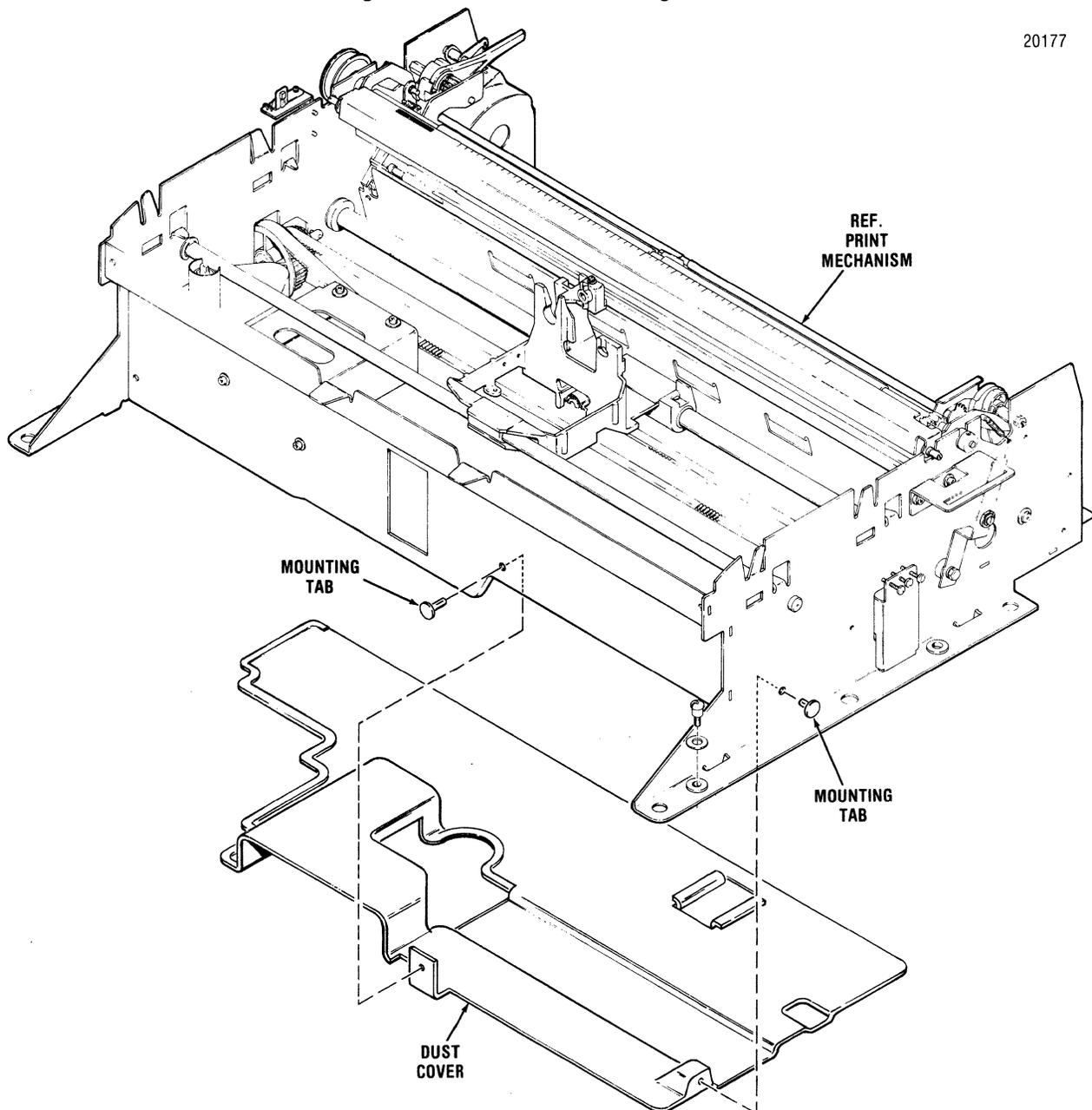
Figure 5-8 Removal/Replacement, Dust Cover
