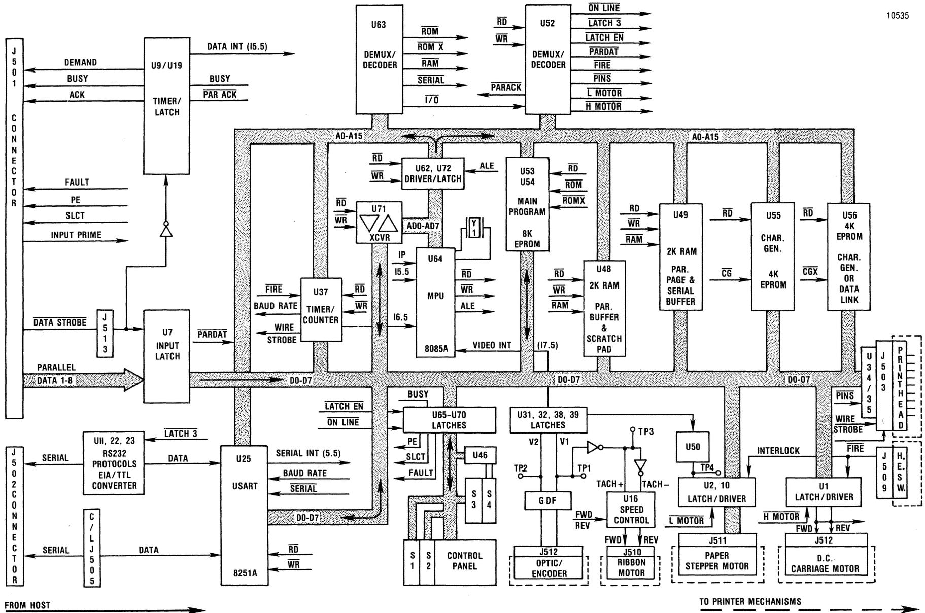
Figure 2-2 Model 351 Formatter/Controller Board
