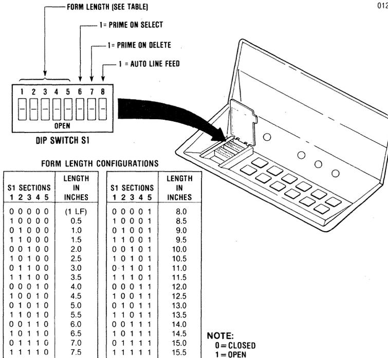
**Figure C-4 Printer Features Dip Switch S1**
