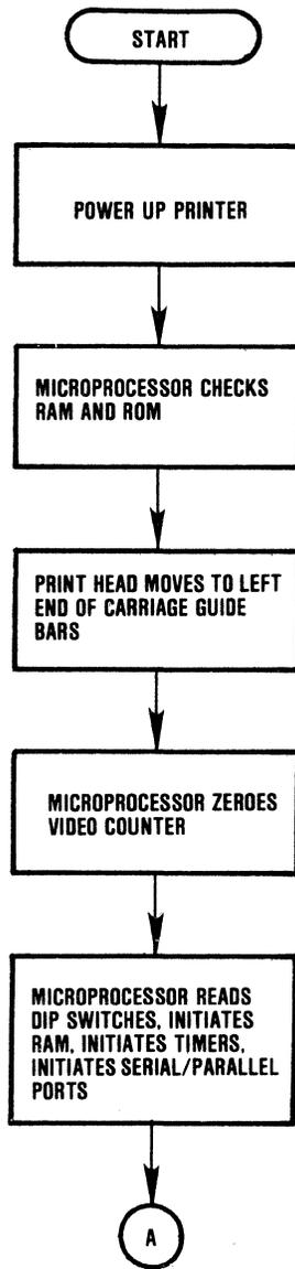
Figure 3-2 Self-Test on Power-up Flow Chart (Sheet 1 of 3)
