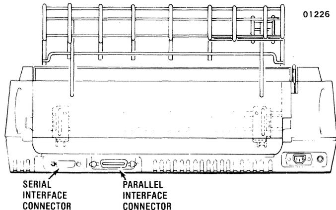
Figure B-2 Parallel and Serial Interface Connectors
