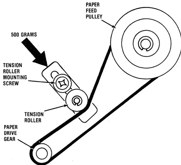
Figure 4-4 Paper Drive Belt Adjustment
