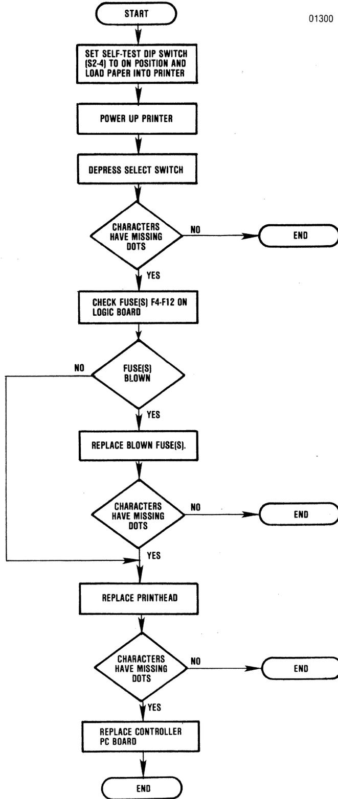
Figure 3-9 Broken Characters (Missing Dots) Troubleshooting Flow Chart
