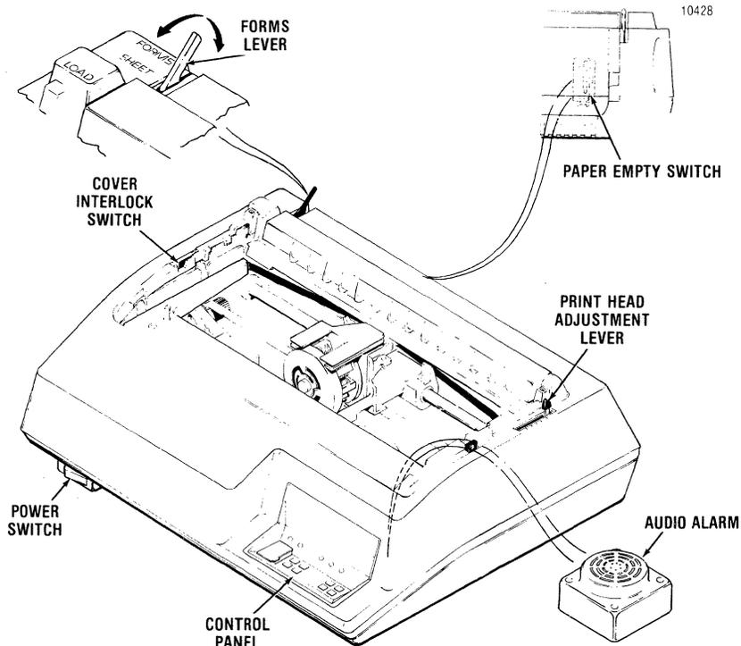
Figure C-1 Printer Mechanism Controls and Switches
