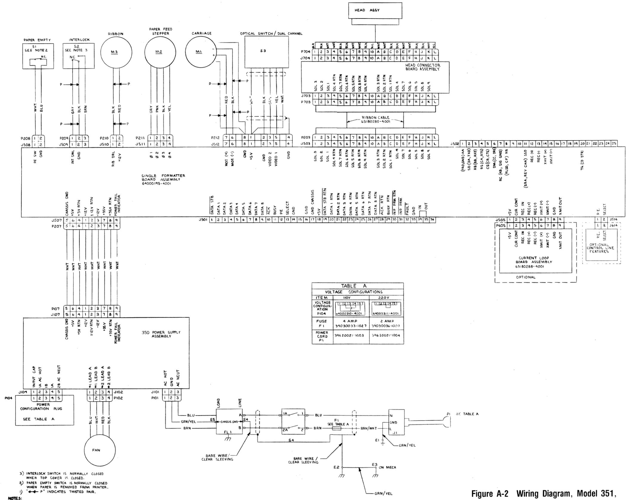
Figure A-2 Wiring Diagram, Model 351, 64000504-9001.
