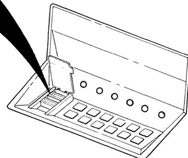
Figure C-3 Control Panel Dip Switches
