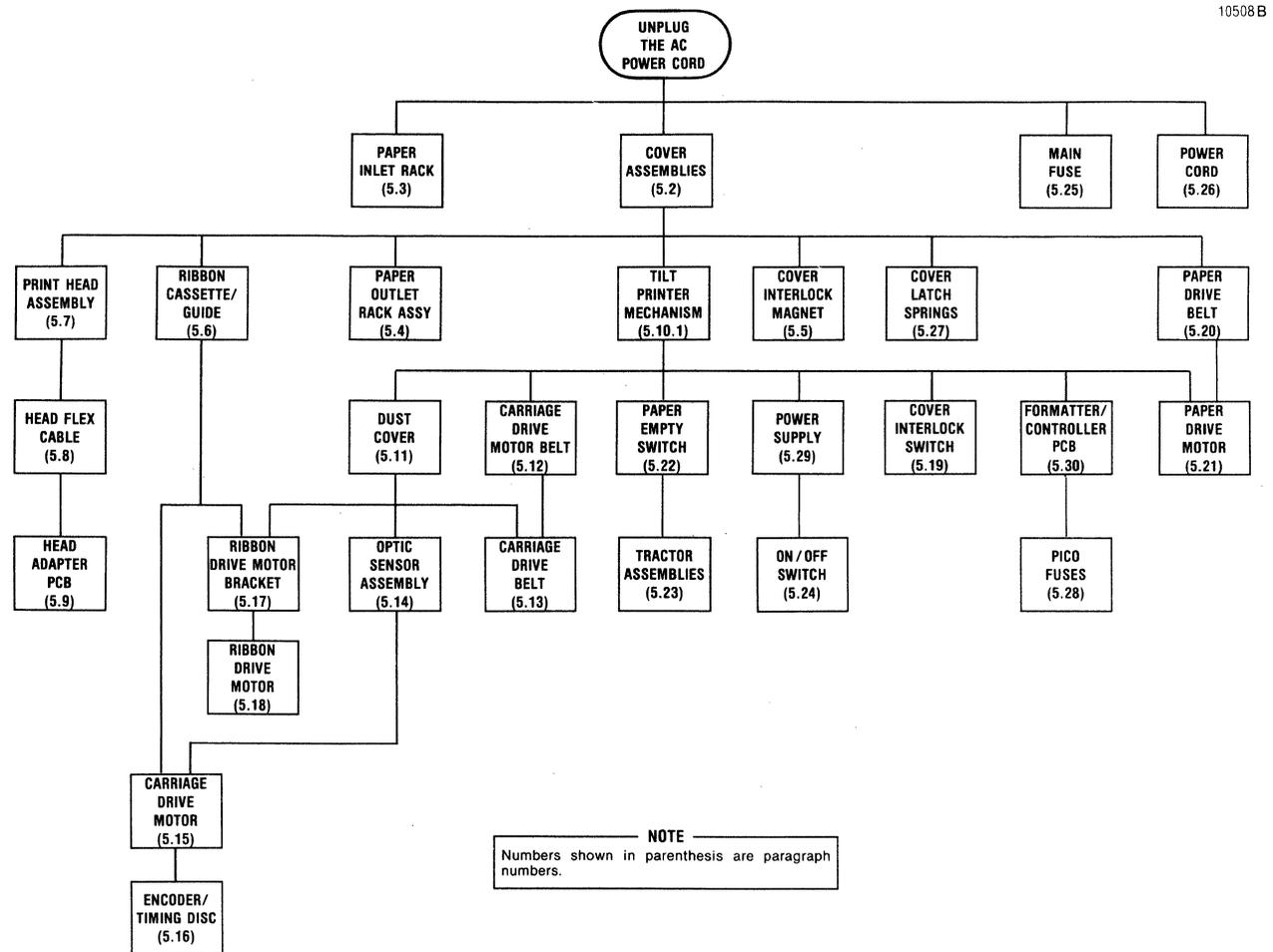
Figure 5-1 Removal/Replacement Procedure Diagram
