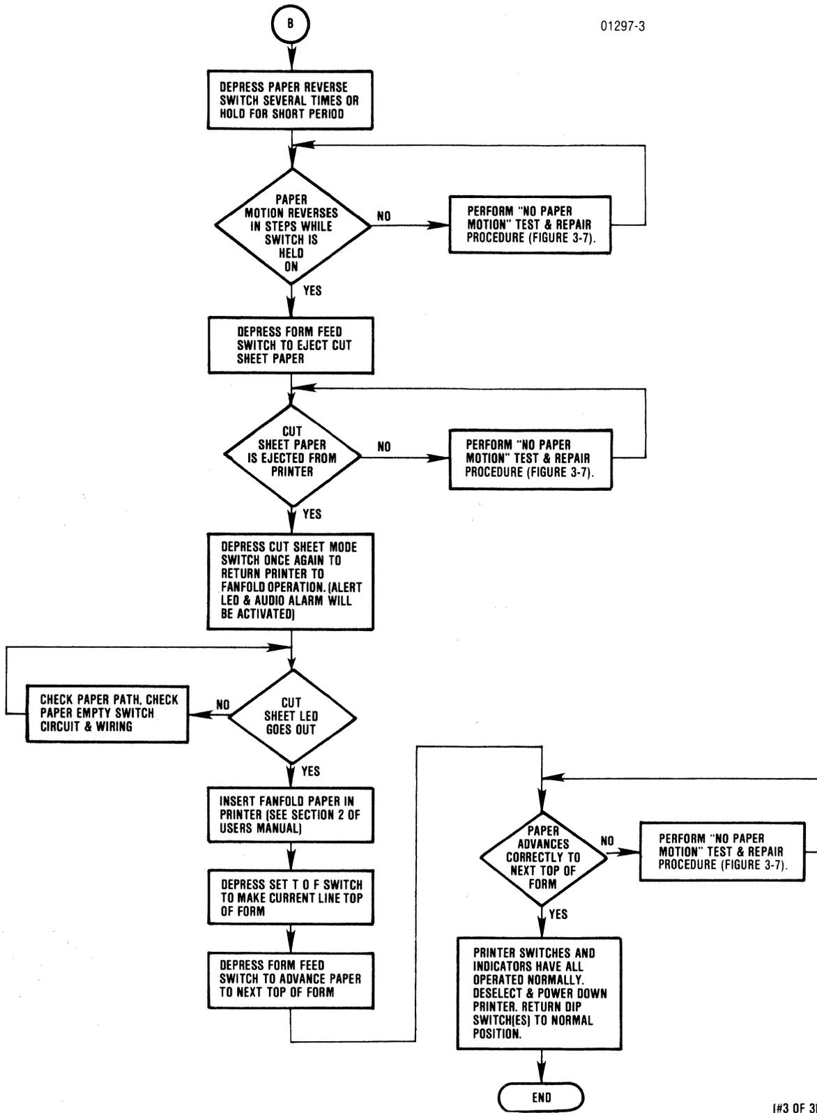
Figure 3-6 Control Panel Switches and Indicators Troubleshooting Flow Chart (Sheet 3 of 3)
