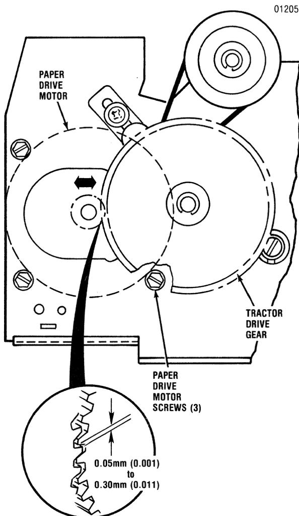
**Figure 4-3 Tractor Gear Backlash Adjustment**
