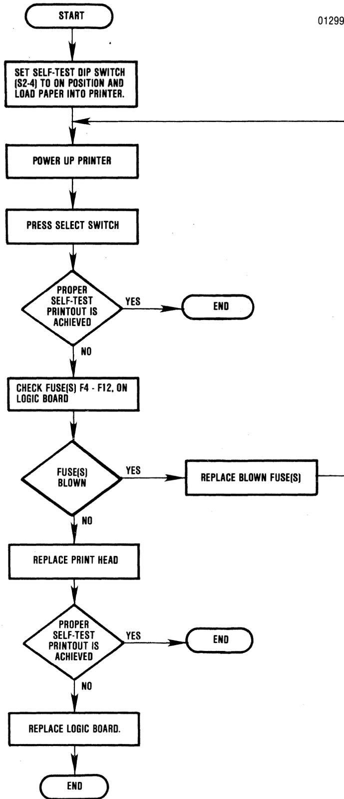
Figure 3-8 Print Head Movement, Paper Movement, No Printout Troubleshooting Flow Chart
