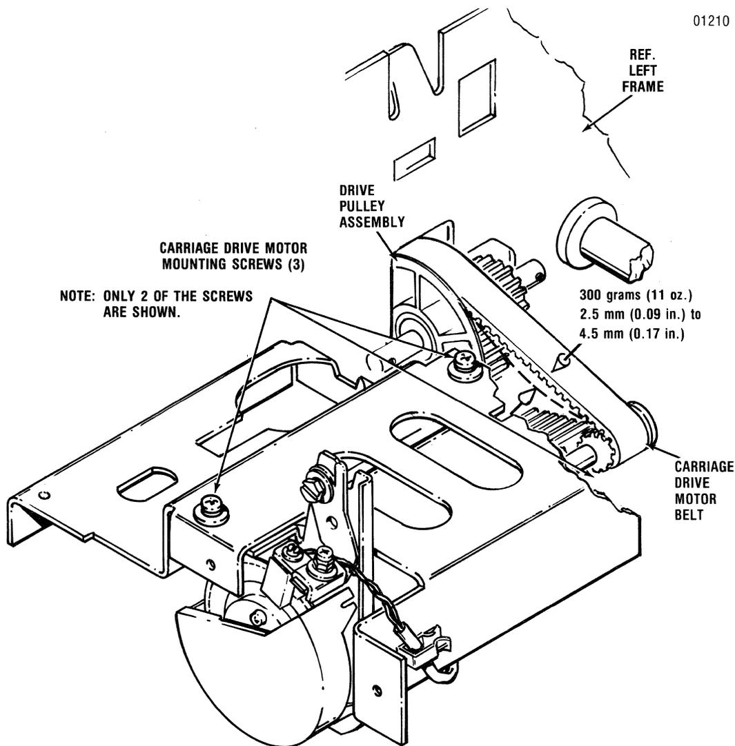
Figure 4-2 Carriage Drive Motor Belt Adjustment
