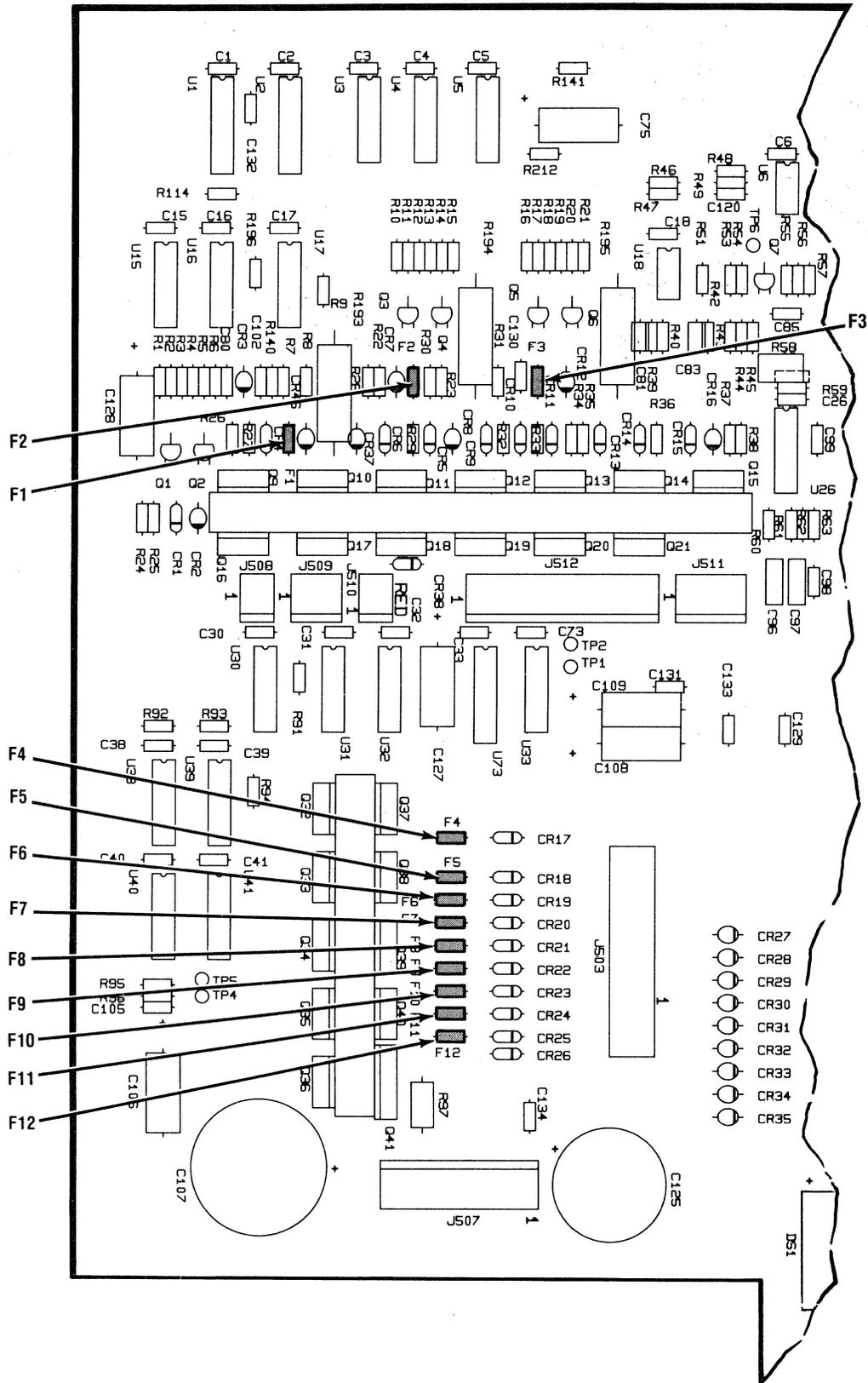
Figure 5-23 Removal/Replacement, Pico Fuses
