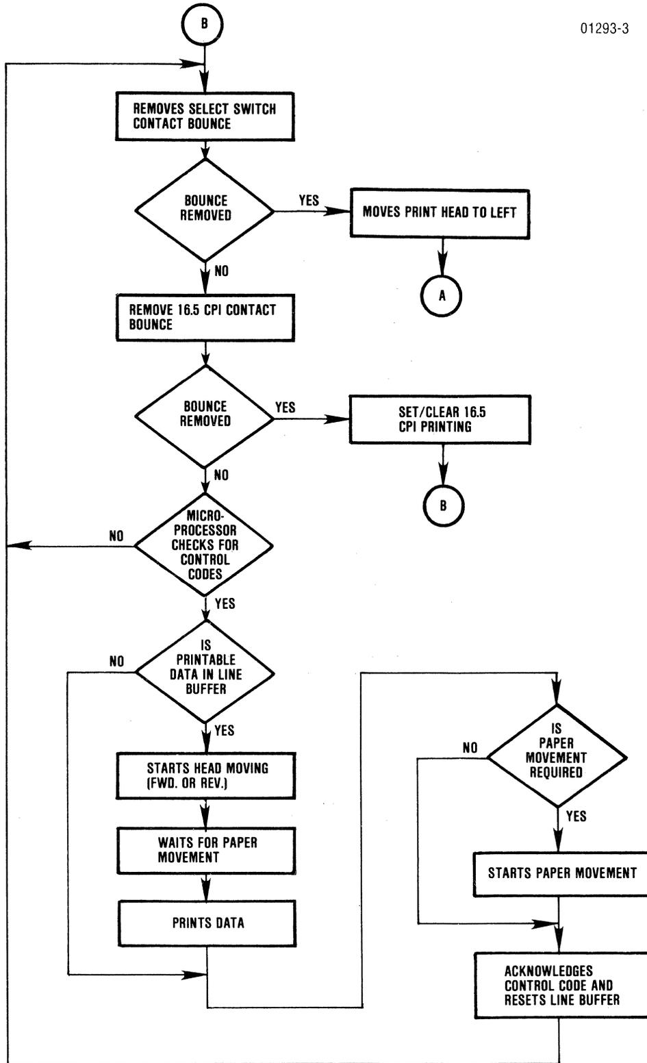
Figure 3-2 Self-Test on Power-up Flow Chart (Sheet 3 of 3)
