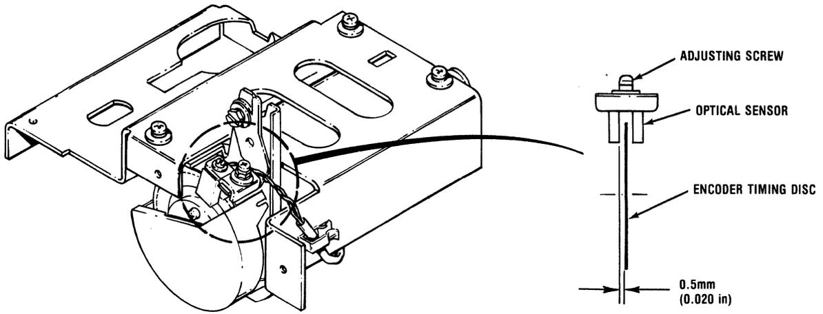
Figure 4-6 Mechanical Adjustment, Optical Sensor and Encoder/Timing Disc
