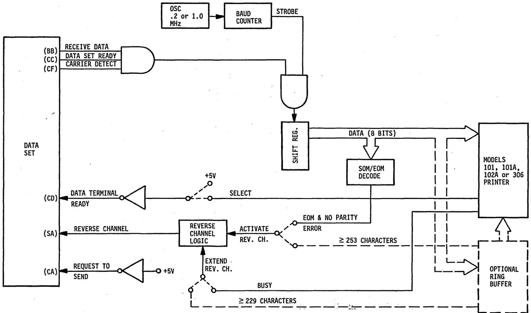
Figure 1. RS232 Interface Data Flow Diagram
