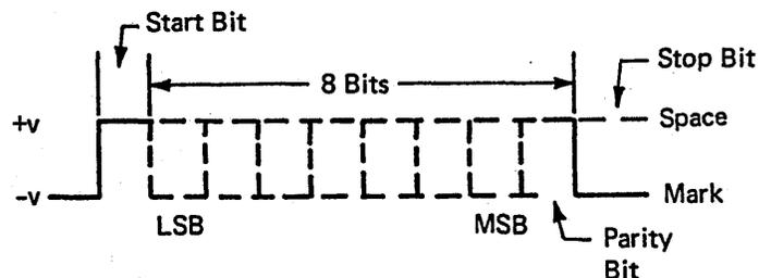
Figure 3. Serial Input Data
