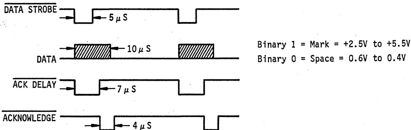
Figure 5. Parallel Output Data
