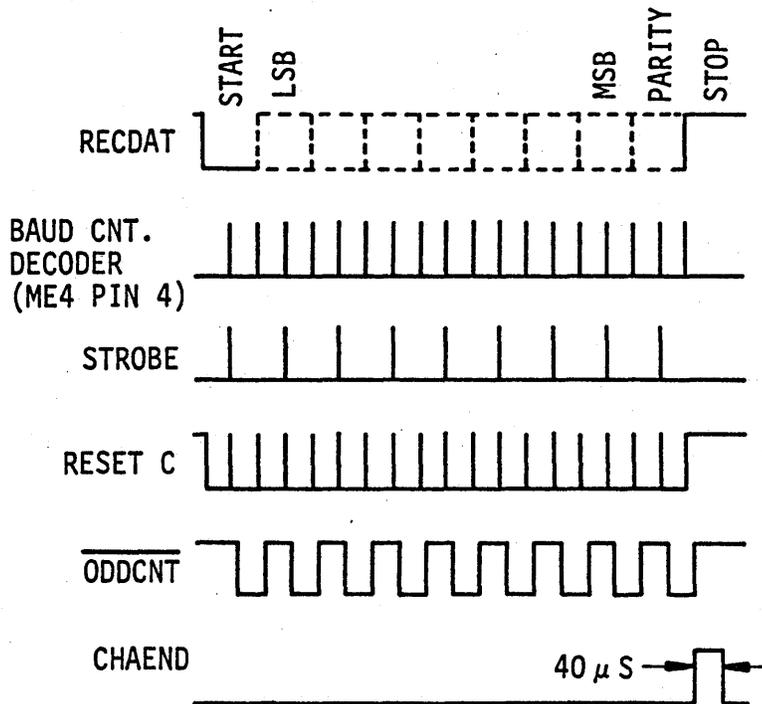
Figure 4. Serial Input Timing
