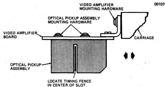
Figure 6-10 Optical Pickup/Timing Fence Alignment
