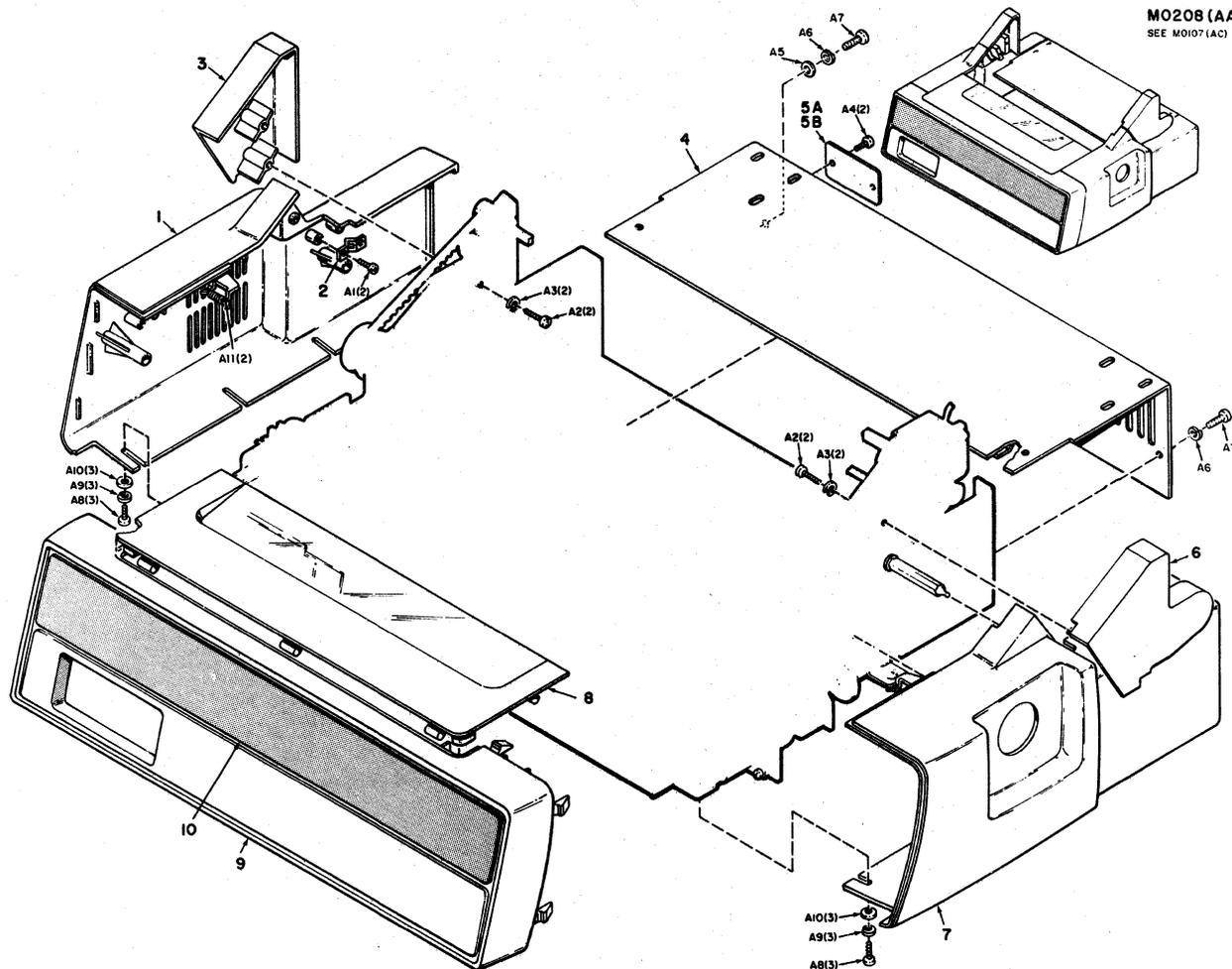
Figure 7-1 Removal/Replacement, Cover Assemblies
