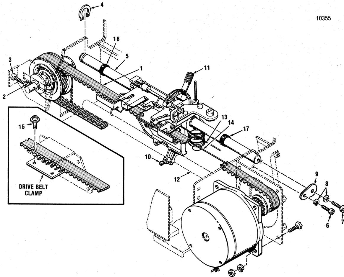
**Figure 7-7 Removal/Replacement, Carriage Assembly**
