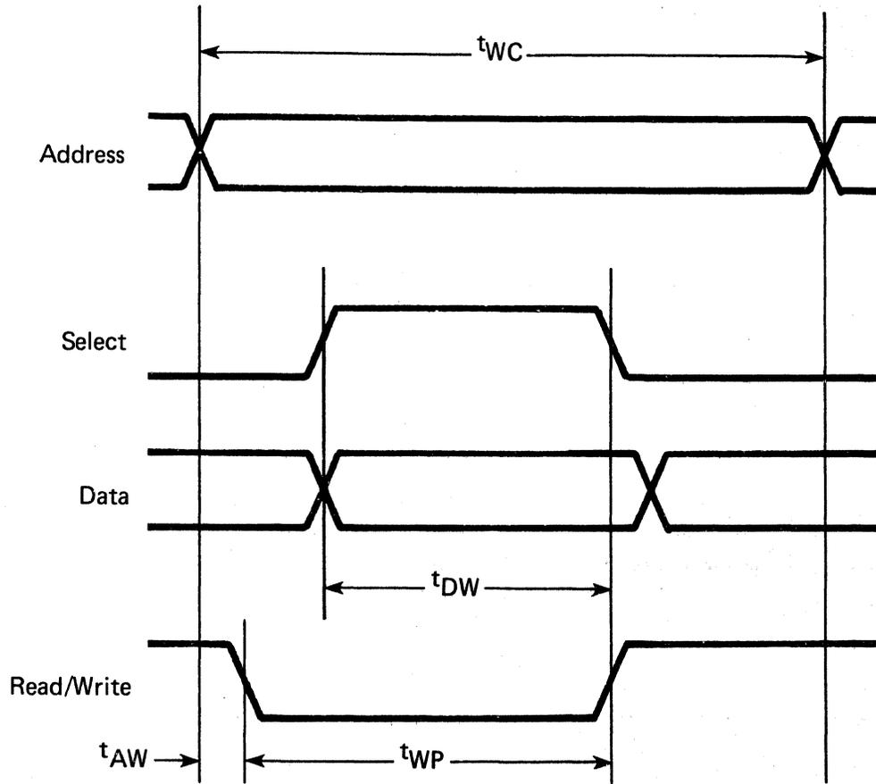
Rise and fall times shall be less than 30 nanoseconds.
