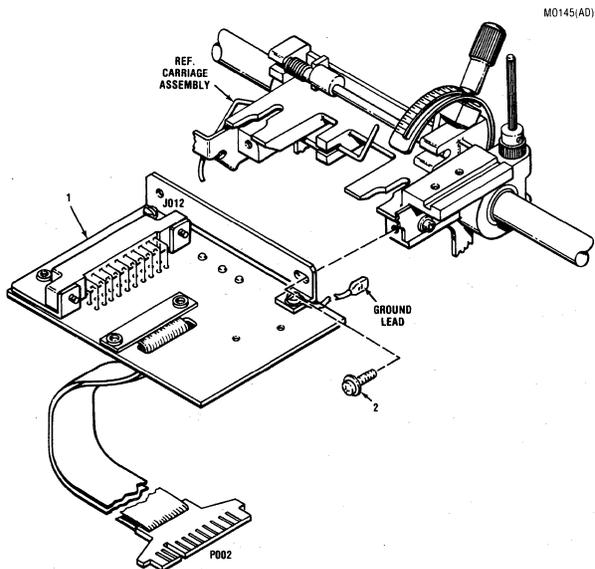
Figure 7-6 Removal/Replacement, Video Amplifier Assembly
