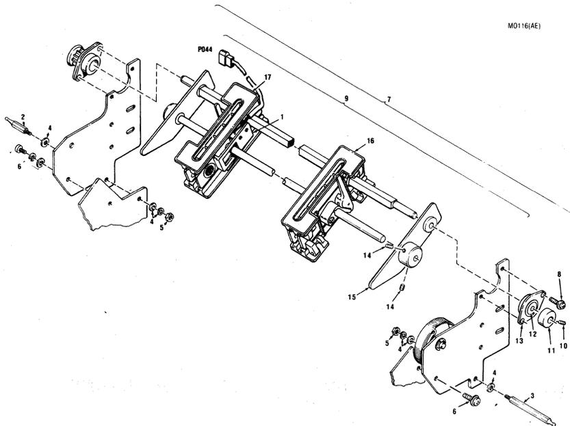
Figure 7-11 Removal/Replacement, Tractor Drive Assembly and Left/Right, Pin Feed Tractors
