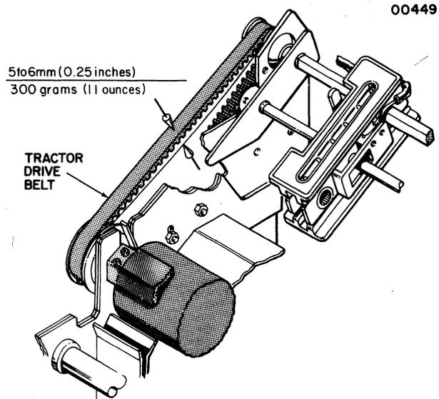
Figure 6-7 Tractor Drive Timing Belt Tension
