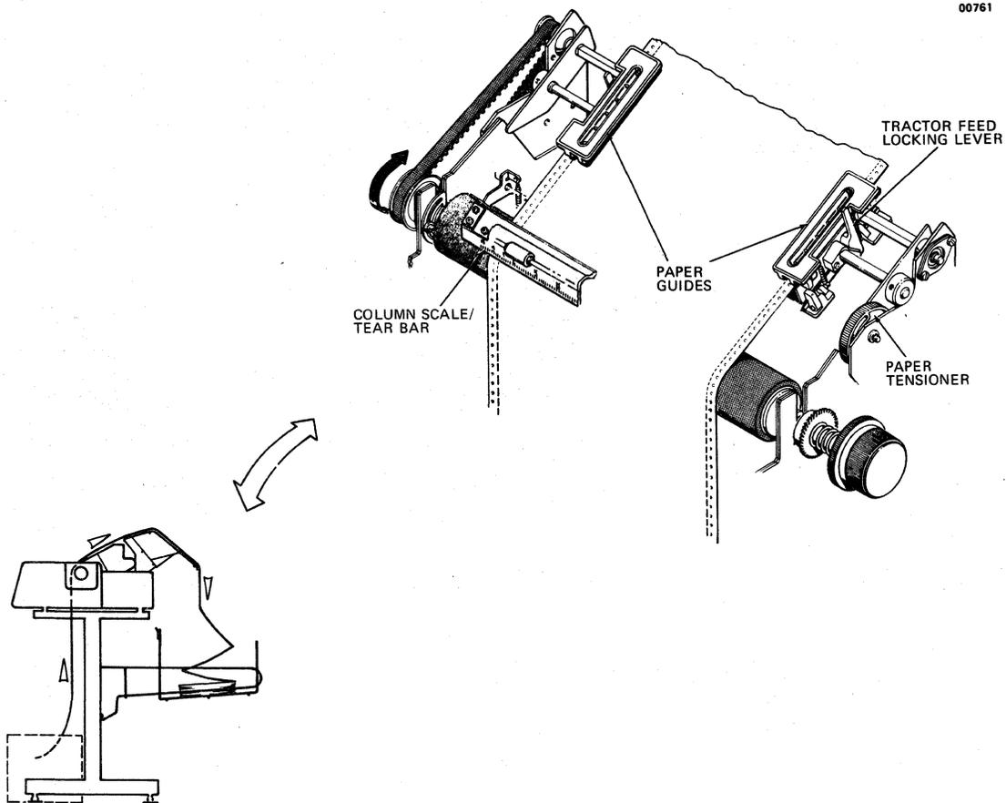
Figure 3-6 Loading paper, Bottom Tractor Feed
