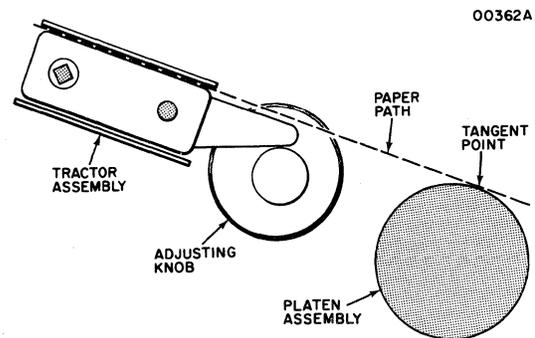
Figure 6-8 Paper Tension Adjustment
