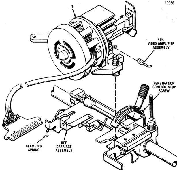
**Figure 7-2 Removal/Replacement, Print Head Assembly**
