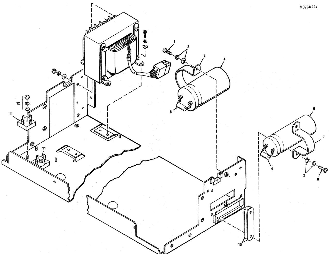
Figure 7-13 Removal/Replacement, Capacitor/Diode Bridges
