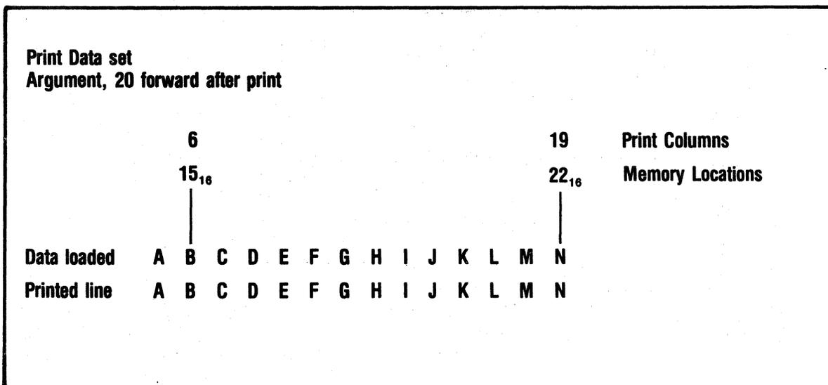
Figure 2-7 Printing Simple Line of Characters, Example 1
