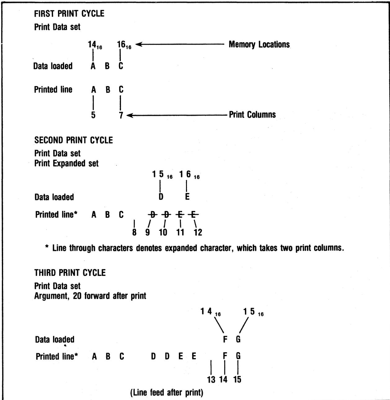
Figure 2-14 Printing Expanded Characters, Example 7
