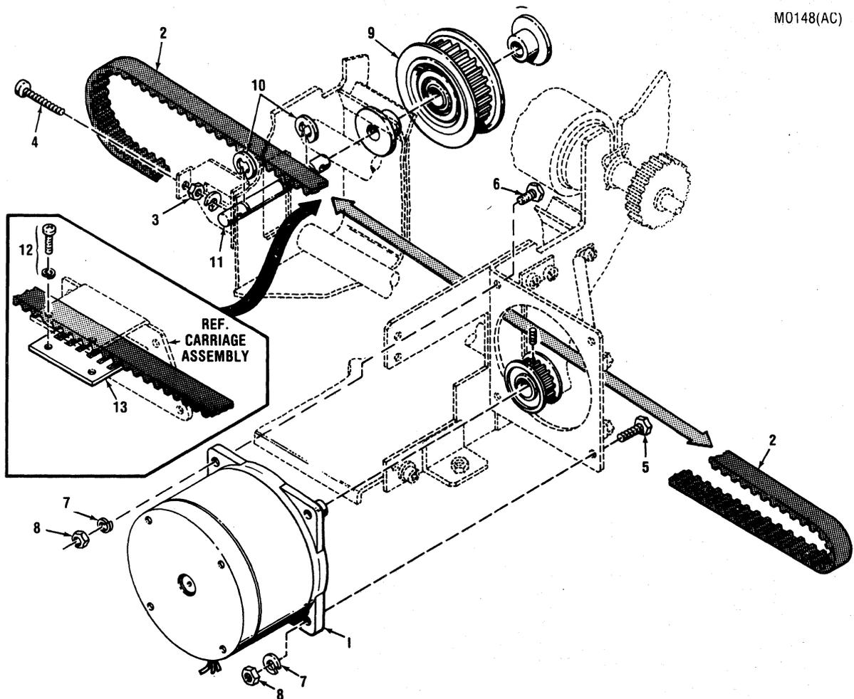
Figure 7-8 Removal/Replacement, Stepper Motor Assembly, Carriage Drive
