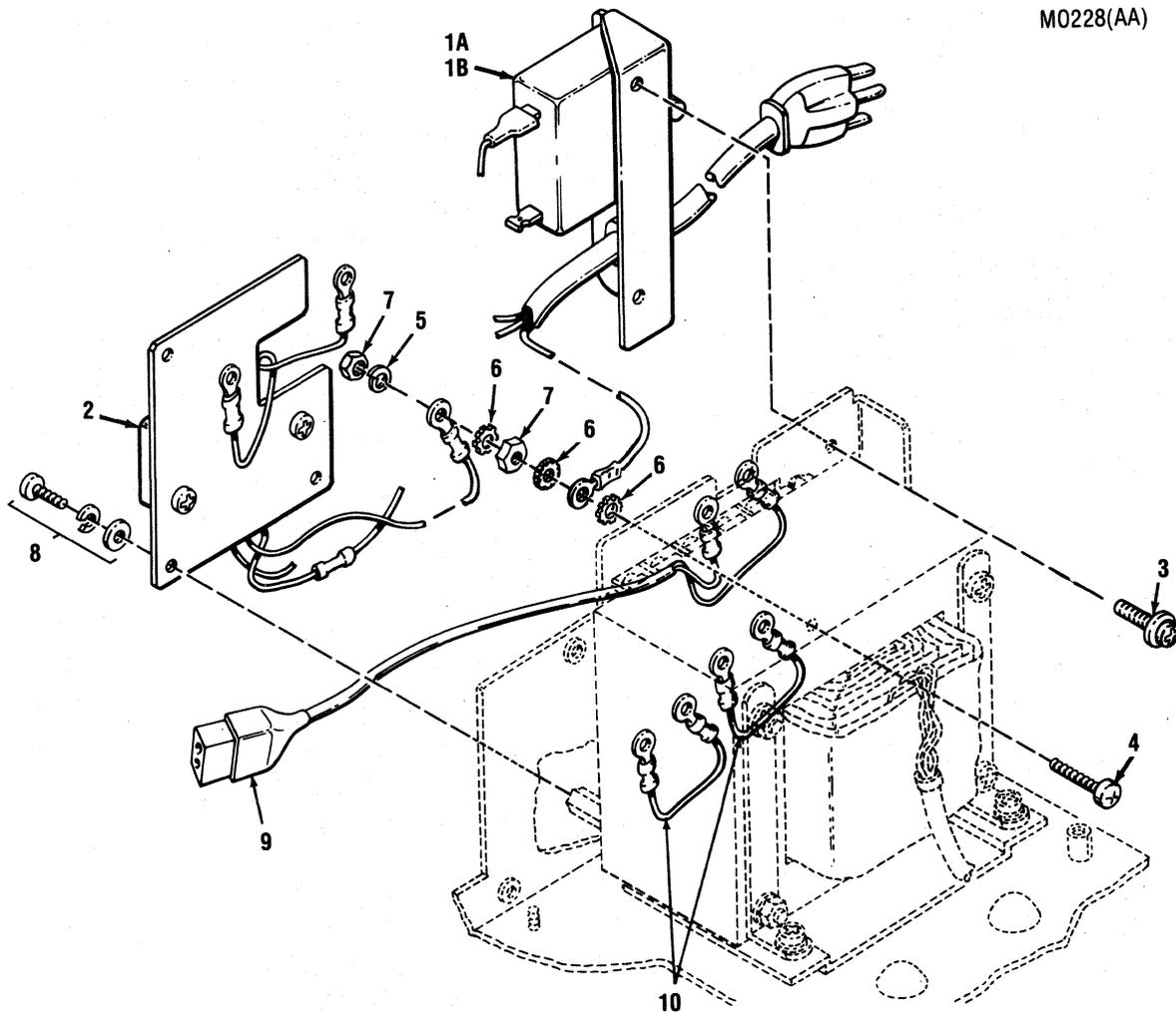
Figure 7-12 Removal/Replacement, Primary Voltage Assembly
