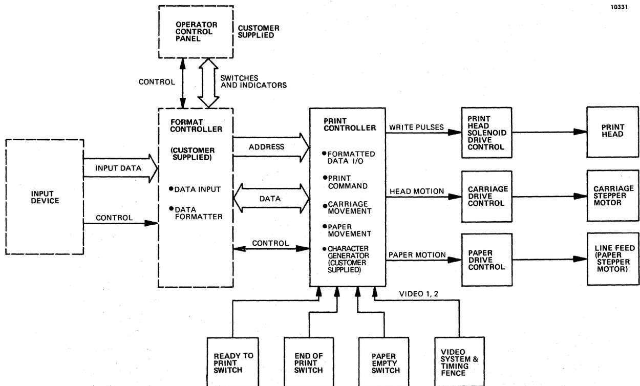
**Figure 1-3 Basic Printer Block Diagram**
