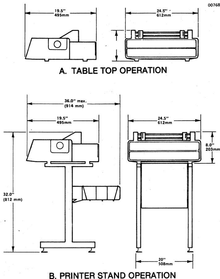
**Figure 3-1 Printer Dimensions**
