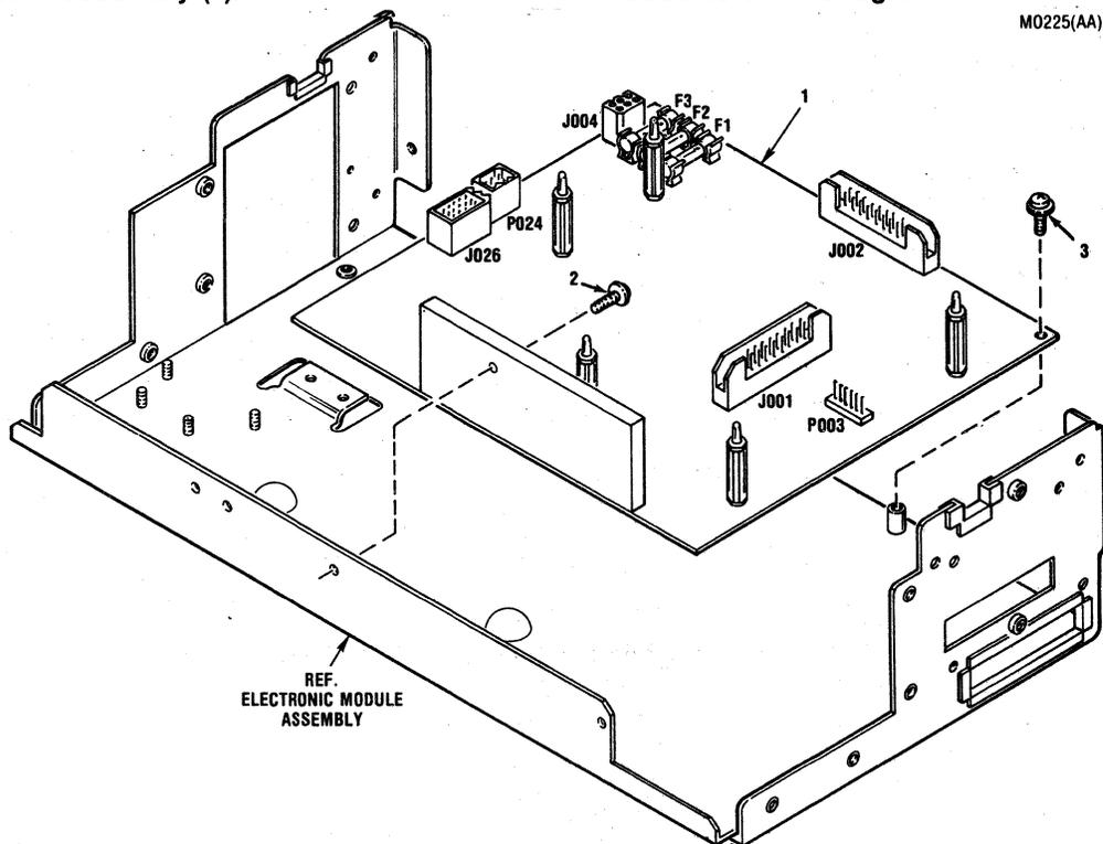
Figure 7-15 Removal/Replacement, Logic Board Assembly
