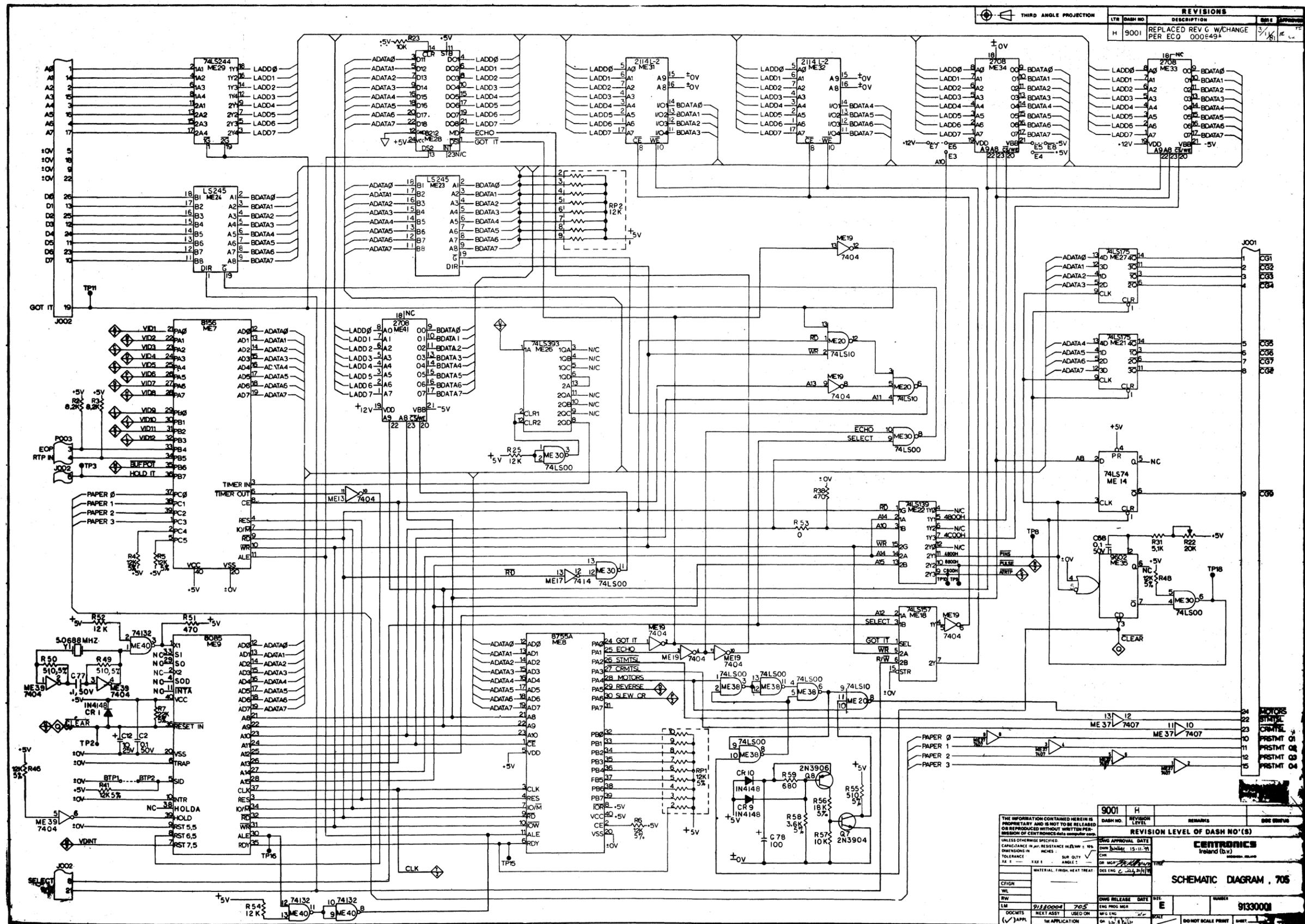
Figure A-1 Schematic Diagram, Model 705 Logic Board (Revision E, Sheet 1 of 2)
