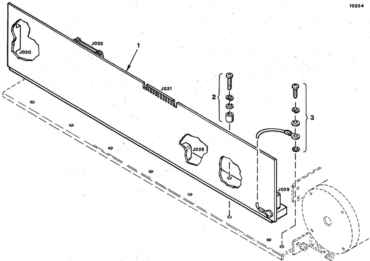
Figure 7-4 Removal/Replacement, Power Driver Board Assembly
