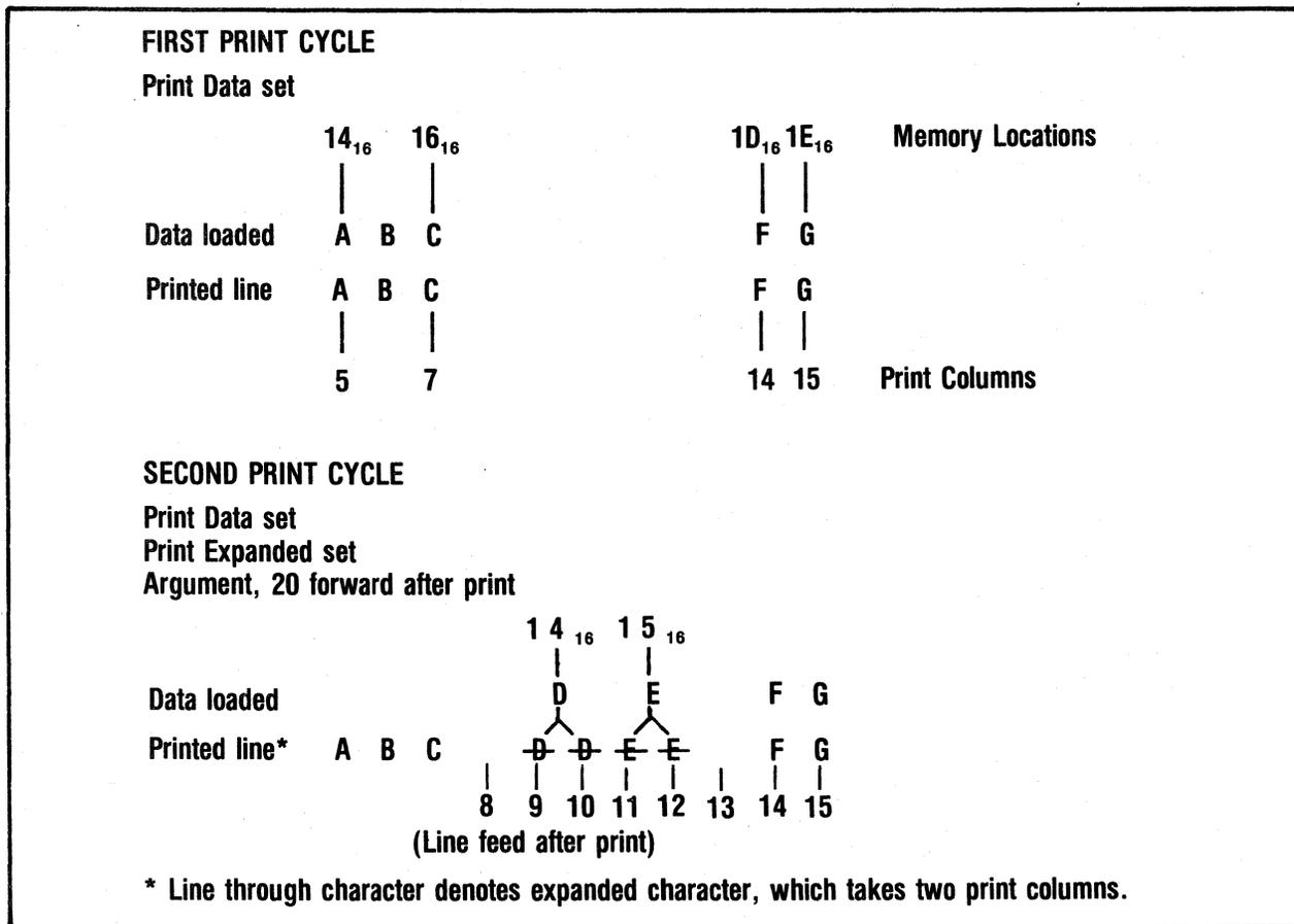
Figure 2-13 Printing Expanded Characters, Example 6
