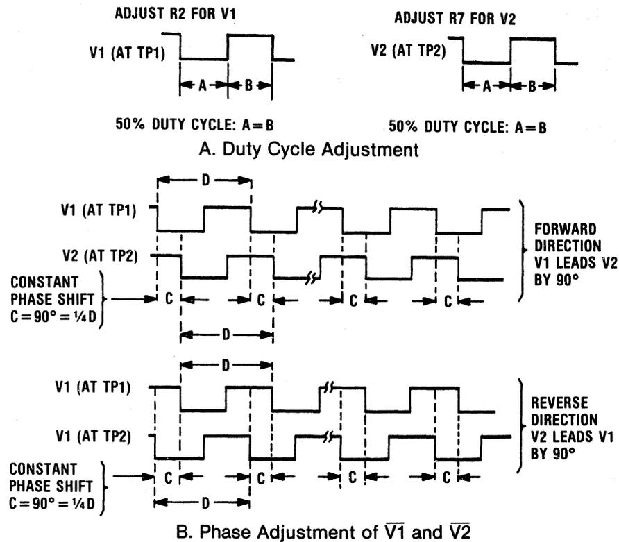
Figure 6-11 Duty Cycle and Phase Adjustment of Video Amplifier
