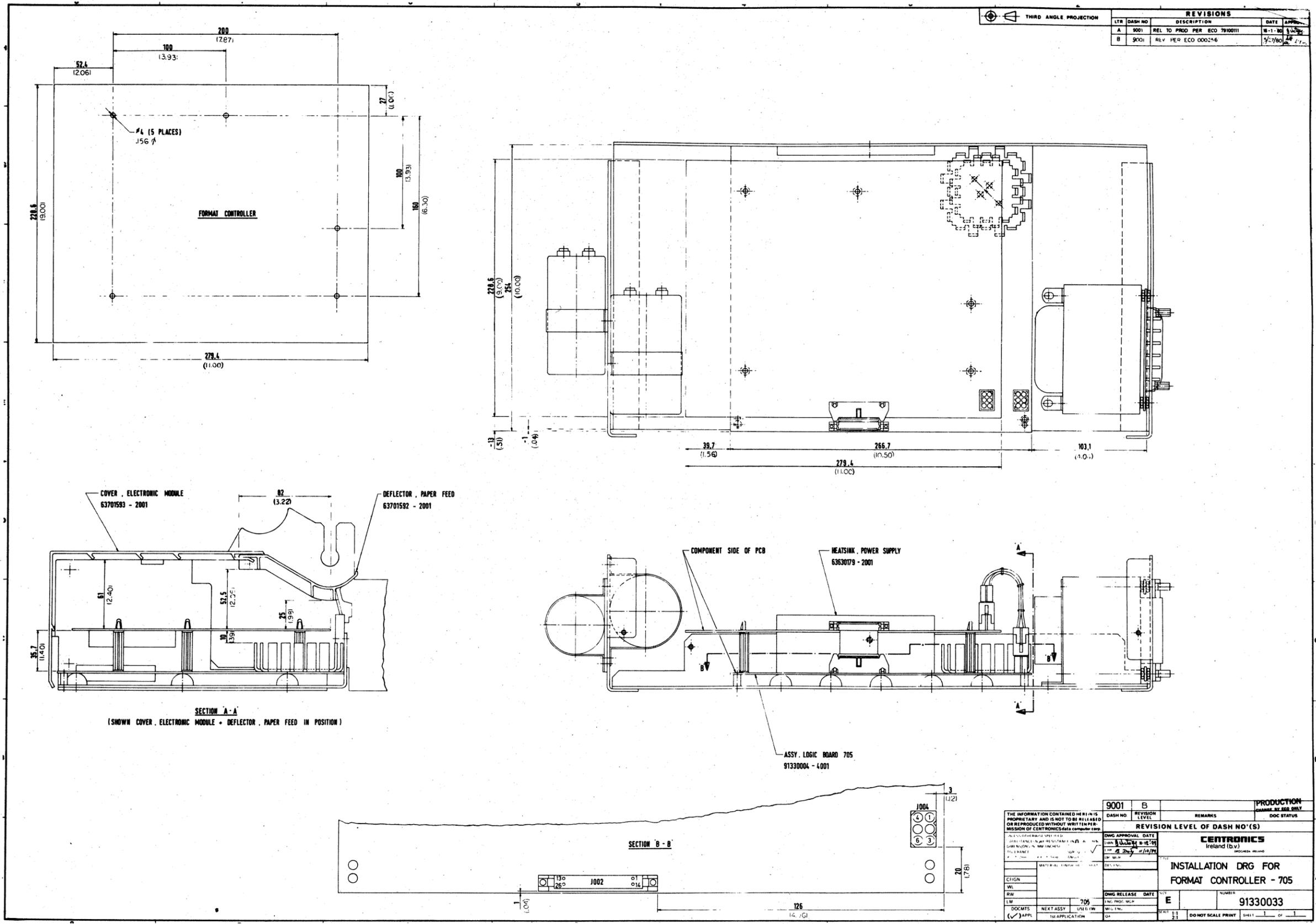
Figure B-2 Format Controller 705 Installation Dimensions
