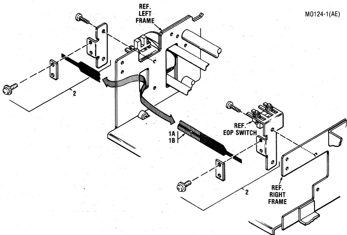
Figure 7-5 Removal/Replacement, Timing Fence Assembly
