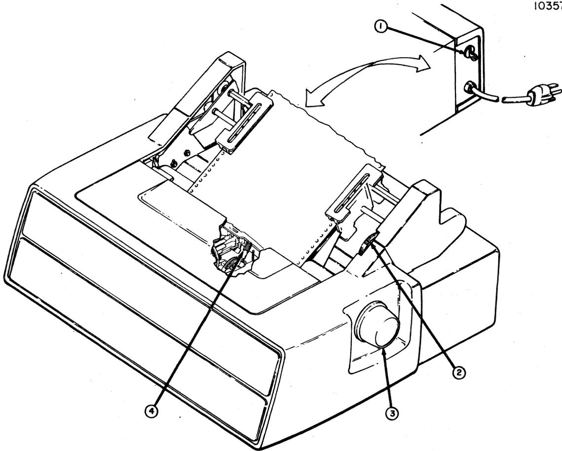
**Figure 3-3 Controls, Printer Mechanism**
