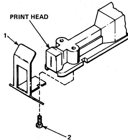
**Figure 7-3 Removal/Replacement, Ribbon Guide**
