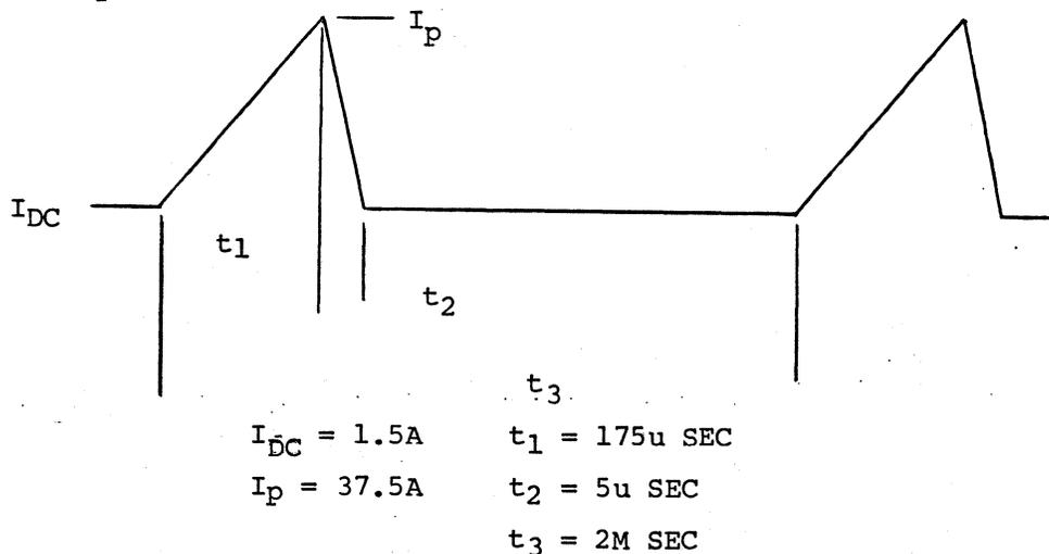
Figure 2. DYNAMIC LOADING FOR +35V OUTPUT
