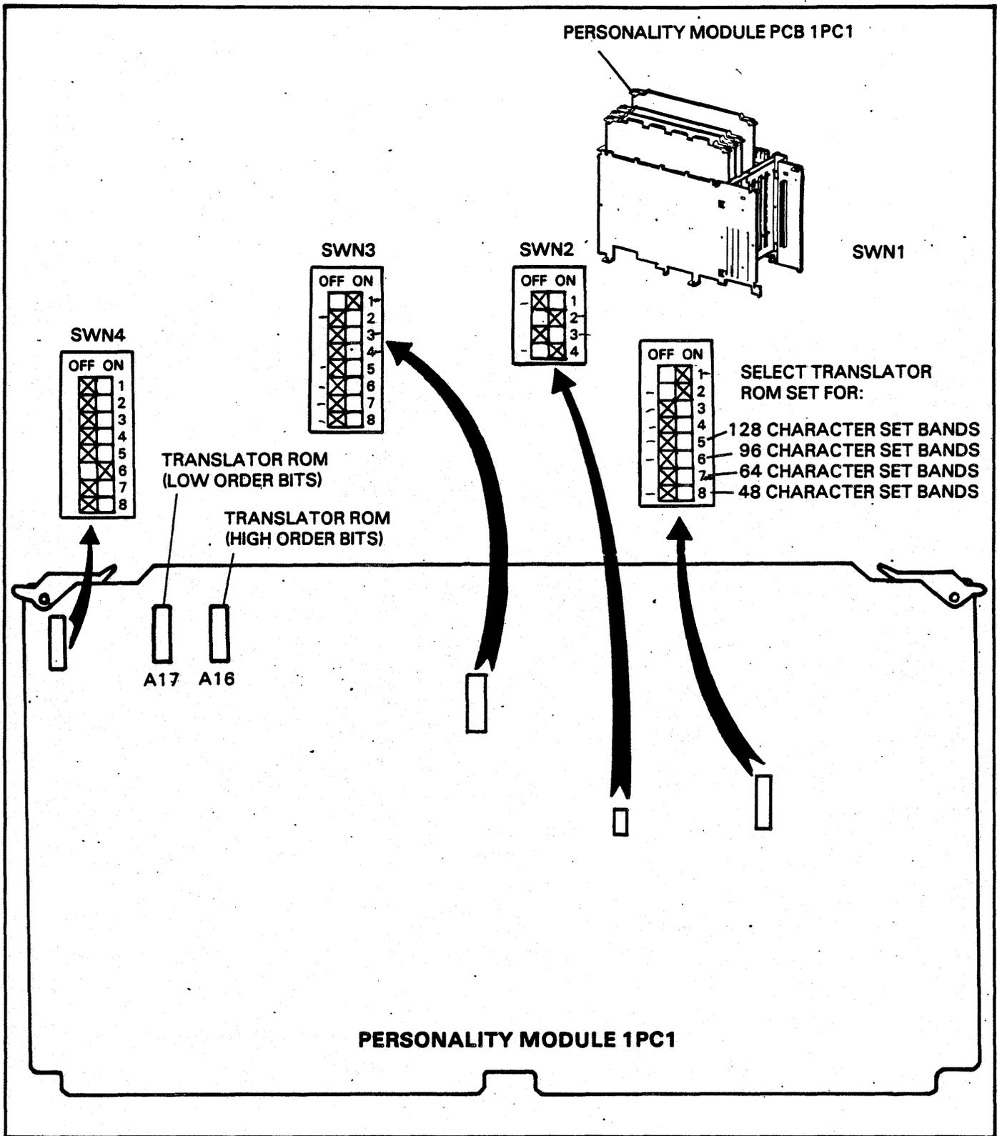
**FIGURE 1-1. PERSONALITY MODULE (1PC1) FACTORY SWITCH SET-UP AND TRANSLATOR ROM LOCATIONS (FOR ASSEMBLY NUMBER 44682847/48).**
