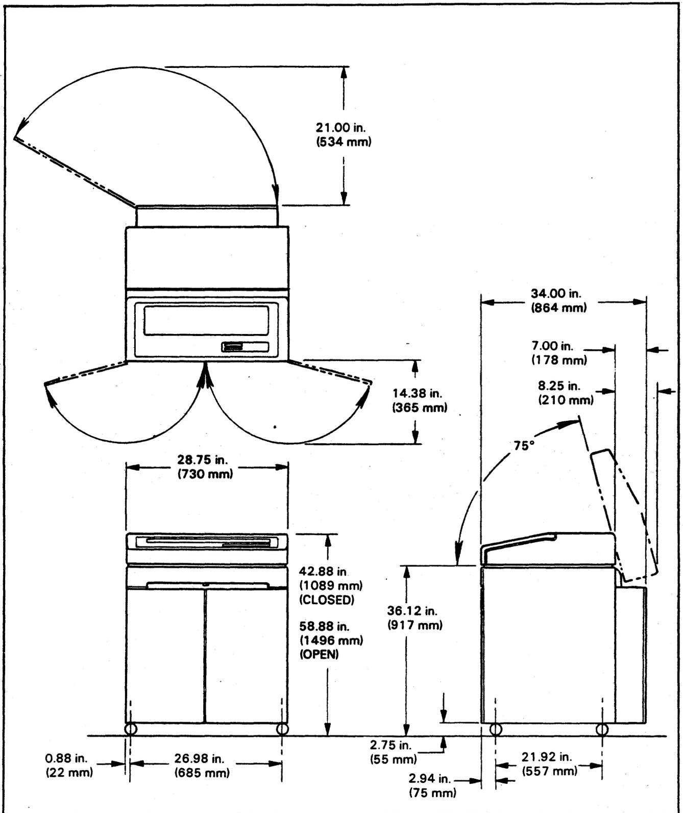
FIGURE 3-2. SERVICE ACCESS SPECIFICATIONS (WITH FRONT DOORS)
