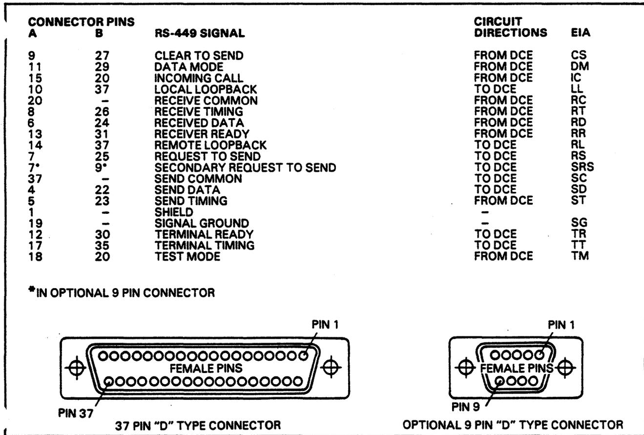
FIGURE 5-2. I/O SIGNALS AND PIN ASSIGNMENTS – RS-449 CONNECTOR
