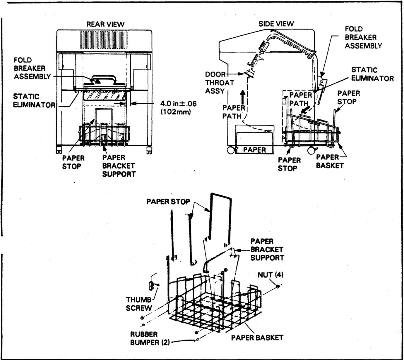
FIGURE 1-6. PAPER BASKET INSTALLATION AND SET-UP
