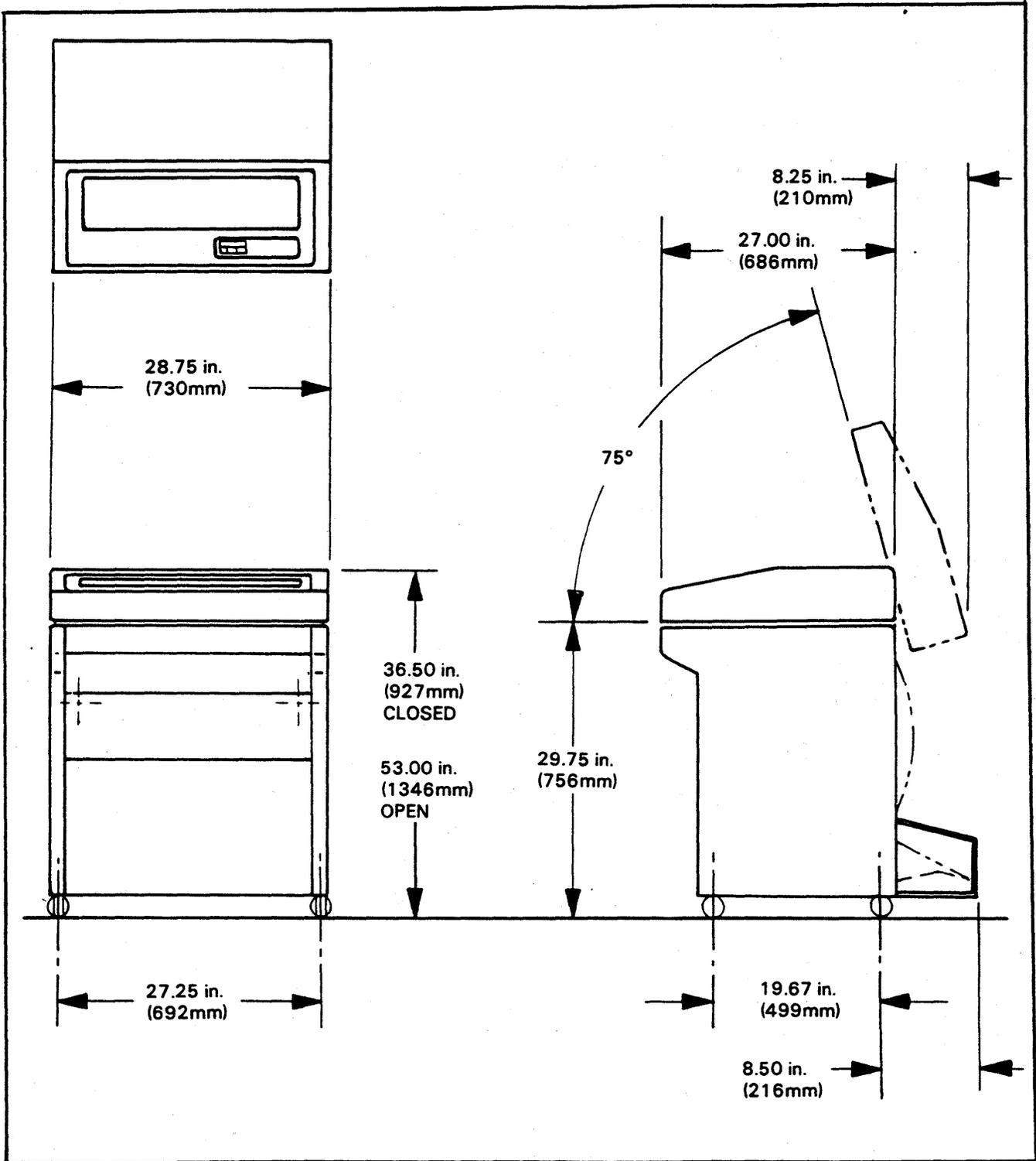
FIGURE 3-1. SERVICE ACCESS SPECIFICATIONS (WITHOUT FRONT DOORS)
