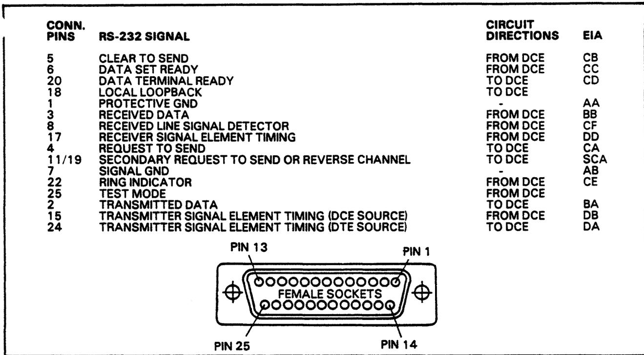
FIGURE 5-1. I/O SIGNALS AND PIN ASSIGNMENTS – RS-232 CONNECTOR
