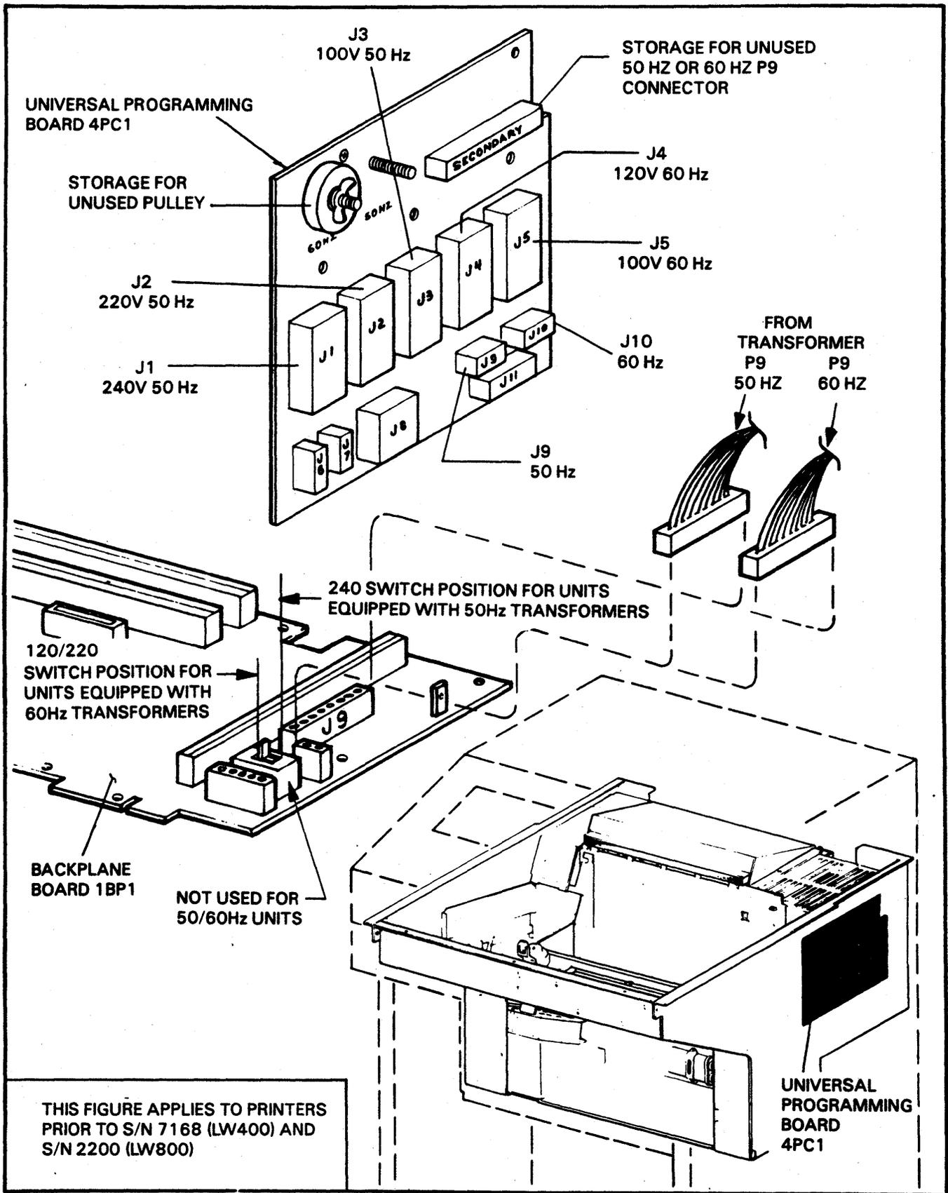
FIGURE 4- . INPUT POWER/FREQUENCY MODIFICATIONS (EARLY UNITS)
