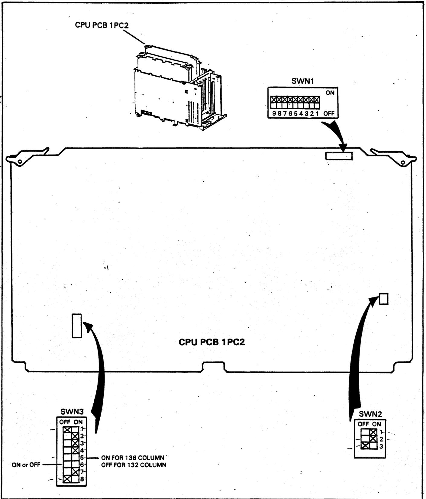
FIGURE 1-2. CPU (1PC2) FACTORY SWITCH SET-UP
