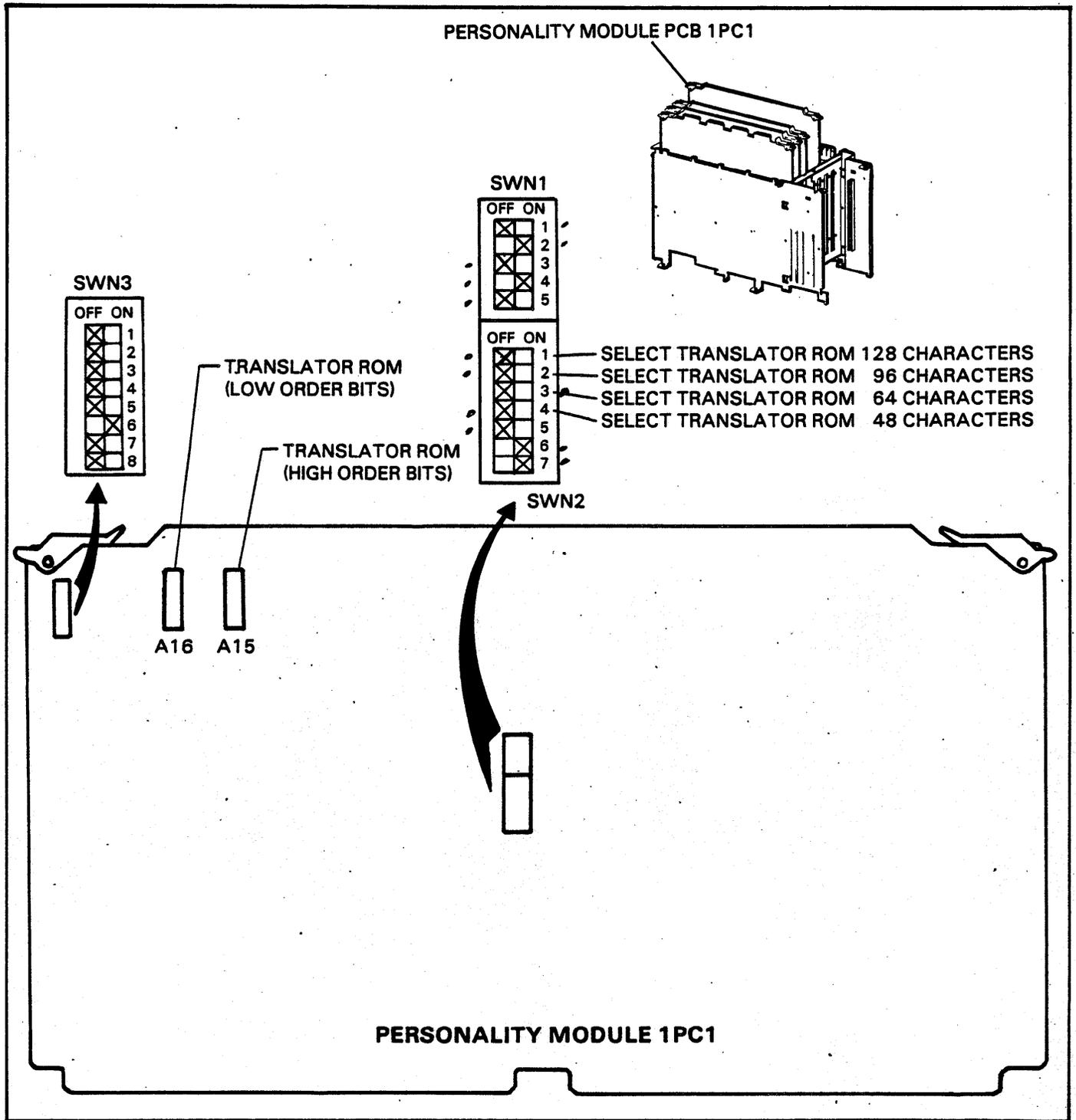
**FIGURE 1-1. PERSONALITY MODULE (1PC1) FACTORY SWITCH SET-UP AND TRANSLATOR ROM LOCATIONS (FOR ASSEMBLY NUMBER 44682846).**
