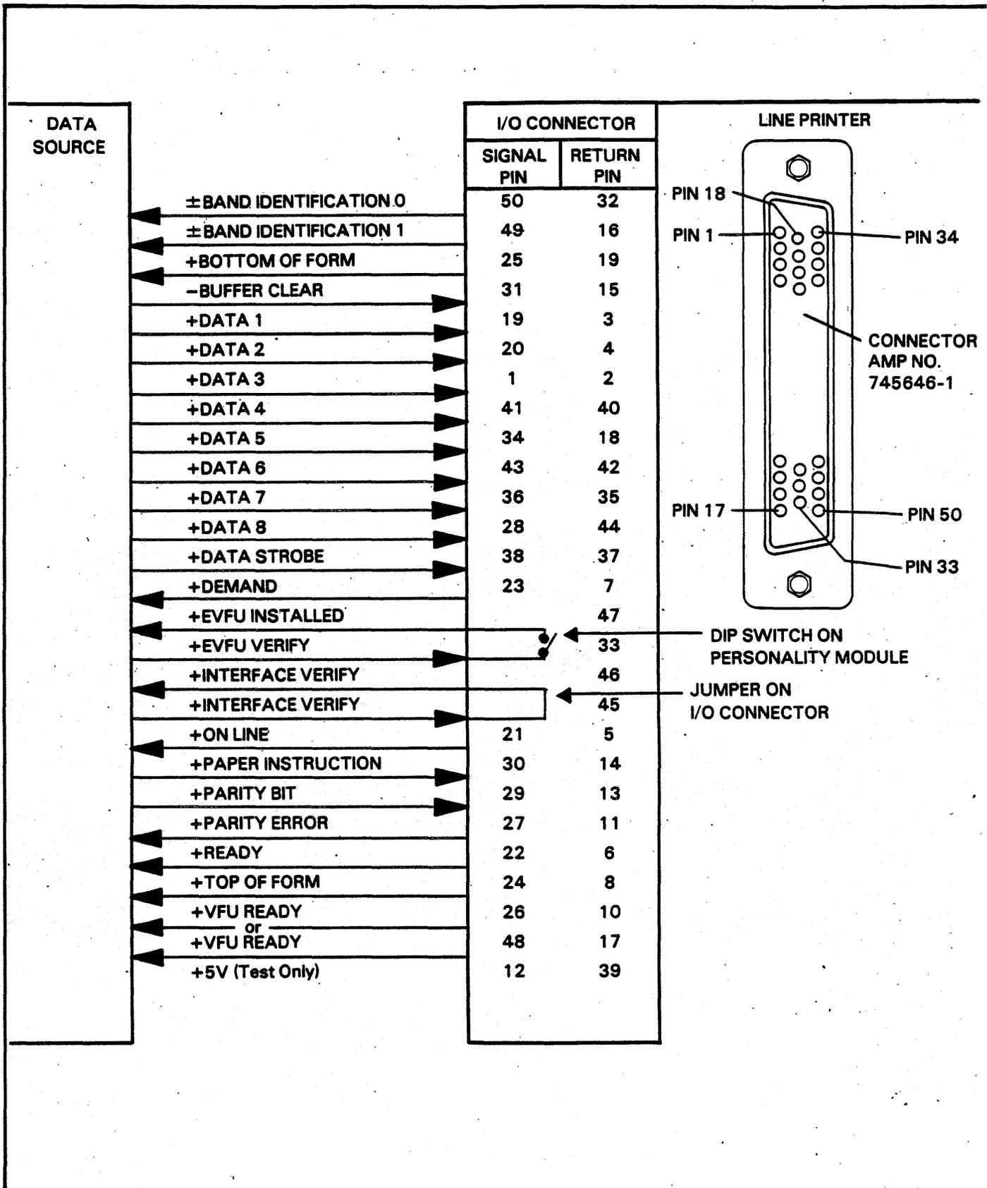
FIGURE 1-6. I/O SIGNALS AND PIN ASSIGNMENTS-"D" TYPE CONNECTOR
