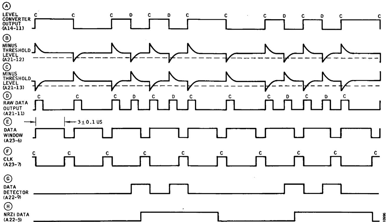
Figure 3-37. RAW and NRZ Read Data Decoder Waveforms
