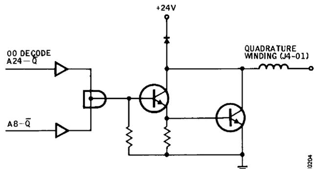
Figure 3-27. Decode and Current Drivers for 00 Code
