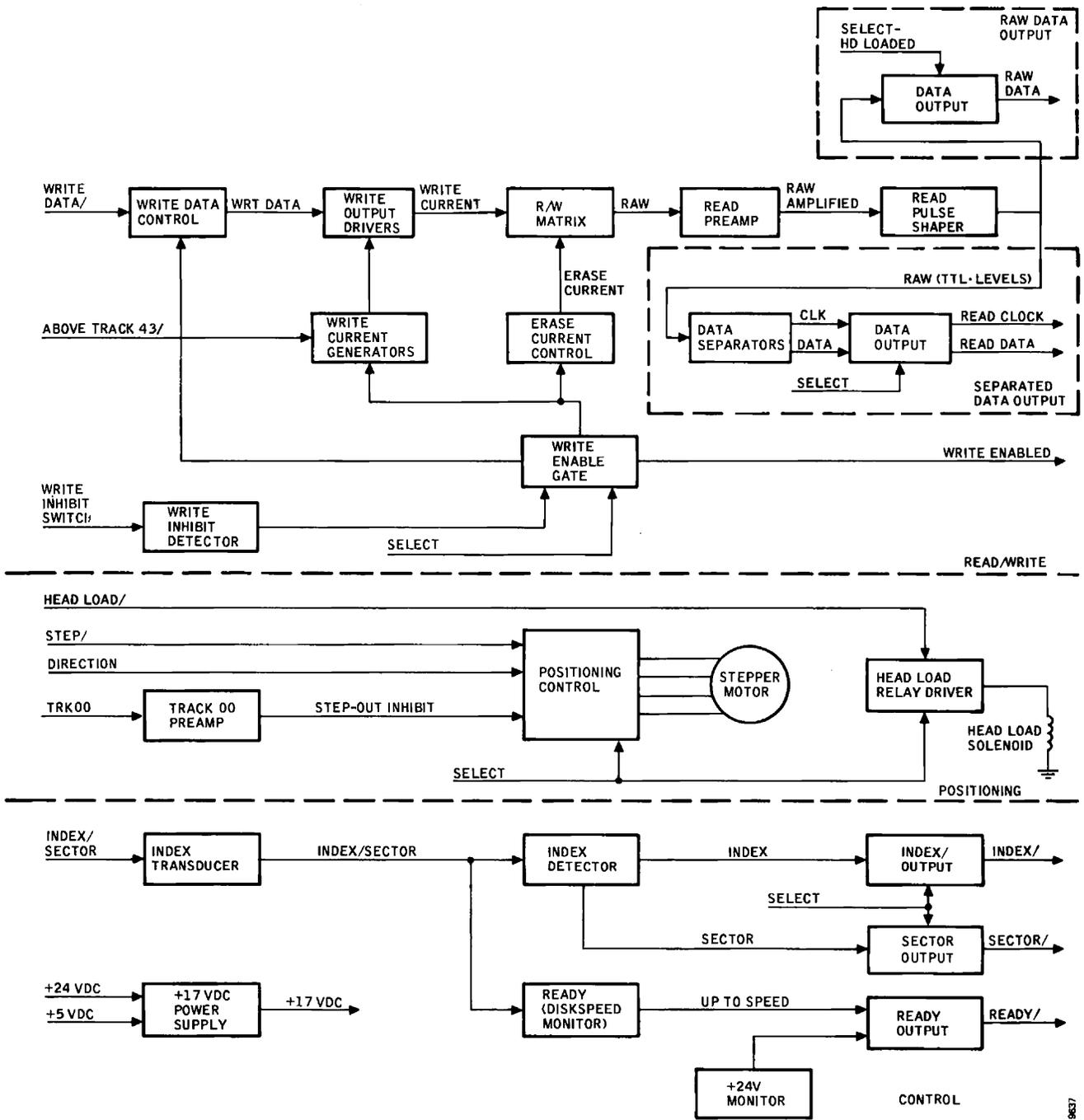
Figure 3-17. Detailed Block Diagram
