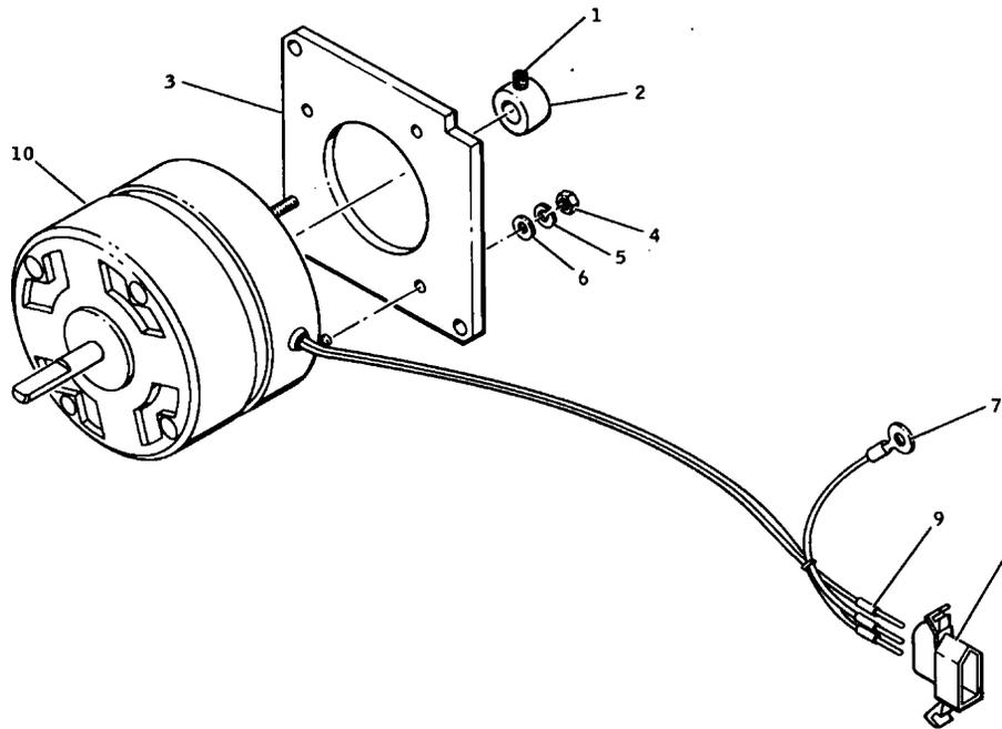
Figure 5-3. Drive Motor Assembly
