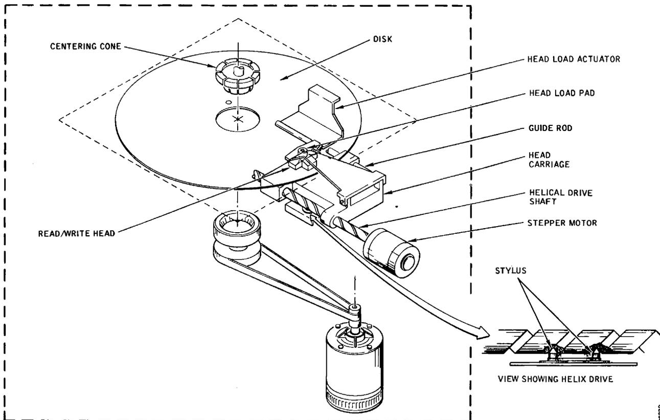
Figure 3-12. Disk Drive Mechanical System Pictorial View
