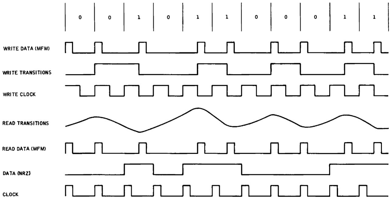
Figure 3-42. Read/Write Coding Waveforms
