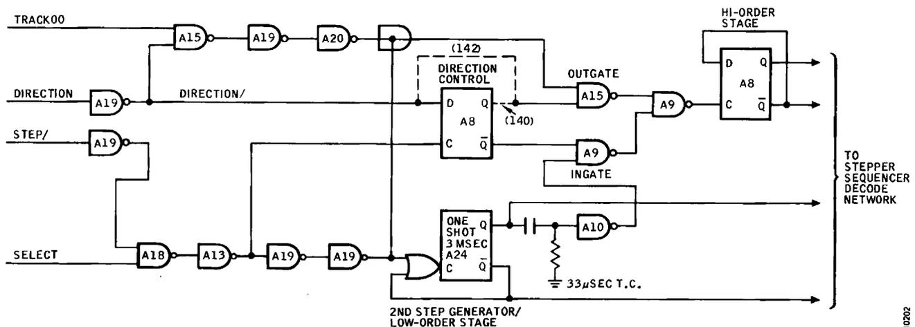
Figure 3-25. Stepper Motor Position Control Simplified Logic Diagram
