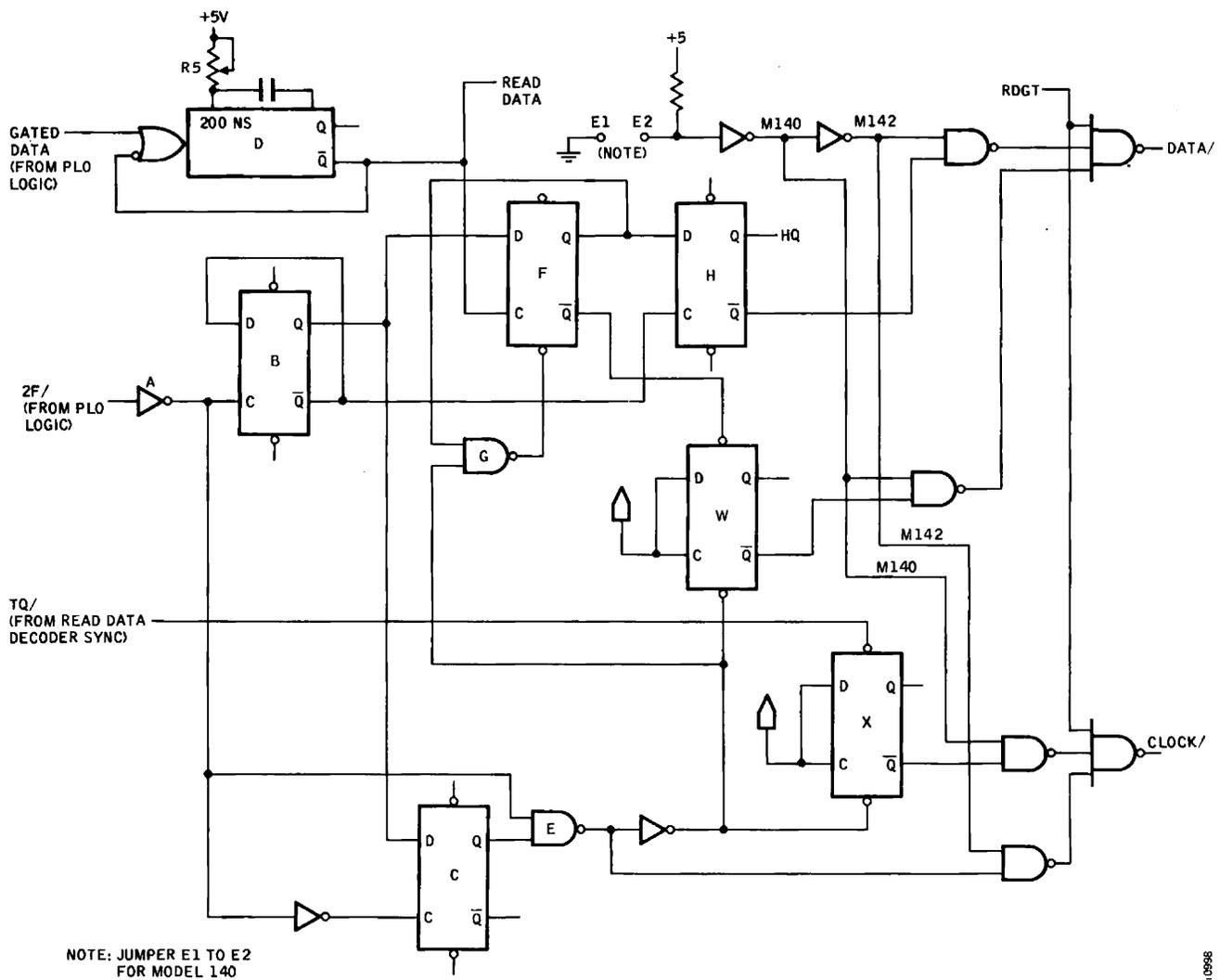
Figure 3-43. Data Decoder, Simplified Logic Diagram
