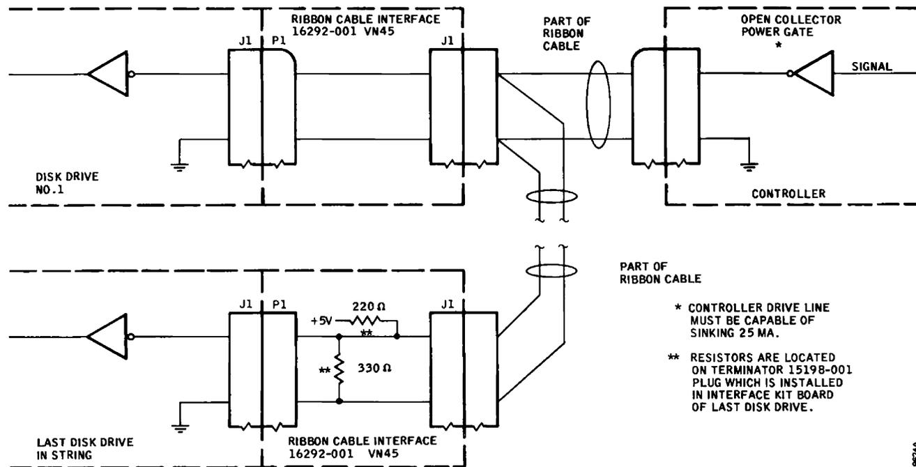
Figure 2-6. Termination for Disk Drive Input Signals
