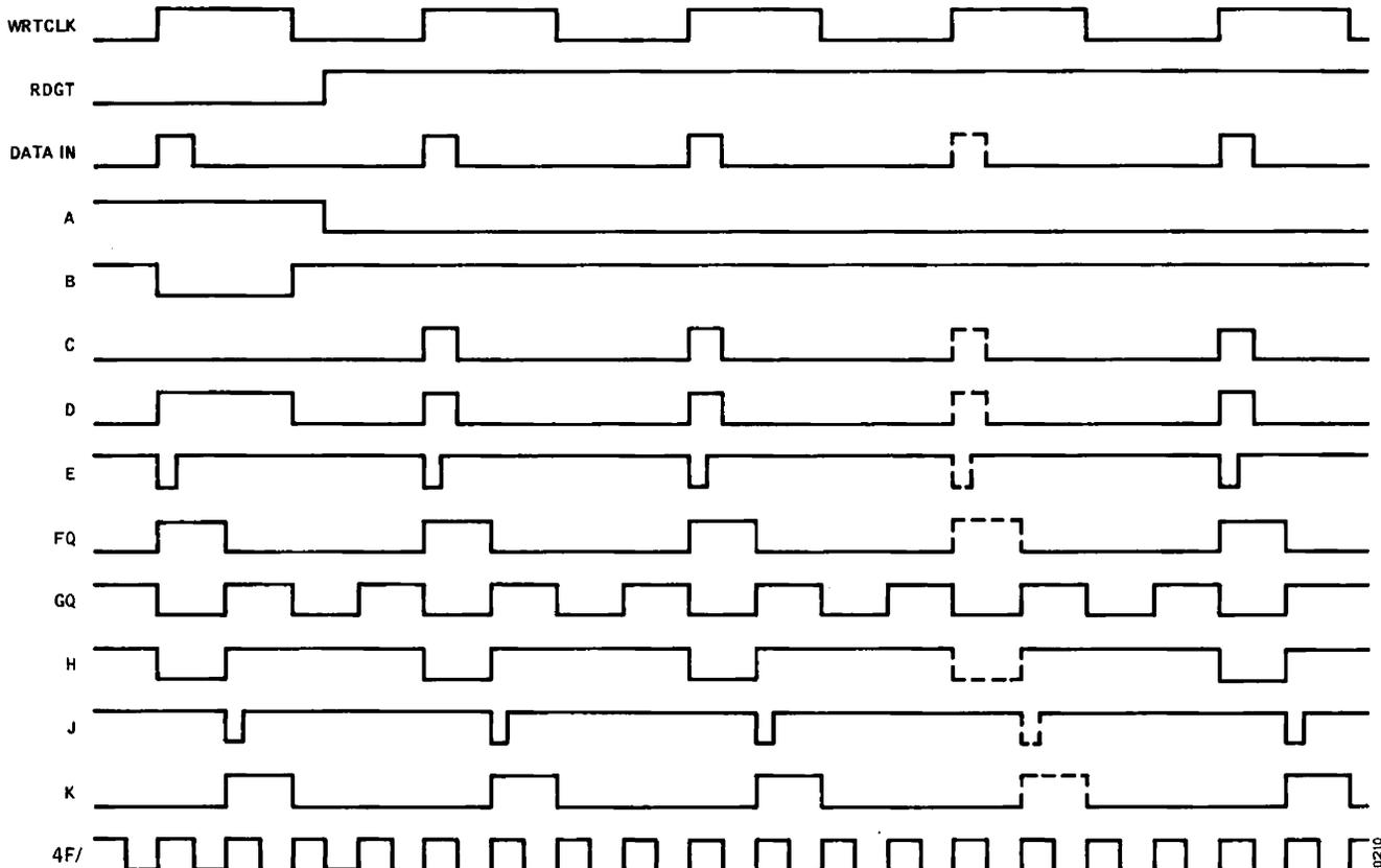
Figure 3-40. PLO Locked On and Missing Pulse Operation
