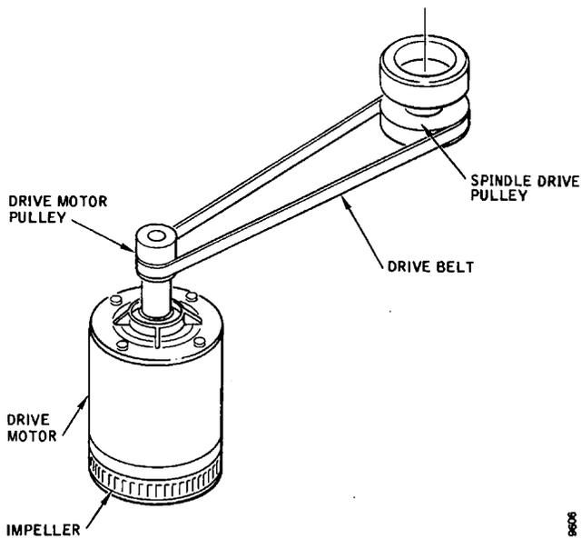
Figure 3-13. Drive Mechanism
