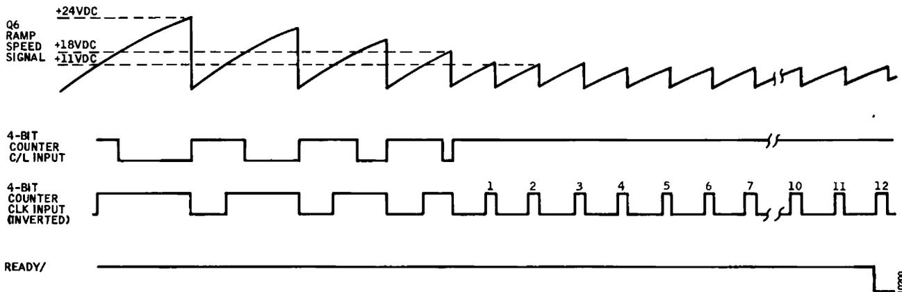
Figure 3-21. Power-On to Ready Transition Period Waveforms
