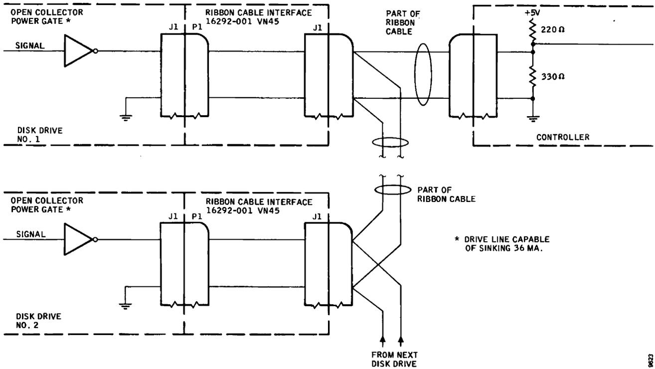
Figure 2-5. Termination for Disk Drive Output Signals
