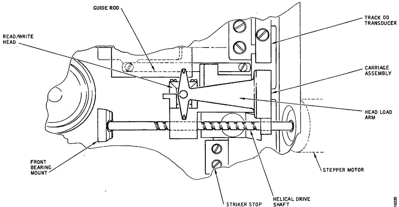
Figure 3-15. Positioning Mechanism
