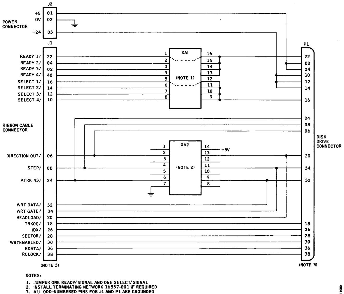
Figure 2-4. Ribbon Cable Interface Connector Board, Schematic Diagram
