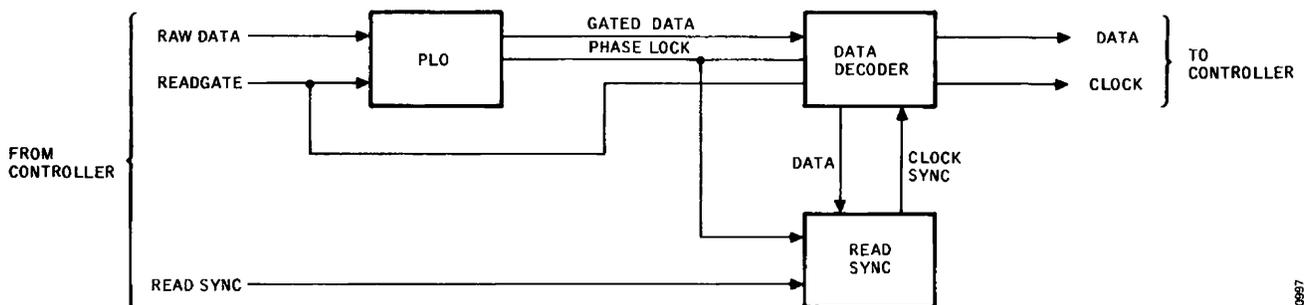
Figure 3-38. Read Decoder with PLO Block Diagram
