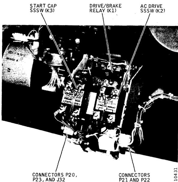
Figure 3-22. Sequence Relay Assembly Component Locations
