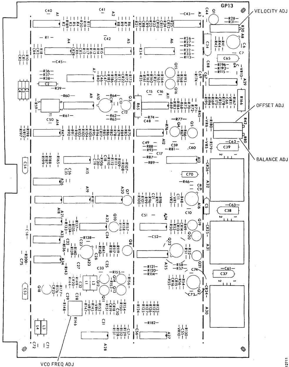
Figure 3-8. Servo Control Card Adjustment Point Locations
