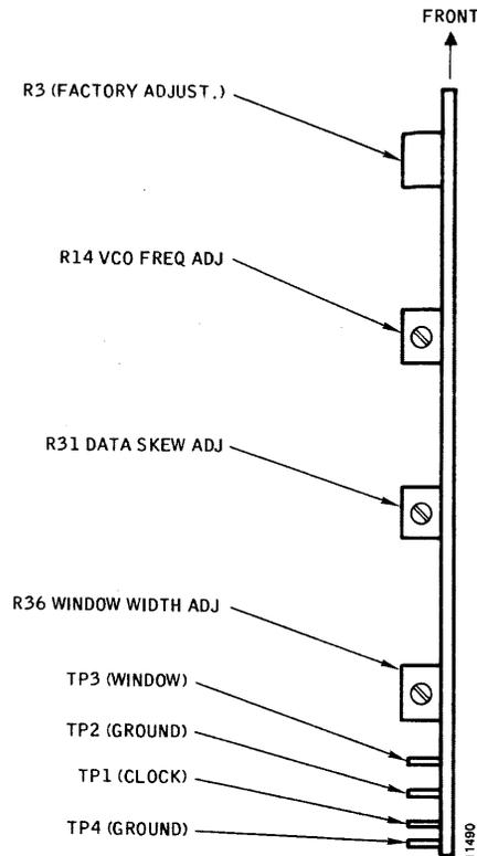
Figure 3-14. Data Separator Test and Adjustment Points (T80)
