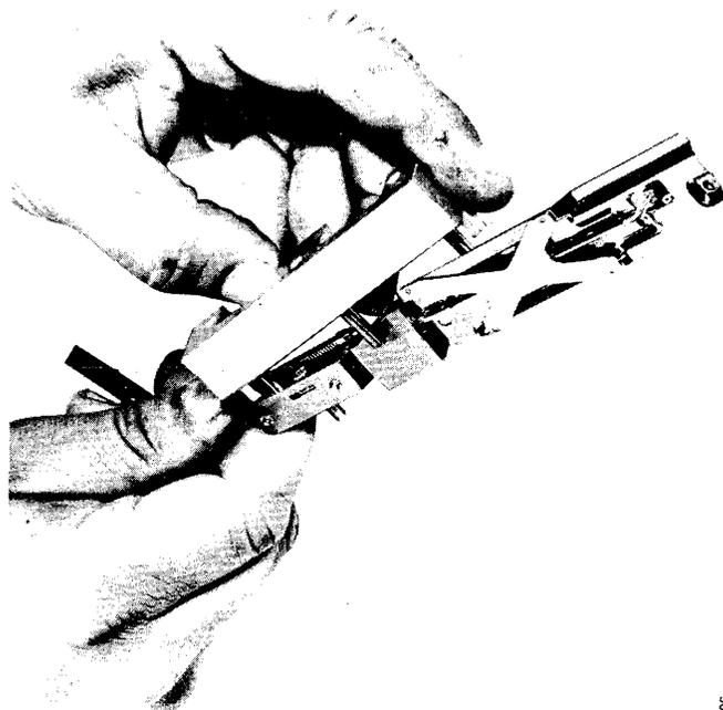
Figure 3-1. Head Camming Tool Installation
