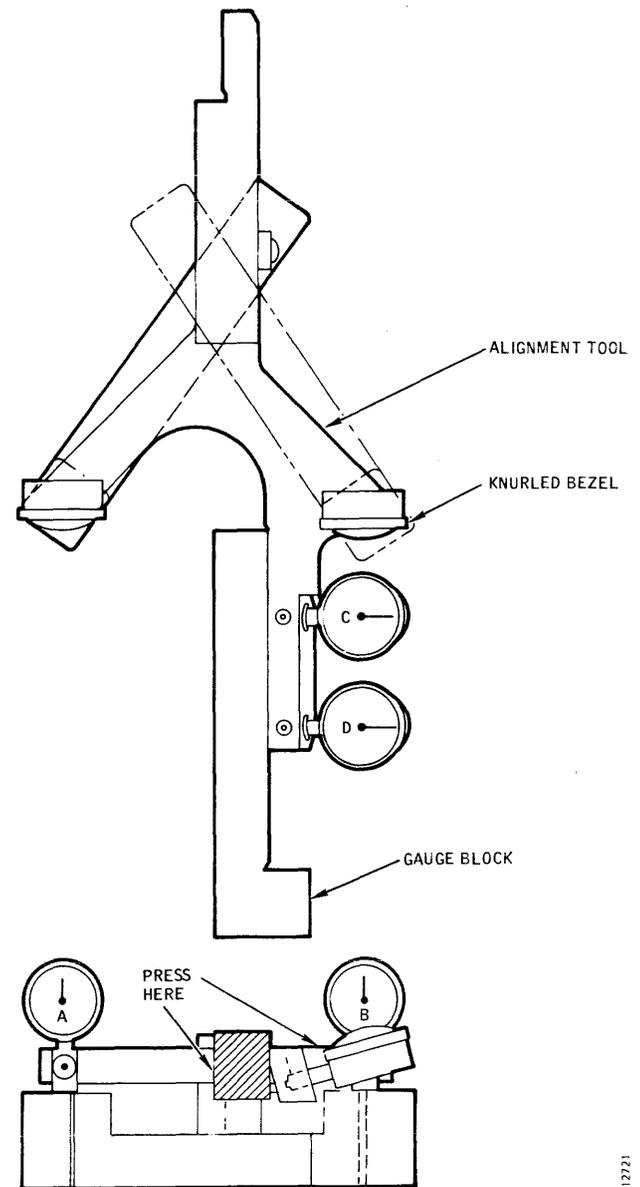
**Figure 4-10. Calibration of Alignment Tool Indicators**
