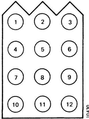
**Figure 3-21. Connector J30 Pin Locations**
