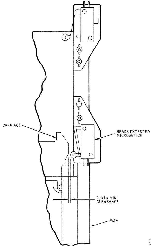
**Figure 3-19. Microswitch Adjustment Clearance**
