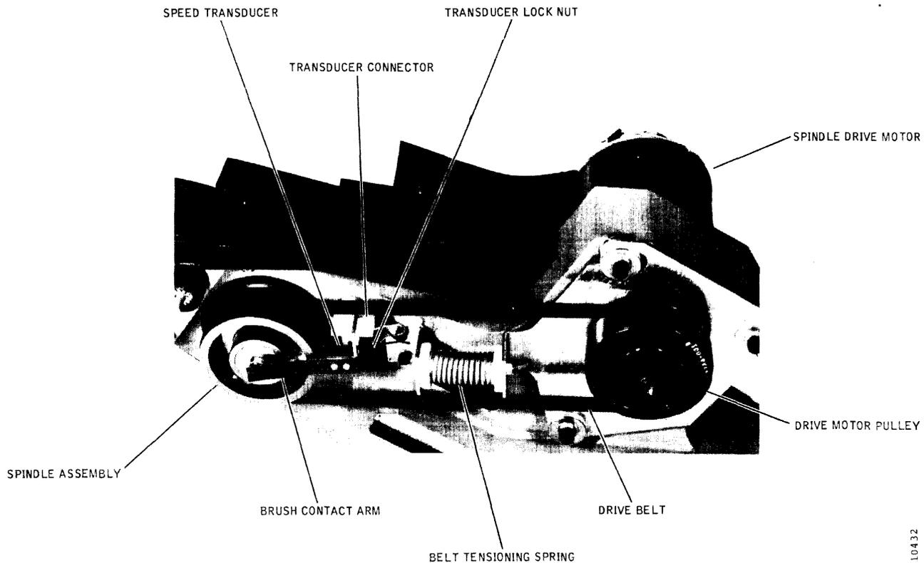
**Figure 3-24. Spindle Drive Component Locations**
