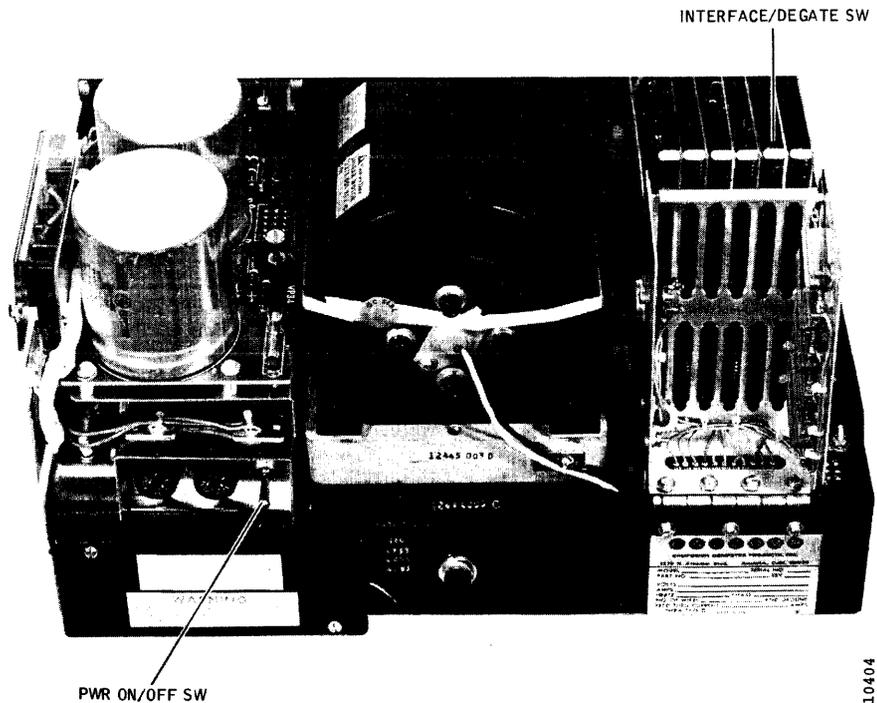
Figure 1-4. Location of Maintenance Switching
