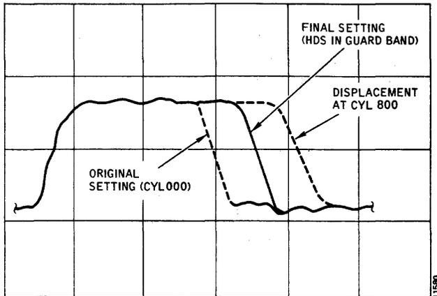
**Figure 3-15. Clock Frequency Adjustment Waveform (T80)**
