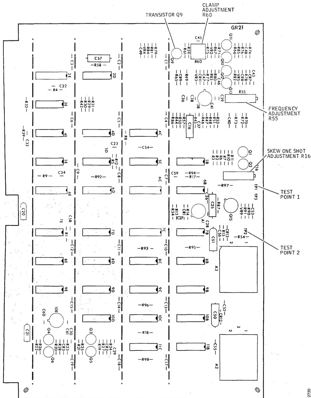
Figure 4-3. Data Separator Test and Adjustment Points (Early T80)
