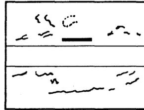
B. ALCOHOL RESIDUE. HEAD MUST BE CLEANED
