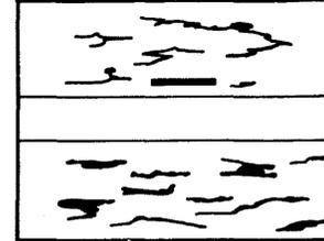
E. CRASHED (USUALLY BURNED). HEAD MUST BE REPLACED
