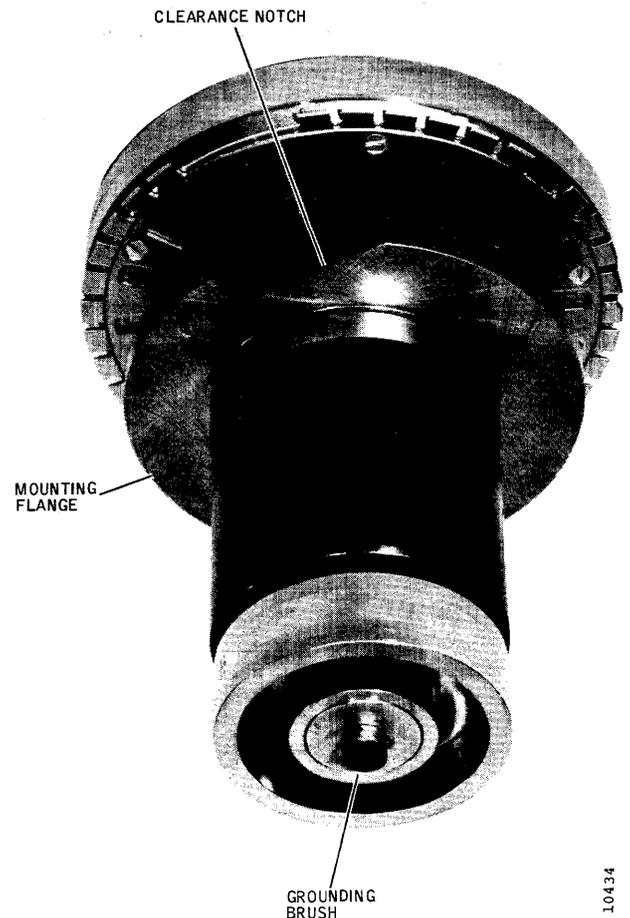
Figure 3-27. Spindle Assembly
