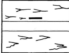
D. OXIDE BUILDUP DUE TO SCRATCHES. HEAD MUST BE REPLACED
