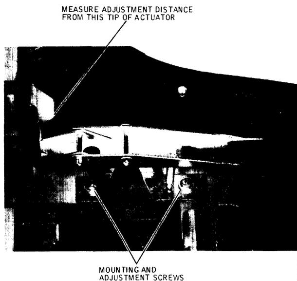
Figure 3-26. Spindle Lock Assembly
