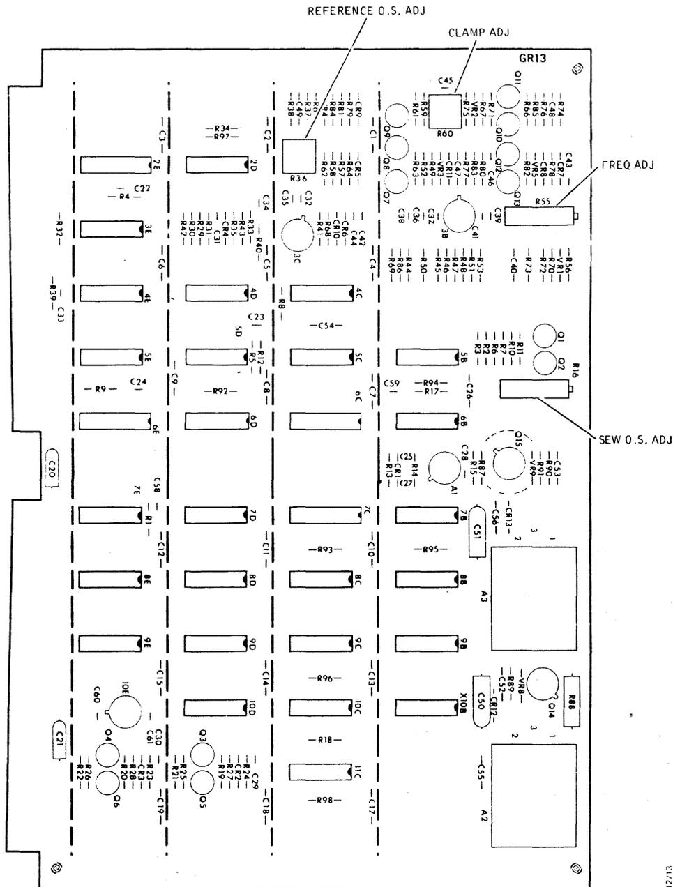
Figure 3-10. Data Separator Adjustment Point Locations (T25, T50)
