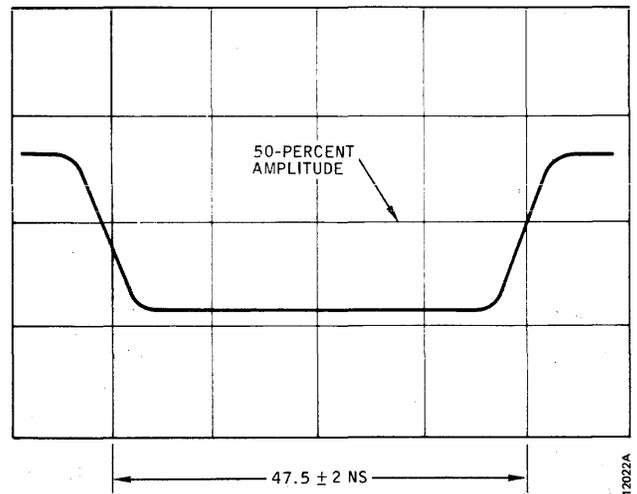
**Figure 3-16. Window Width Adjustment Waveform (T80)**
