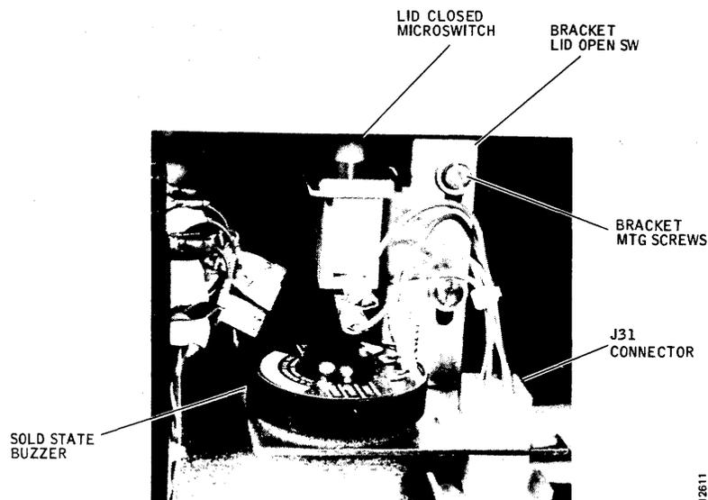
Figure 3-20. Lid Closed Switch and Solid State Buzzer Component Locations
