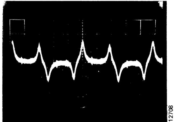
Figure 4-2. Head Alignment Dibit Waveforms
