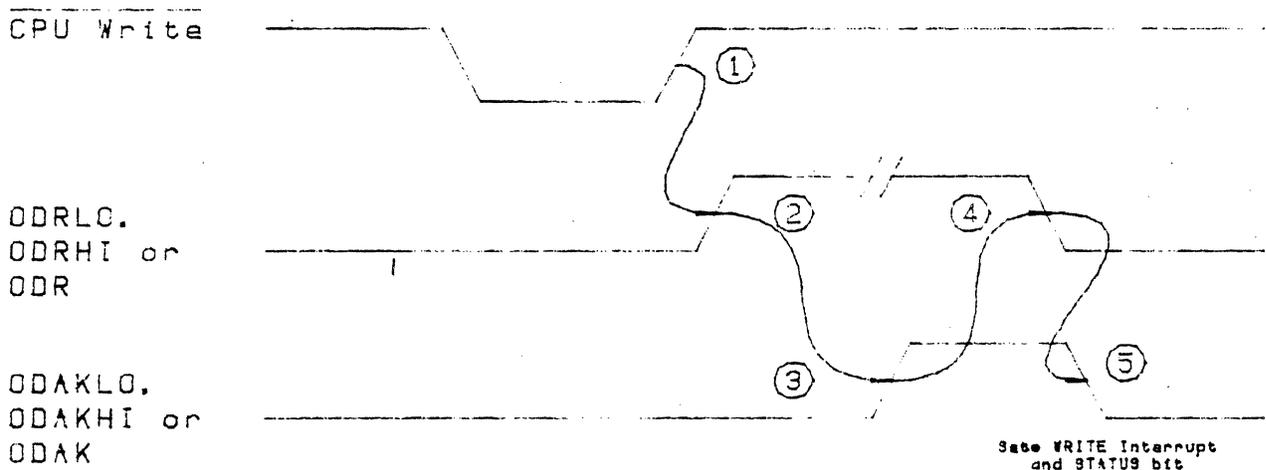
Figure 4-1. PIO Write Timing
