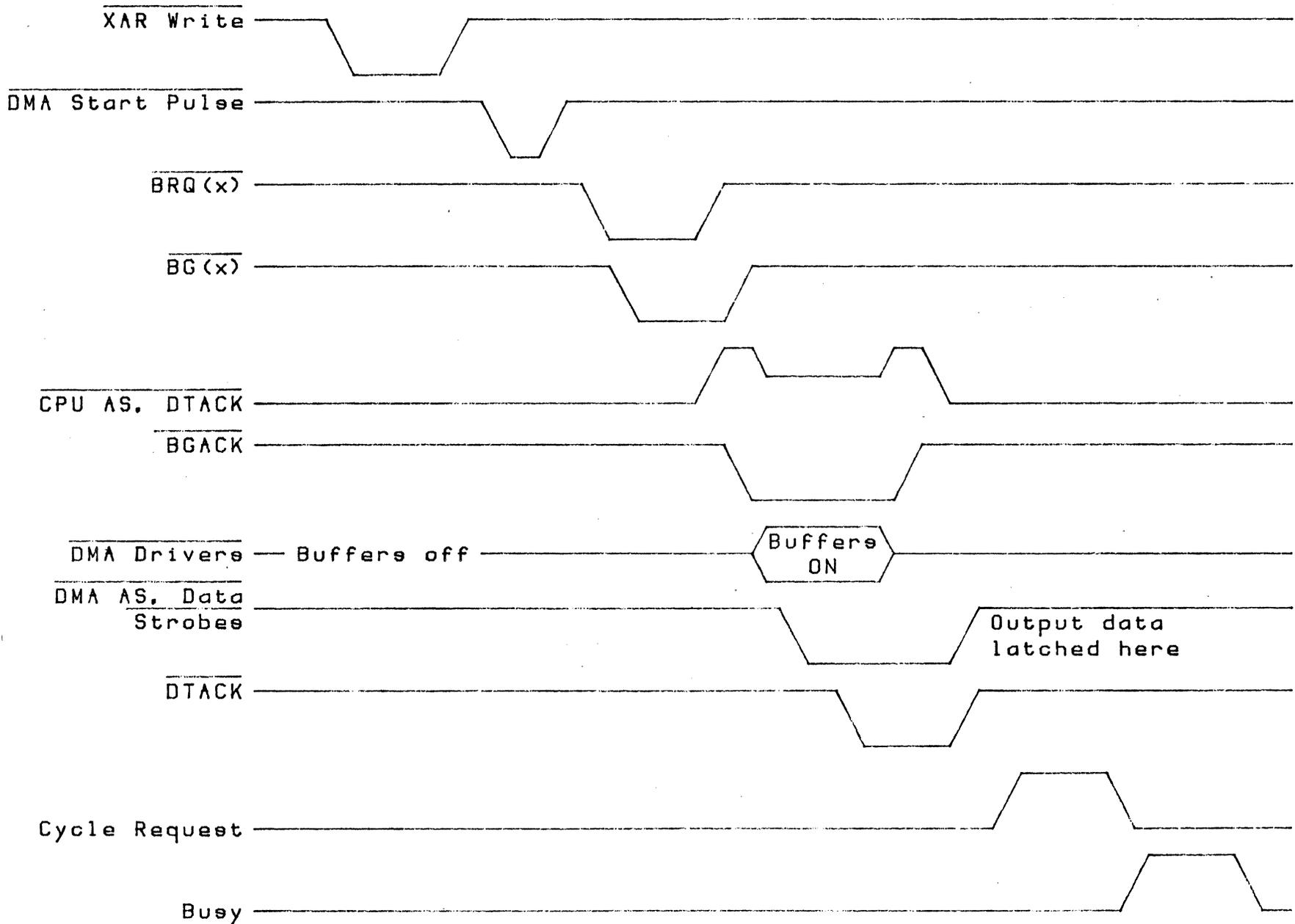
Figure 5-1. CGC to DEC Host Timing
