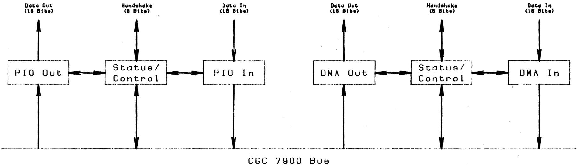
Figure 1-2. PIO/DMA Functional Diagram
