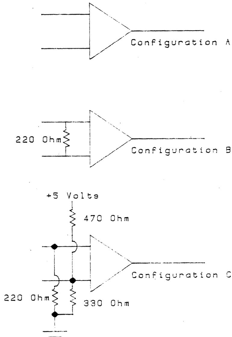
Figure 4-3. PIO Terminator Configurations
