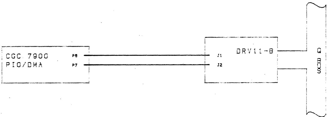
Figure 6-8. DRV11-B System Configuration
