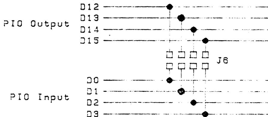
Figure 4-4. PIO Input Rerouting
