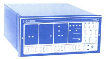
The CIP/2200 with its TTL logic elements including MSI has achieved a cost/performance that allows many tasks previously assigned to large computer systems, or hard wired controllers to be achieved much more efficiently on a CIP/2200.
