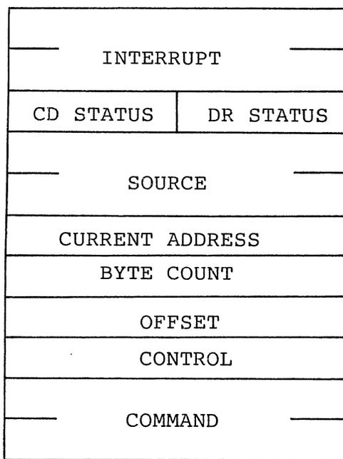
Figure 4-8 Exchange Parameter Block
