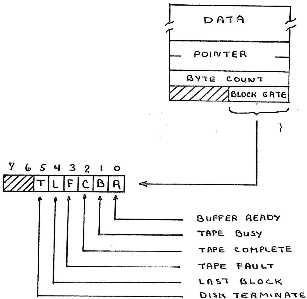
Figure 5-2 Streaming Block Header
