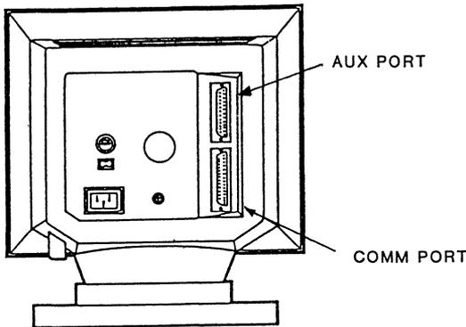
**Figure 2-2. Back View of the Display Unit**
