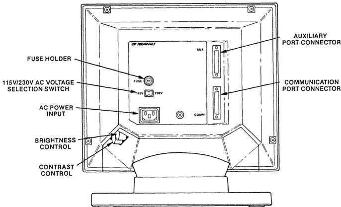
**Figure 2-1. Back View of the Display Unit**
