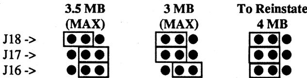
The DCME-Q4B/3.5 MB memory board (Special Revision) has 8 rows of memory chips and may be configured as a 3 MB, 3.5 MB, and 4 MB. Jumpers J5 and J6 are configured the same as the 4 MB. Jumpers J16, J17, J18 are used to strap the DCME-Q4B addressing to 4 MB, 3.5 MB and 3 MB.
