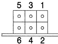
The top row of pins are for connecting external temperature sensor.
