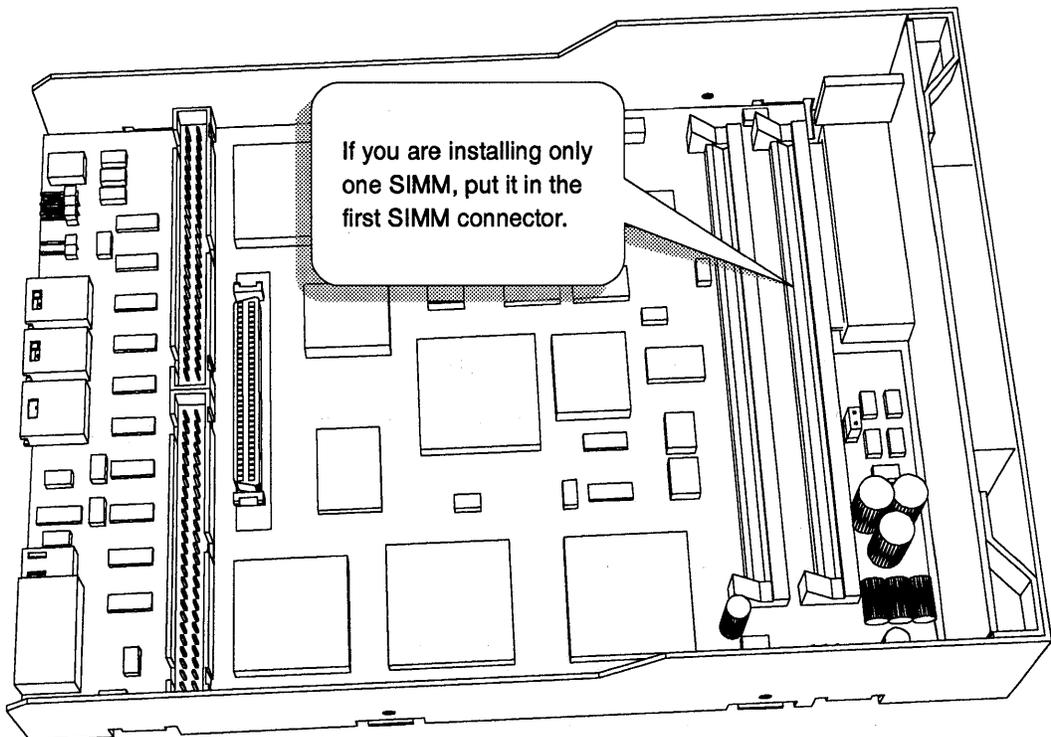
**Figure 1-6: Installing SIMMs**
