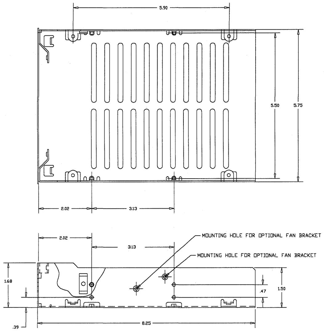
Figure 1-1: Mounting diagram
