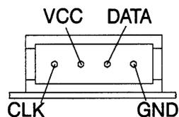
**UART Connector:** This is used to connect an external monitor to the controller. The CRD-5400's monitor utility offers a means to configure the controller, create and manage RAID sets, initiate rebuild operations, and view error logs, among other functions. The following diagram shows the pinout of the UART connector and how the signals should be carried to DB-25 and DB-9 connectors.
