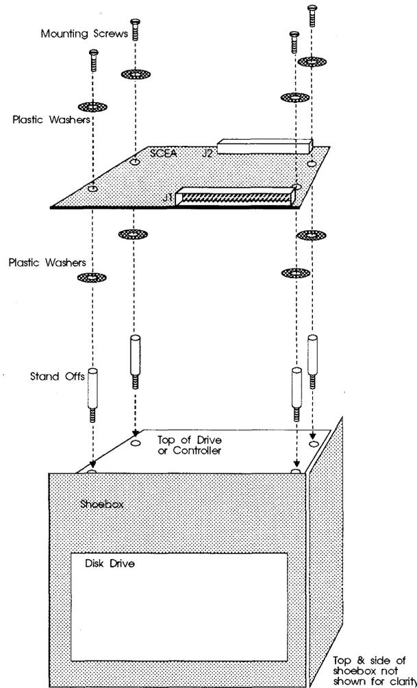
Figure 1: Shoebox installation example
