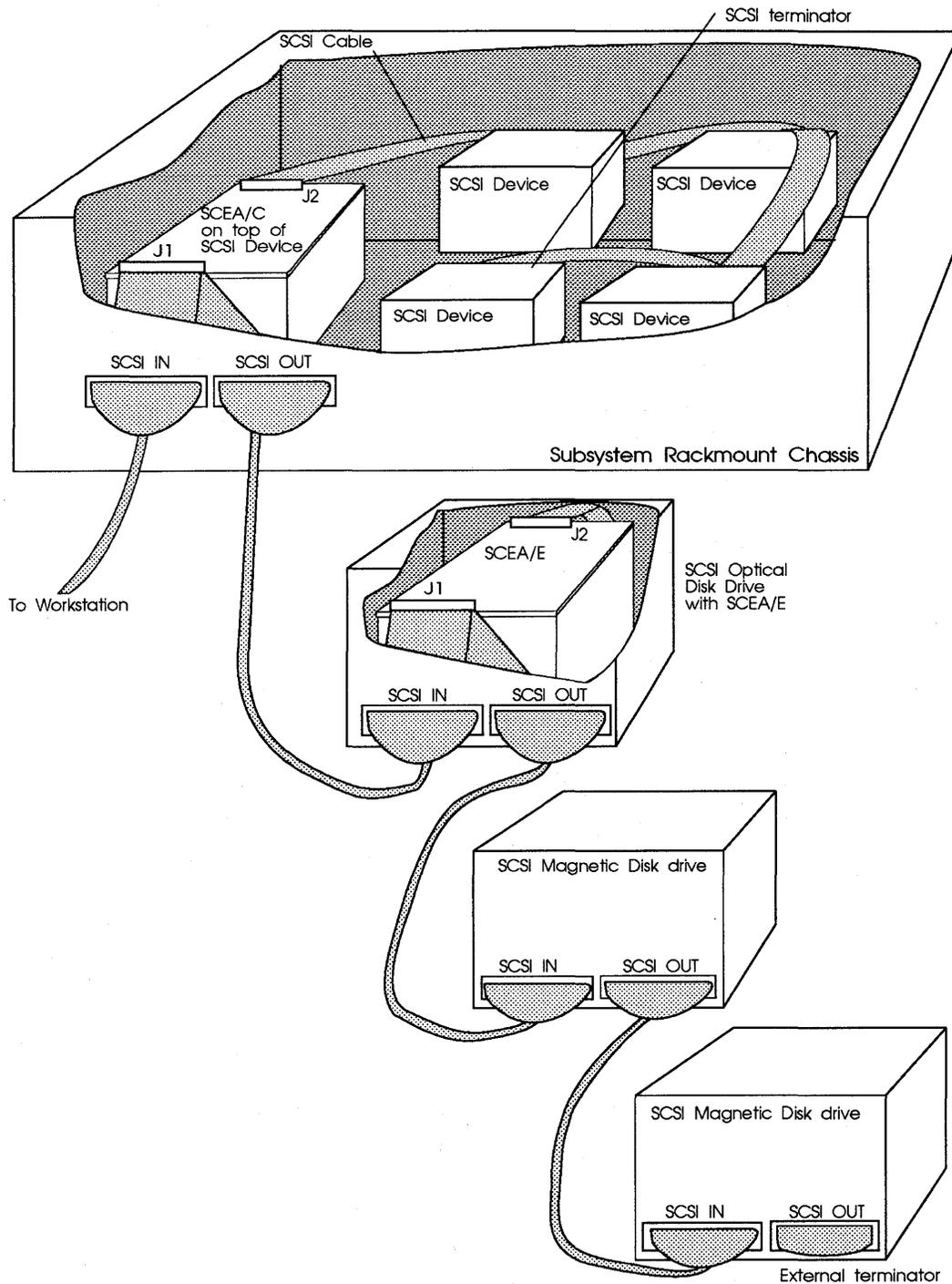
Figure 3-8: Cabling example from inside Subsystem
