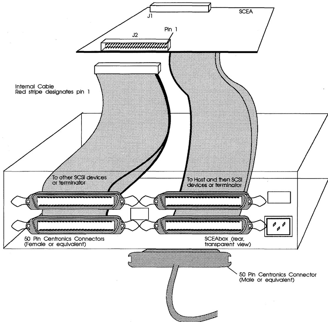
**Figure 3-10: Connecting SCSI cables in the SCEAbox**
