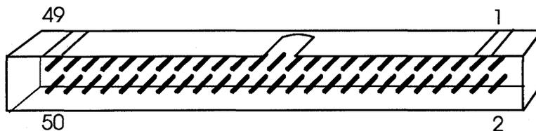
**Figure C-1:** Nonshielded SCSI device connector
