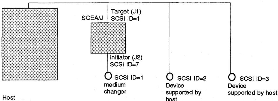
This diagram is for SCSI IDs and LUNs for workstations that do not support LUNs with devices supported by the host.
