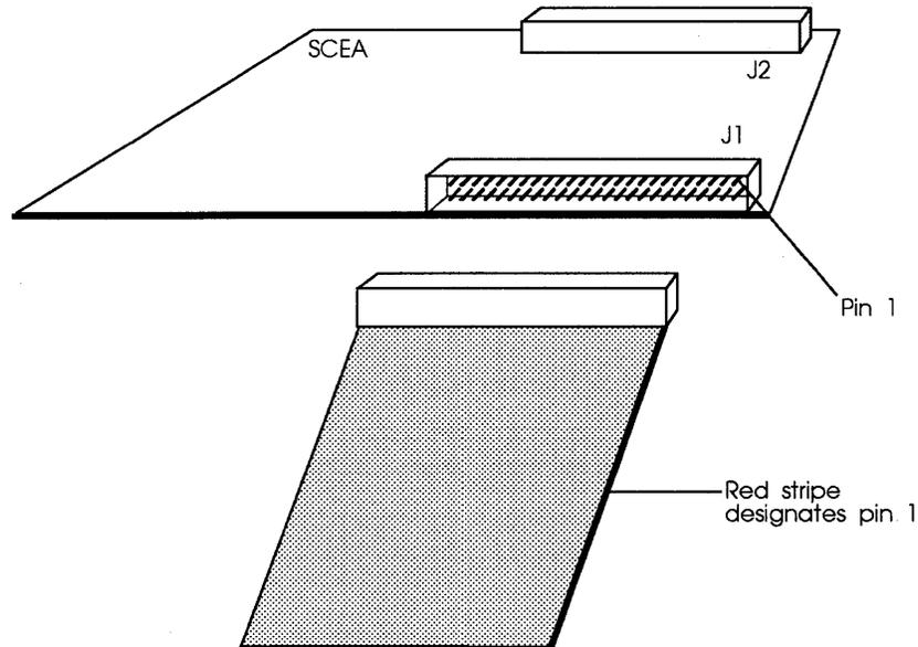
**Figure 3-3: Host SCSI port (J1) cable connection**
