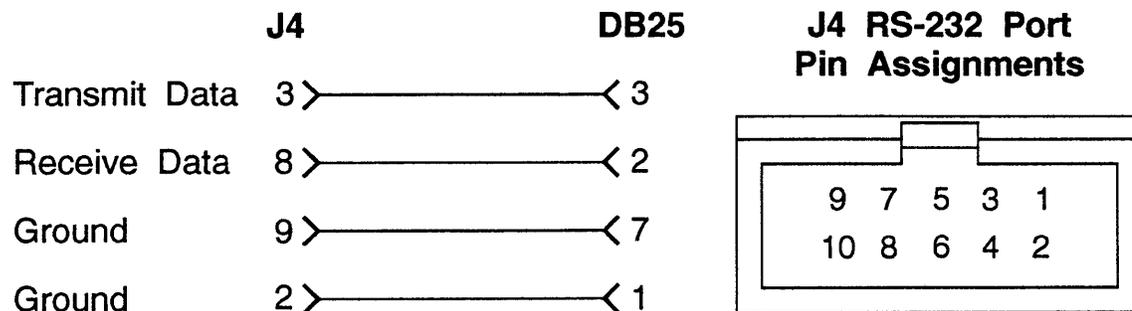
Figure 4-25: RS-232 Cable Pin Out
