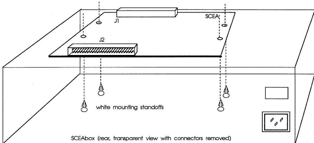
**Figure 3-11: Installing the SCEA into the SCEAbox**
