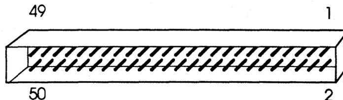
**Figure 5-1: SCSI device non-shielded connector**
