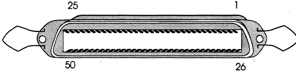
Figure 5-2: SCSI device shielded connector
