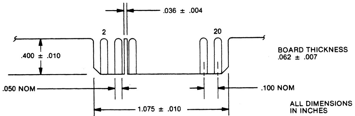
FIGURE 6. CONNECTOR DIMENSIONS
