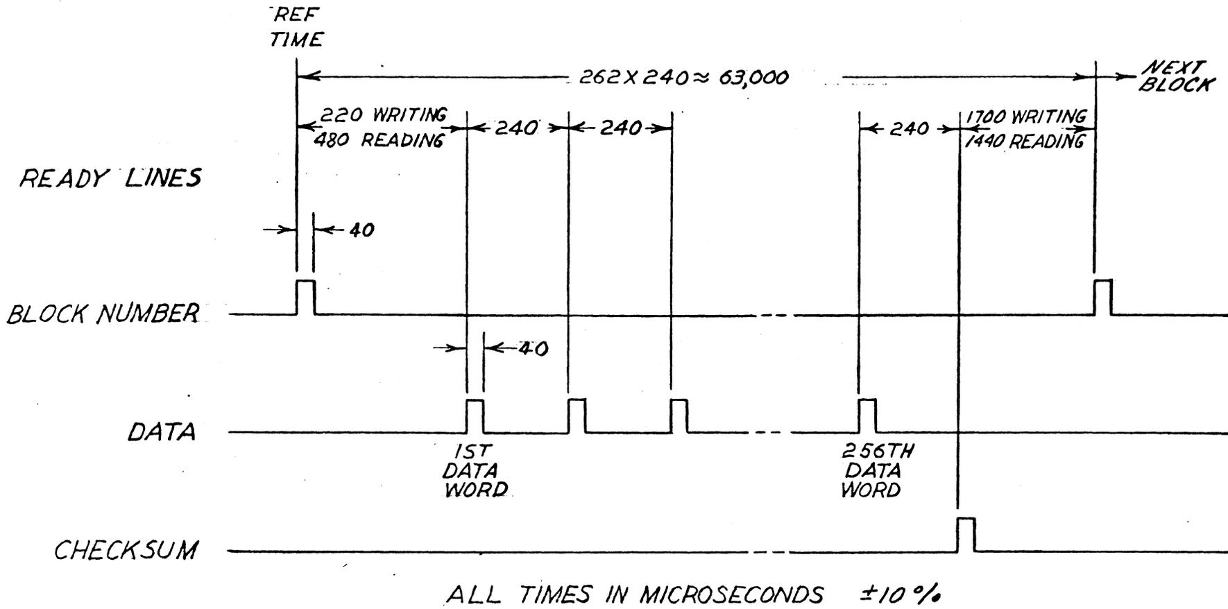
NOTE: THIS TIMING DIAGRAM REPRESENTS POSITIVE TRUE LINES. THE LINCTAPE I/O LINES ARE GROUND TRUE.
