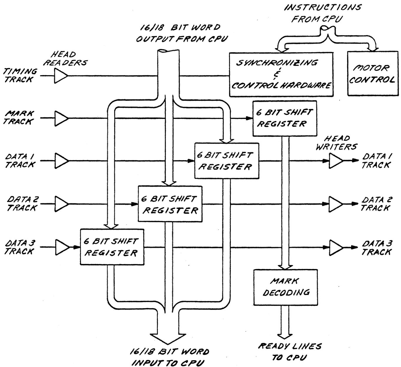
Figure 10.1 Basic LINC Tape Block Diagram
