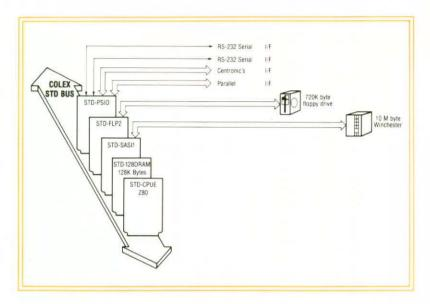
bytes of storage. Additional drives may be connected to the disk controller card for a total of four floppy drives and eight rigid disk drives.
