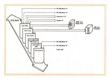
STD BUS – The system uses the STD bus. This allows the basic configuration to be expanded to multiuser operation at much lower cost than other bus concepts. The bus also allows an OEM to interface customized peripherals or additional memory to the system. COLEX is a leader in manufacturing of STD-BUS systems and boards, and offers both 8 and 16 bit STD bus products.
