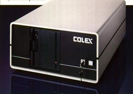
STD-Bus system. If additional system memory is required, add more memory cards; if additional I/O capability is needed, install more I/O cards. Need a CRT controller/keyboard interface? Add that card, too. If the mass storage capabilities of the 820 are outgrown, the simple addition of a 10 M byte rigid disk creates the 850.
