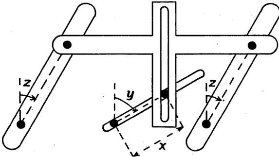
The equation  $\sin z = x \sin y$  may itself be very useful, especially in connection with the law of sines in trigonometry. When one has our previous arrangement, i.e., the one with the link in a groove, we may take the z arm also as a variable and get the equation  $W \sin z = x \sin y$ .
