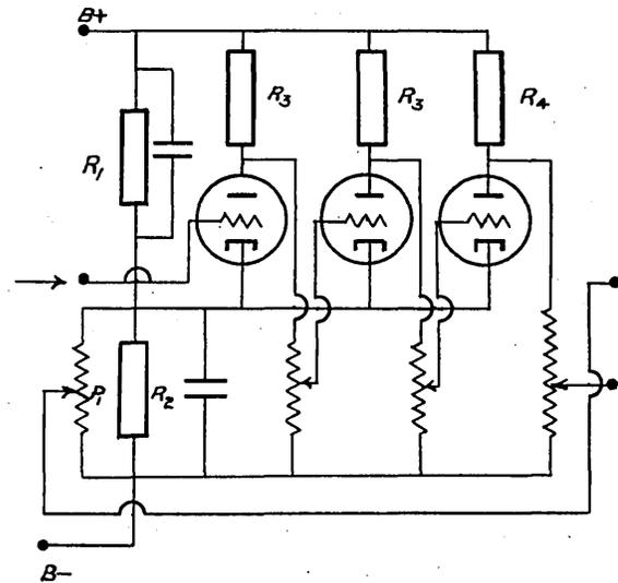
stage should be modified to minimize drift. This will also provide bias relative to ground. Confer the article by Y.P. Yu in *Electronics*, Vol. 19, No. 8 (August 1946), pp. 99-103. Relative to the output, this device is a two-terminal voltage source, whose value depends on the input voltage. The internal resistance can be calculated by considering the evident bridge circuit.
