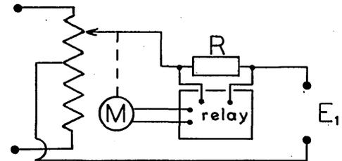
the contact so that the displacement from the center of the scale is proportional to the input voltage. By using the voltage across the potentiometer as another variable, a quotient can be obtained. The center tap on the potentiometer is used to permit the signs of the various quantities to be free.
