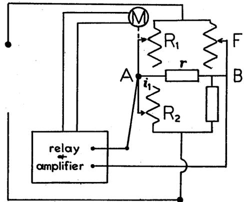
same sign as  $i$ . If  $i$  is positive  $R_1$  is too small and hence should be increased. If  $A B$  is positive, a voltage amplifier and a relay circuit will cause the motor to turn so as to increase  $R$ . On the other hand, if  $i$  is negative  $R_1$  is too large. Since the voltage drop  $A B$  is negative, the relay circuit will cause the motor to turn in the opposite direction and reduce  $R_1$ .
