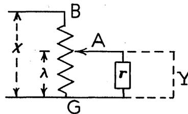
Let  $X$  be the input voltage,  $Y$  the output voltage across the resistance  $r$  (which may be an impedance of a more general character). Let  $P$  be the total resistance in the potentiometer,  $\lambda$  the fraction of  $P$  in parallel with  $R$  from  $A$  to  $G$ . The resistance from  $A$  to  $G$  is that of the two parallel resistances  $\lambda P$  and  $r$ , i.e.,
