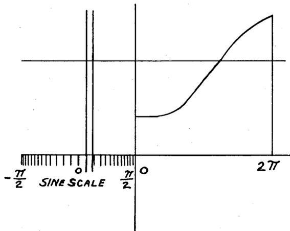
lel to the  $y$ -axis. To set up a rectangle with one pair of sides having the length  $\sin \beta - \sin \alpha$ , we set the wire of one slide on the value  $\alpha$  of the sine scale and the other on the value  $\beta$ . The distance between the wires is then  $\sin \beta - \sin \alpha$ . The  $x$ -axis, the first slide wire and these last two now enclose a rectangle. (This is not the device described by Galle, *loc. cit.*, but the idea is the same.)
