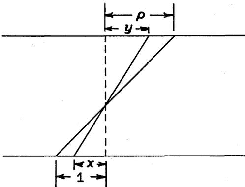
arrangement is analogous to our previous one and that the upper arrangement will be used to position the pivot. Suppose we move the upper bar over the x bar to the unit position and the one over the y bar an amount  $\rho$ . This will determine the position of the common pivot so that  $s_1/s_2 = \rho$ . Hence the output y will have the value  $y = \rho x$  where  $\rho$  and x can be variable.
