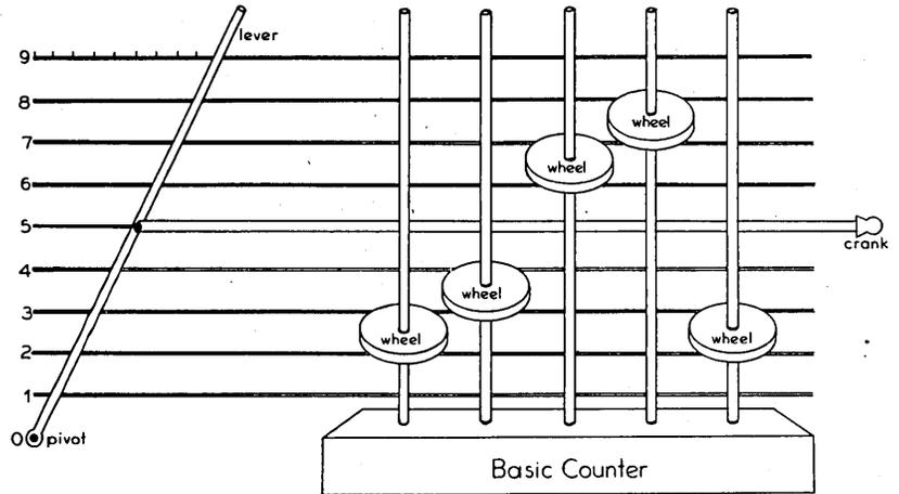
5. All the previous feeds were similar in that a choice of possible motion is made in order to obtain the proper feed. A somewhat different principle is used as the basis of keyboard machines, for instance, the comptometer, an American invention. Here the various feeds are obtained by stopping a motion at different places. To illustrate the principle, we introduce an extremely simplified version of such a feed.
