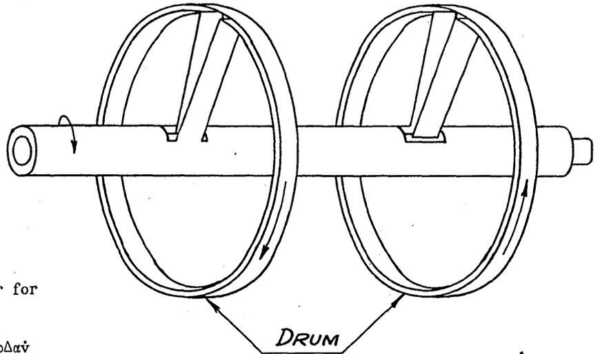
is a set of drum and band for each direction. The control shaft can be considered as a hollow cylinder surrounding the solid driven shaft. The brake bands are mounted on a steel strip of spring-like nature. One end of this strip is connected to a projection from the control shaft, the other end to a projection on the driven shaft, which passes through a slot on the control shaft.
