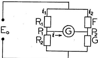
ances. G may be variable but its value is known.  $R_1$  and  $R_2$  are resistances to be compared. Let  $i_1$  denote the current through  $R_1$ ,  $i_2$  through F and  $i$ , the current through the galvanometer, which we suppose flows from  $P_1$  to  $P_2$ . Let E be the applied voltage. The current through  $R_2 = i_1 - i$  and hence
