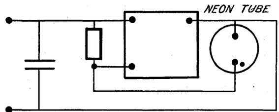
above. Normally the amplifier circuit behaves just like a high resistance. But when the voltage reaches a certain value, the neon tube discharges and the circuit is briefly then a relative short across the condenser.
