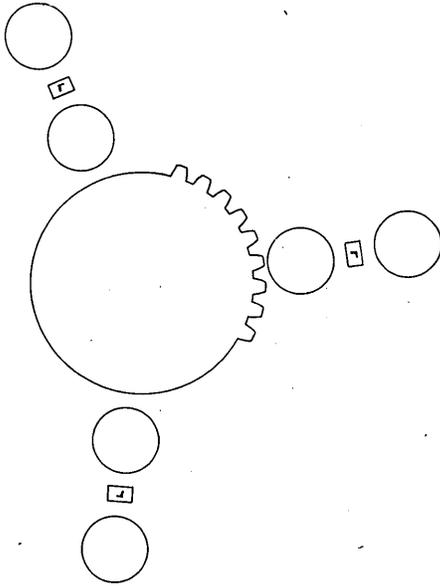
3. Another way in which a feed can be arranged is by means of the Leibnitz wheel. The latter is a cylinder along whose lateral surface teeth of varying length are placed. Associated with this wheel is a smaller gear which meshes with a varying number of teeth, depending upon its position.
