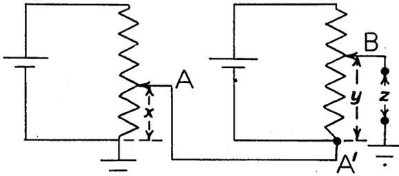
points A and A' are x volts above ground and the point B is y volts above these. Hence, B is  $x + y$  volts above ground. The trouble with this game is that it can be played only once. After one such connection the circuits are no longer independent. However, the batteries can be replaced by the secondary coils of transformers.
