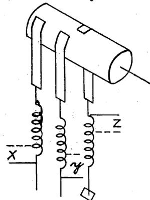
around its axis. On one side of the cylinder, we have two bands. One end of these bands is fastened to the cylinder, the other end to a spring. The band is partly wrapped around the cylinder and extends down vertically to the corresponding spring. Each band and spring corresponds to an input. On the opposite side of the cylinder is a similar arrangement of band and spring for the output.
