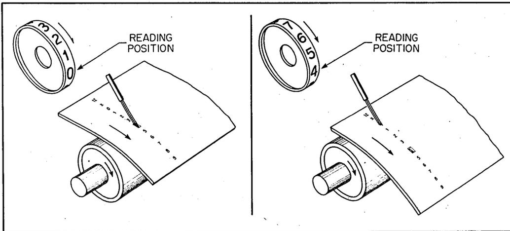
MOVEMENT OF A COUNTER WHEEL IN ADDITION
