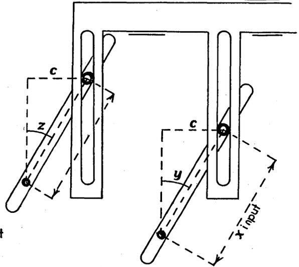
ever the method for putting in the  $x$  input is not indicated. The  $y$  input and the output  $z$  are angles. The cross piece is constrained to move parallel to itself. The  $x$  input is a length. The cross piece causes the two triangles pictured to have a common side  $c$ . For this common side we have  $c = \sin z$ ,  $c = x \sin y$ , or  $\sin z = x \sin y$  which is approximately  $z = xy$ .
