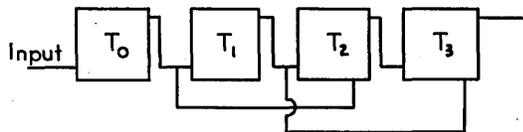
to (1,1,0,0) in response to the first three pulses. As above the effect of the next pulse is to send it to the (0,1,1,0) stage, i.e., the counter passes from 3 to 6 skipping two states. The next state is (1,1,1,0) or 7. The next pulse, at first, clears the system to (0,0,0,1). However, there is also a feedback from the last stage so the circuit goes to (0,0,1,1) or 12. [One would also expect that when  $T_2$  turns to 1 from 0 in this process,
