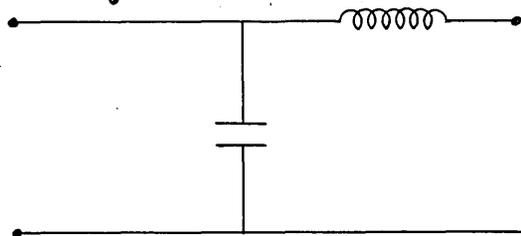
which  $1/Cw \ll wL$ . For the condenser offers a path with impedance  $1/Cw$  for these frequencies, while the impedance of the other path contains the term  $wL$ . (There is a case where this won't work. The reader is urged to consider the possibilities for the output impedance.)
