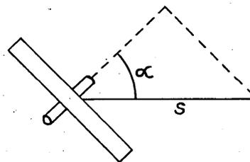
makes an angle  $\alpha$  with the axle of the wheel. During this displacement the axle remains parallel to its original position. The component of the displacement parallel to the axle will induce no rotation, while if the wheel turns freely, there will be no slipping perpendicular to the axle. Consequently, the wheel will turn through an angle  $\phi$  such that  $r\phi = s \sin \alpha$ .
