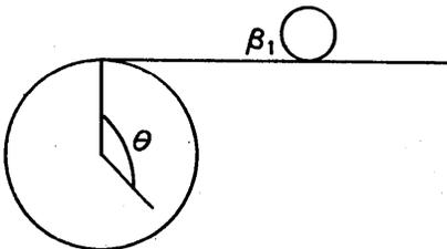
Let us consider such a tape on a spool whose angle of rotation we will call  $\theta$ . The length of the tape can be measured by causing it to turn a cylinder an amount  $\beta$ . If  $r$  is the radius of the cylinder  $r d\beta = \rho d\theta$ . We see that if  $d$  is the thickness of the tape,  $\frac{\Delta\theta}{2\pi}$  is the number of revolutions for a change  $\Delta\theta$  and  $\Delta\rho = d \frac{\Delta\theta}{2\pi}$ . Thus we may assume  $d\beta = k\theta d\theta$ .
