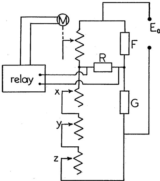
If  $R_0$  is the value chosen as unit resistance, the maximum resistance for  $x$  should be  $3R_0$ , that for  $y$  and  $z$   $2R_0$  and for  $w$ ,  $7R_0$ . This illustrates the convenience of logarithms when one has to deal with greatly varying quantities. However, this has its difficulties too as we shall see.
