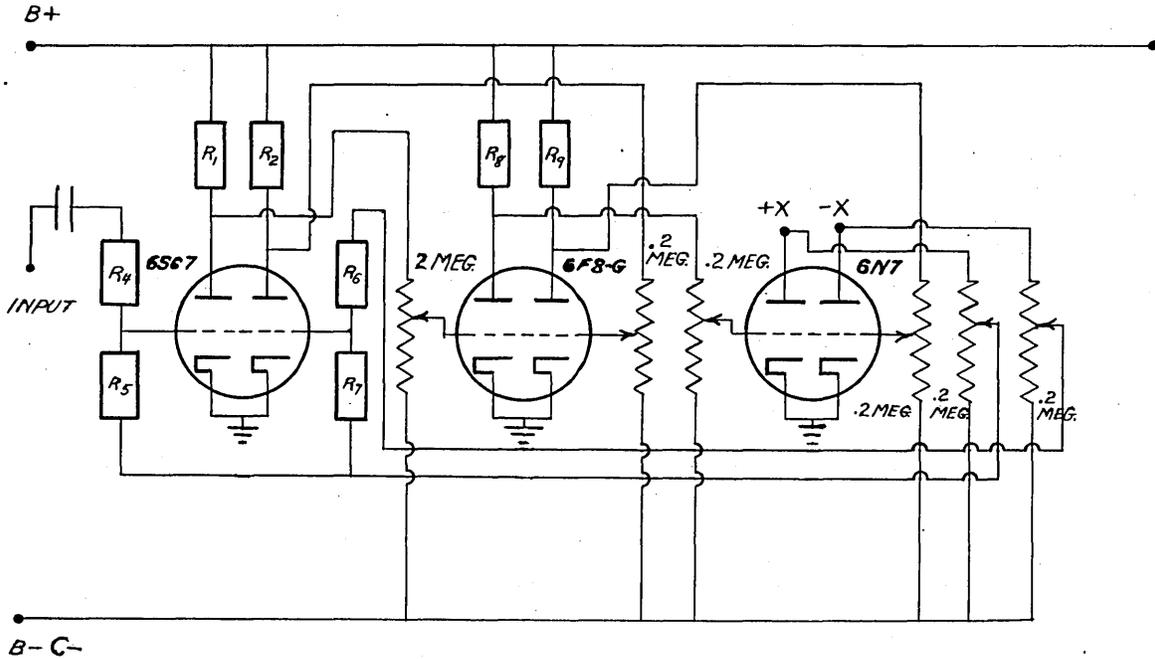
However, in using this power box in the general schematic shown on page III - 18, B+ replaces ground in the coefficient boxes and blocking condensers should be inserted at  $\epsilon_1$  and  $\epsilon_2$ . The input to the power box is taken from a potentiometer which determines the absolute value of  $x$ . These potentiometers in turn can be powered by an oscillator tuned to some frequency which should in general not be a harmonic or subharmonic of the power supply a.c. frequency.
