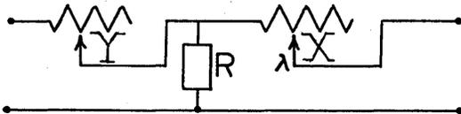
Here  $x$  and  $y$  are variable resistors connected so that  $x = R/\lambda - 2R$  and  $y = R\lambda$ . It is readily seen that for every value of  $\lambda < \frac{1}{2}$ , the total resist-
