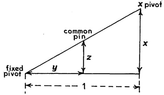
There is another kind of multiplier which while it is only approximate and is limited in range has been very often used because of its simple positive action. This is what is frequently referred to as the "links multiplier." The principle can be understood from the following diagram, where how-
