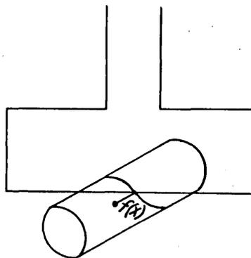
This linear displacement is the linear input of a simple disk integrator. This consists of a disk which rotates an amount  $x$  and an integrating wheel on it which is displaced from the center an amount equal to the linear input.
