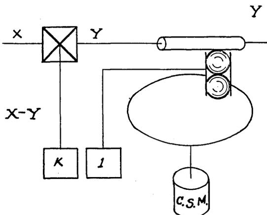
mechanical equivalent of a condenser circuit. The output  $X - Y$  of the differential is applied through gearing to the rate input of the ball cage variable speed so that the equation
