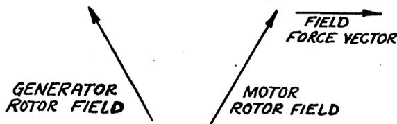
is in the direction tending to bring  $H_m$  and  $H_s$  in coincidence and its size is proportional to the sine of the angle between them. The generator rotor has precisely the opposite torque exerted on it but presumably the input determines its position. Note however that this means that the input must do work if there is any load on the output.
