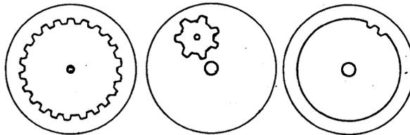
The alternate method for tens transmission in a counter is to gear each dial or cylinder directly to the next by a gear ratio of ten to one. This method has the greatest accuracy, there is no chance for a failure to transmit the one to be carried, and this is, of course, the reason why it is preferred by the public utility corporations in gas and electric meters. Such a gear ratio is indicated in the following diagram. Here we look down on such an arrangement of gears and dials.
