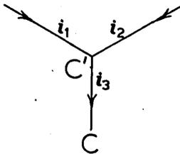
Kirchhoff's Law states that the sum of the currents flowing to a junction point is zero. Here C was the original junction point, C' is the new one added to obtain the addition. At C', we have  $i_1 + i_2 - i_3 = 0$ .
