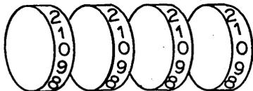
Each cylinder is wheel-like with a broad rim. The interior of the rim on the side next to the lower decimal place is fully toothed; that on the other side is partly toothed. There is an idler gear on a fixed partition between these. When a
