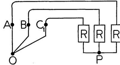
that each of the points A, B, C, etc., is connected through a large resistance of value R to a point P. Suppose that P has a potential  $w$  relative to the origin O. Let  $i_1, i_2, i_3$ , etc., denote the current flowing from A, B, C, etc., to P. Then
