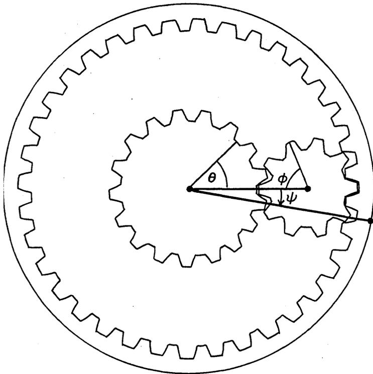
rotation of the outer gear, we have  $y = z - \psi$  or  $\psi = z - y$ . Substituting for  $\psi$  and  $\theta$  in the equation  $\psi = 2\theta$ , we obtain  $3z = 2x + y$ .
