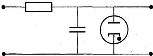
condenser will slowly charge until the breakdown potential is reached, then it will discharge. Unfortunately, the current will continue even with a much lower voltage unless the plate is made negative with respect to the cathode. (This assumes that the cathode is emitting electrons.) This can be accomplished by introducing a resistance and a capacity in the cathode circuit. Thus in this cir-
