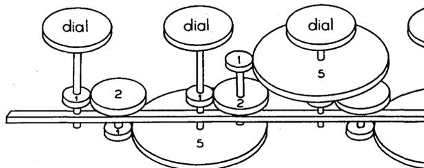
Each relative unit shaft is geared to an idler shaft in a 1 to 2 ratio and the idler shaft is geared to the relative ten shaft in a 1 to 5 ratio.
