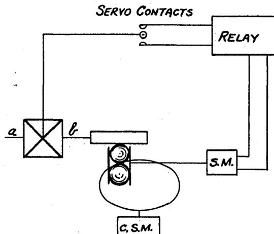
will not work. Here  $a$  is the shaft whose rate of rotation is to be measured,  $b$  is the shaft whose output is to match the other. The output of the differential is the difference of the shafts  $a$  and  $b$ . The servo contact arrangement is such that when  $a-b$  is positive, the servo motor tends to increase  $b$  ( $= \frac{db}{dt}$ ) and conversely when  $a-b$  is negative, the arrangement tends to decrease  $b$ .
