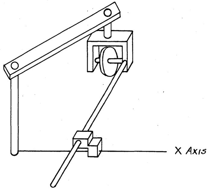
ing perpendicular to the axle of the wheel. In turn this rod slips freely through a collar which is rigidly attached to another collar which slides along a rod parallel to the x-axis. Since the two collars are mutually perpendicular, the rod extension of the yoke is always perpendicular to the x axis and the wheel axle is always parallel to the x axis.
