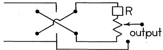
cisely the resistance of the potentiometer  $P$ . This has the effect of "folding the scale." The potentiometer has now two scales, one for the right-hand position of the switch, the other for the left-hand. The scale would look like this if the total deflection was  $180^\circ$  and
