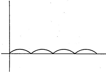
that in the full wave rectifier the  $\frac{1}{2} \sin \omega t$  term has disappeared. It is characteristic of full wave rectifiers that the odd harmonics disappear. In order to minimize the effect of the harmonics, the output of the rectifier is sent through a filter. A typical circuit is shown below. The inductances
