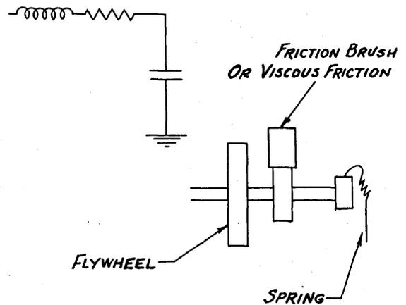
The second combination of flywheel, viscous friction drag and spring is analogous to the electric circuit if we assume that the total charge passing
