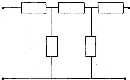
with the shorting circuits having a high impedance for the desired frequency and the series circuits having low impedance. It is clear that this shunts the undesired frequencies through the shorting circuits, while the low impedance of the series circuits favors the desired frequency.
