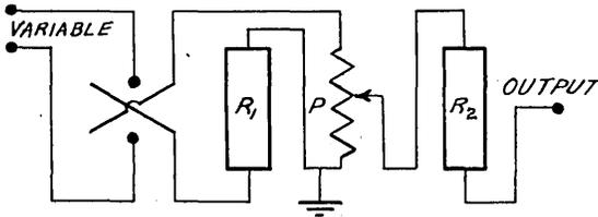
The double pole double throw switch is set according to the sign of  $a_{1,j}$ . The potentiometer  $P$  is 10,000 ohm wire wound and  $R_1$  is a resistance matched to  $P$ .  $R_2$  is .5 megohm and must be matched with the  $R_2$ s of the other coefficient boxes. This can be easily done by taking twice as many .25 megohm resistors evaluating each and then combining them in pairs with the proper total resistance.
