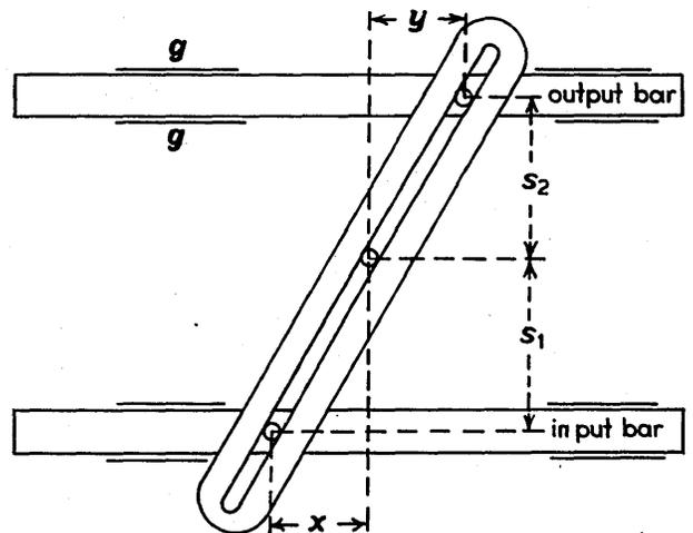
and output displacements apply to bars which are constrained to move parallel to each other, for instance, in grooves or guides. On each bar, we have a pin which fits in a slot in a cross-bar. We also have a pivot in the slot which may be fixed in any position along a line perpendicular to the two parallel bars. When the position of the pivot is determined and one of the parallel bars is moved the other is displaced a proportional amount. For by congruent triangles
