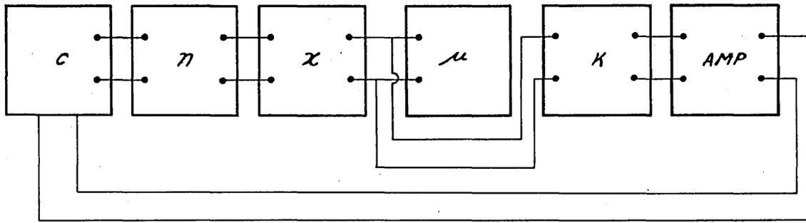
arranged in the case in which the  $x$  boxes are power amplifying circuits. The input signal for each box can be arranged with a current from  $C$ , whose value will be determined so as to maintain  $K$  constant, across a potentiometer whose contact position will correspond to the direction number
