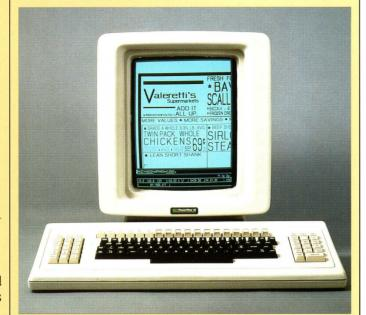
system from any workstation, and the MCS 100 can perform most functions faster than any other input system in the MCS product line. This system's 100-foot cables allow you to position your terminals as much as 200 feet apart. And your operators can access two Previews and two online typesetters.
