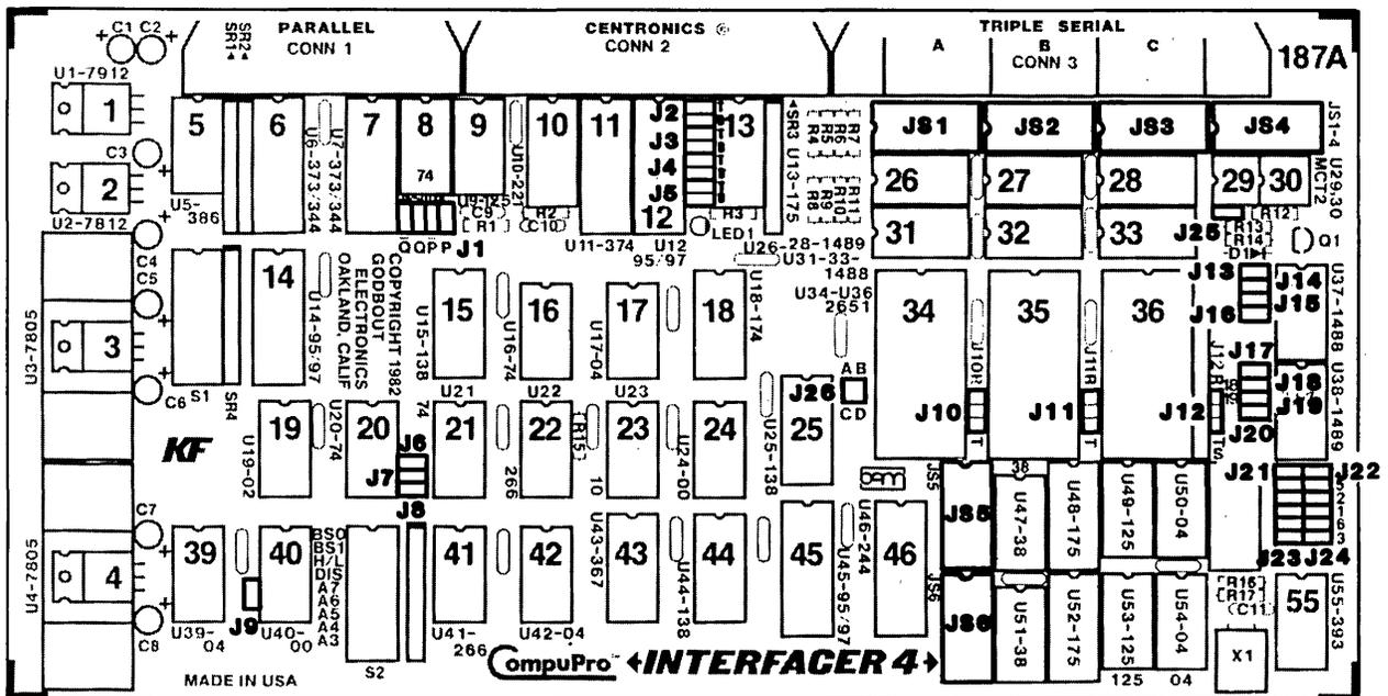
NOTE: Under MP/M 8-16 or an interrupt driven mode, J26 MUST be jumpered A-B and C-D.
