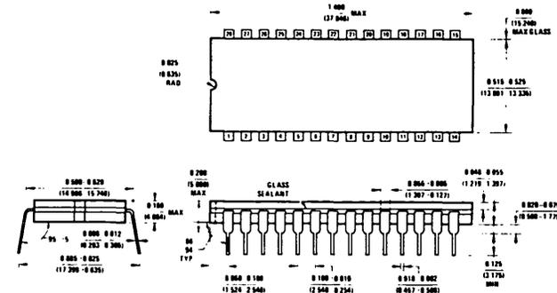
28-Lead Ceramic Dual-In-Line Package (Car Dip [J])
