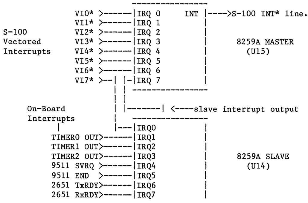
If you wish to "scramble-wire" the interrupts, all interrupt sources and destinations appear at jumpers J7 and J8. They may be jumpered in any conceivable configuration by using dip-headers. The interrupts appear at these jumpers as shown in the following diagrams:
