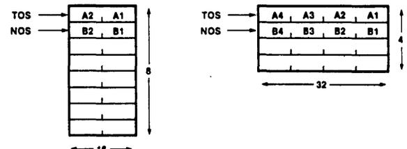
Data are written onto the stack, eight bits at a time, in the order shown (A1, A2, A3, . . .). Data are removed from the stack in reverse byte order (A4, A3, A2 . . .). Data should be entered onto the stack in multiples of the number of bytes appropriate to the chosen data format.
