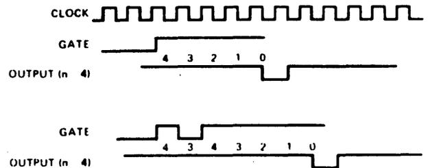
Figure 5. 8253 Timing Diagrams
