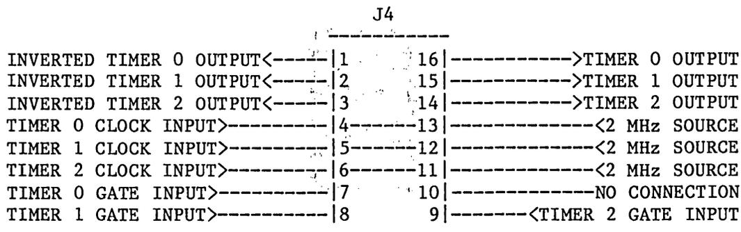
NOTES: All gate inputs are pulled up with a 4.7K ohm resistor. Pins 4 and 13 are connected together, pins 5 and 12 are connected together and pins 6 and 11 are connected together. All timer outputs are buffered.
