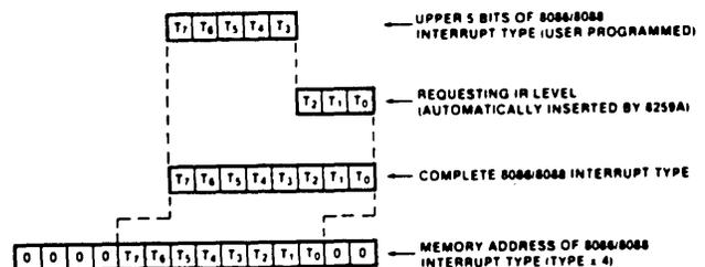
Figure 22. Establishing Memory Address of 8086/8088 Interrupt Type
