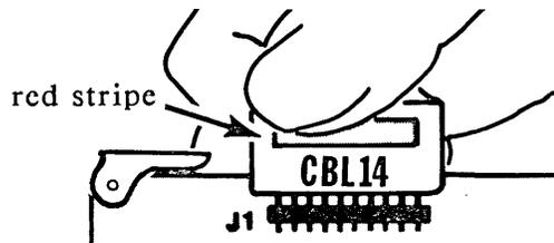
a) Pick up the female connector, of CBL14. Keep the red stripe on the cable to the left.
