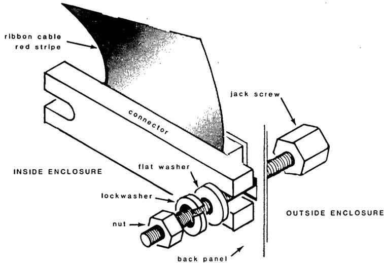
b) Attach connector to back panel with the hardware that came with the system. (Nut/lockwasher inside and jack screw/flat washer outside the enclosure.)
