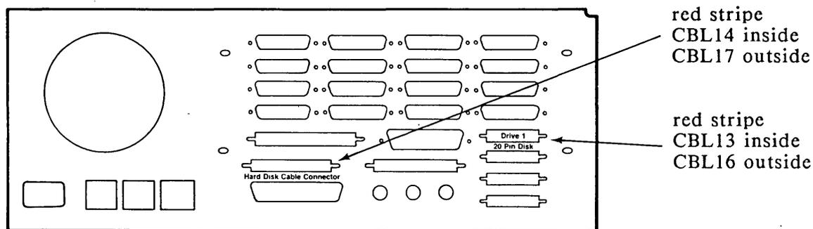
Figure 3. COMPUTER ENCLOSURE - (back panel outside)
