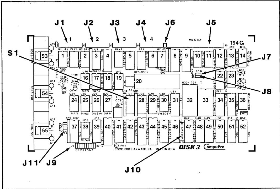
Figure 2. DISK 3 (jumper and switch location)
