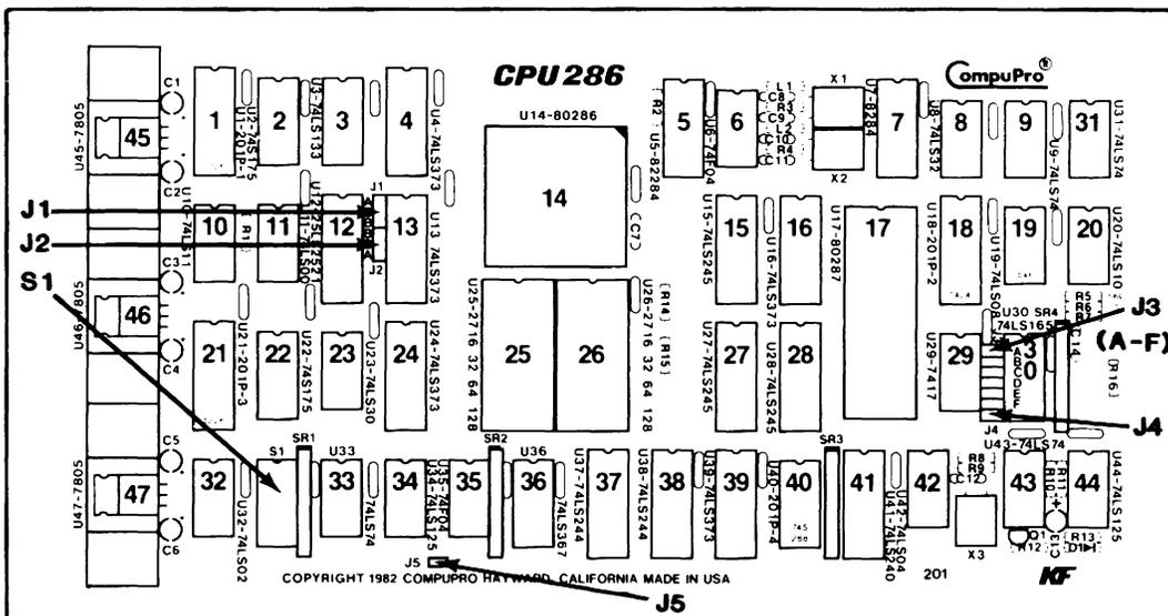
Figure 2. CPU 286 (jumper and switch location)
