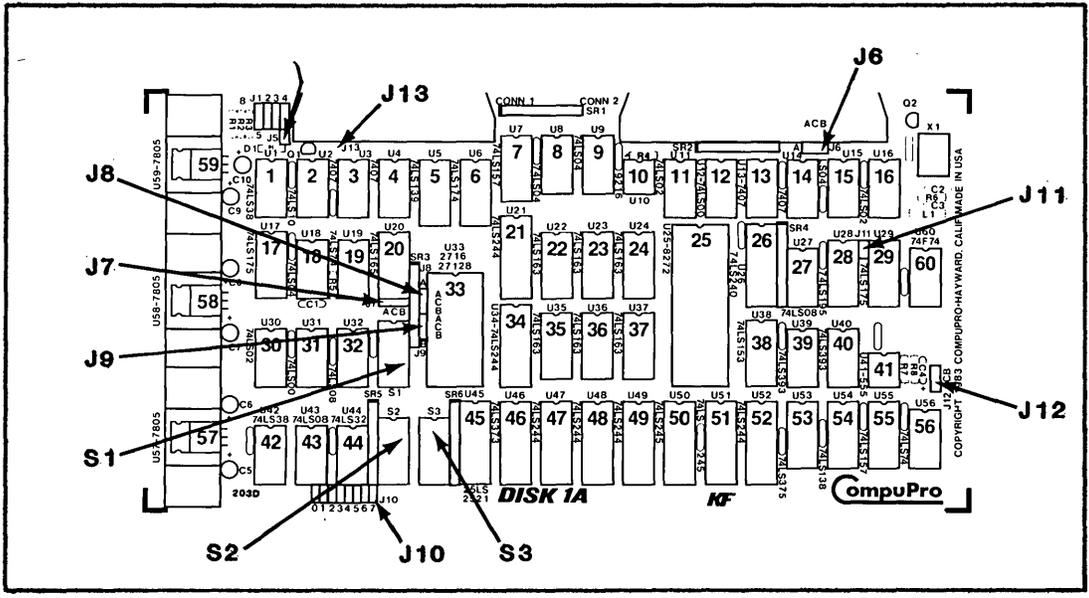
Figure 2. DISK 1A (jumper and switch location)
