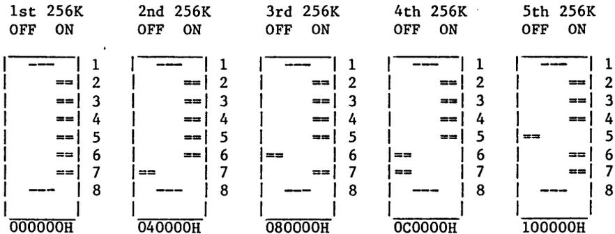
NOTE: This board does not allow any of the four 64K blocks on the board to be disabled.
