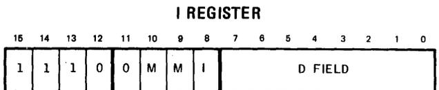
Loads the contents of the effective byte into the lower half of the X Register. The upper half of the X Register is set to zeros:
