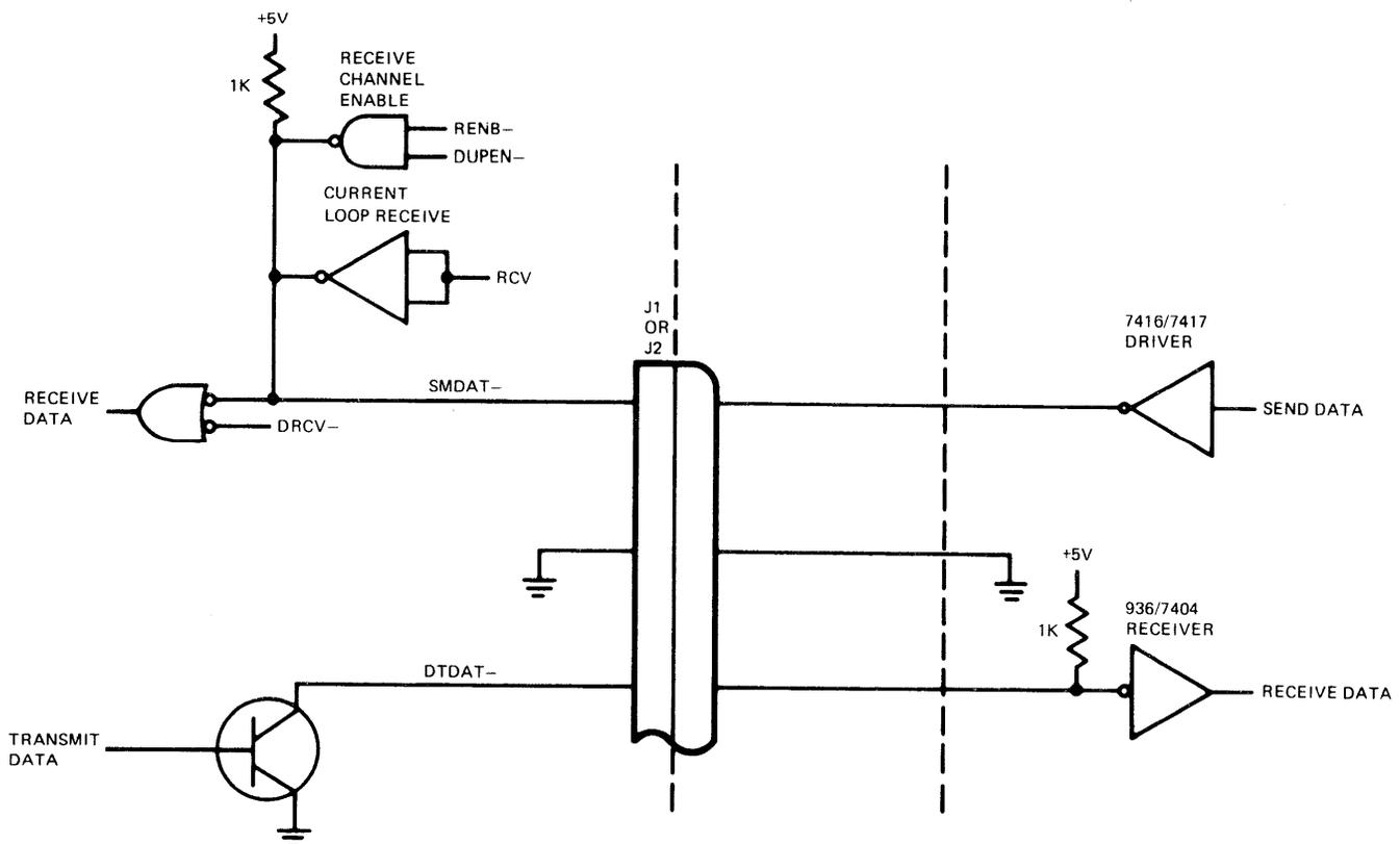
Figure 11-5. TTL/DTL Interface
