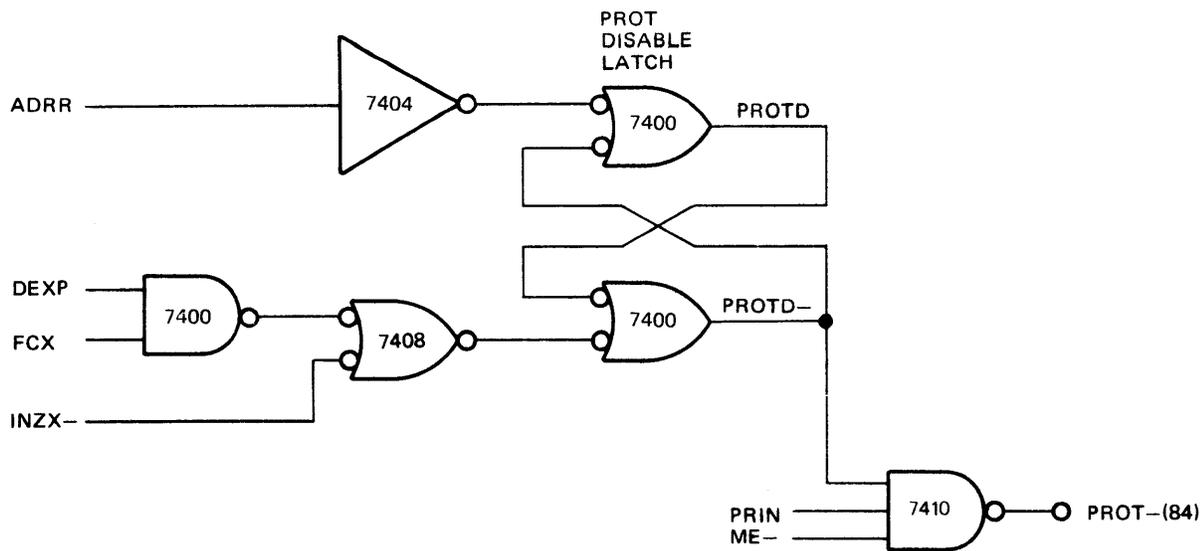
Figure 5-9. Reentrant Interrupt Implementation
