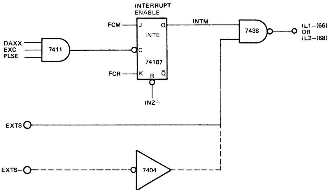
Figure 5-10. Simple IL1-/IL2- Interrupt Structure
