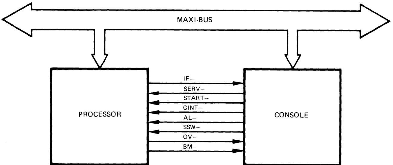
Figure 9-1. Processor/Console Interface
