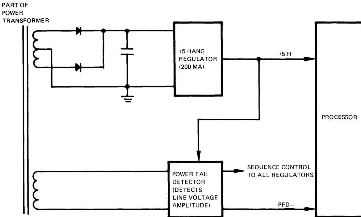
Figure 10-1. Power Monitor Block Diagram.
