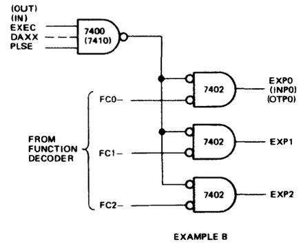
Figure 5-3. Select, Input or Output Command Decode Configurations
