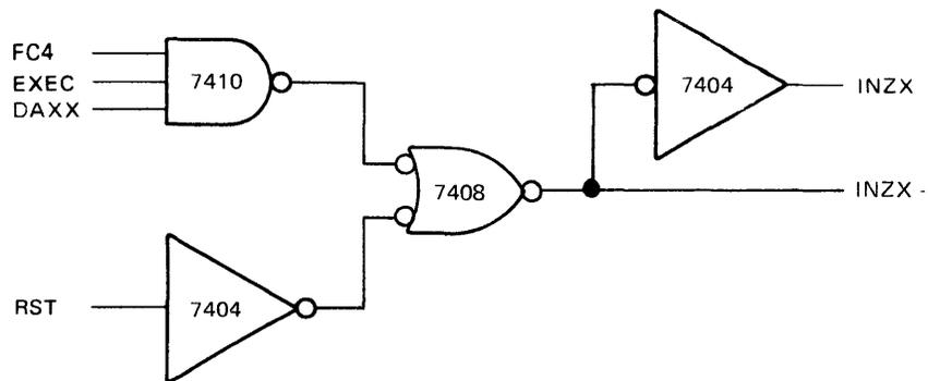
Figure 5-4. Initialization Circuit
