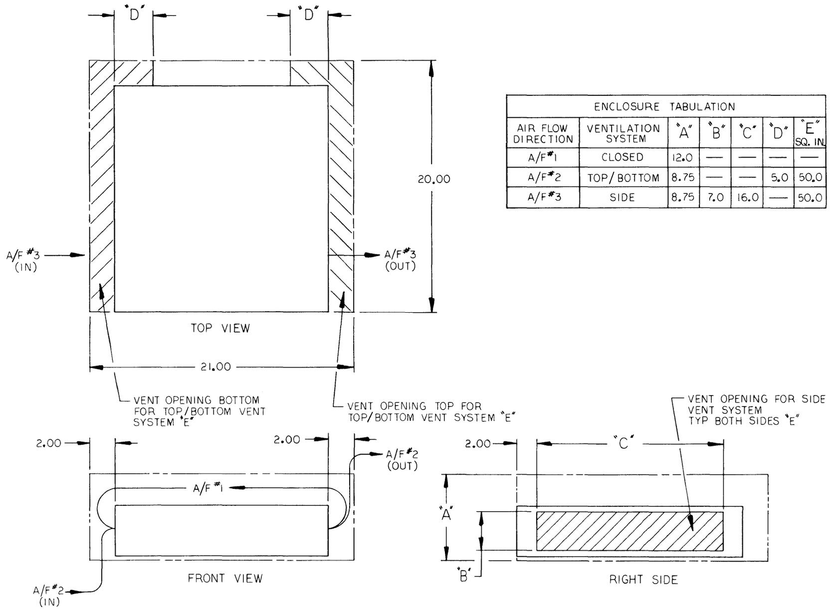
Figure 8-2 ALPHA LSI Ventilation Systems
