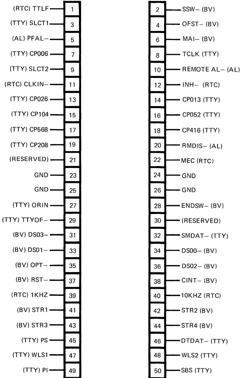
Figure 11-1. Option Card Connector J1 Pin Assignments
