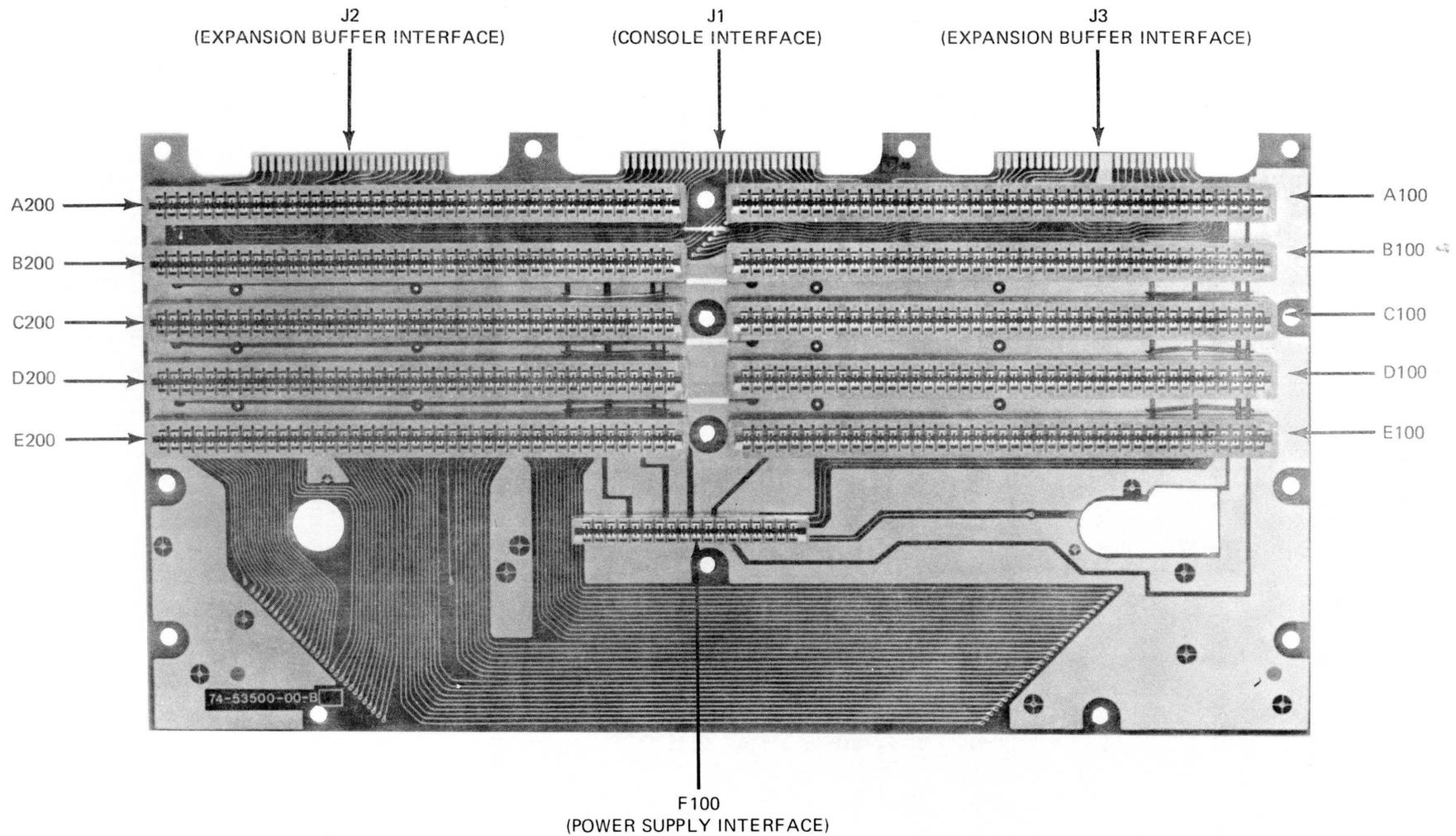
Figure 2-2. ALPHA LSI Motherboard Slot Organization (Rear View)
