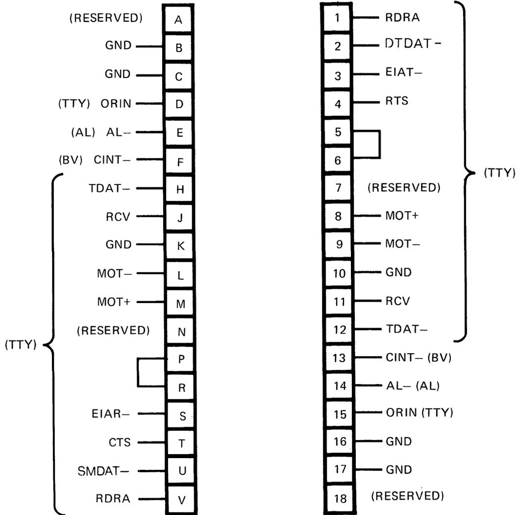
Figure 11-2. Option Card Connector J2 Pin Assignments
