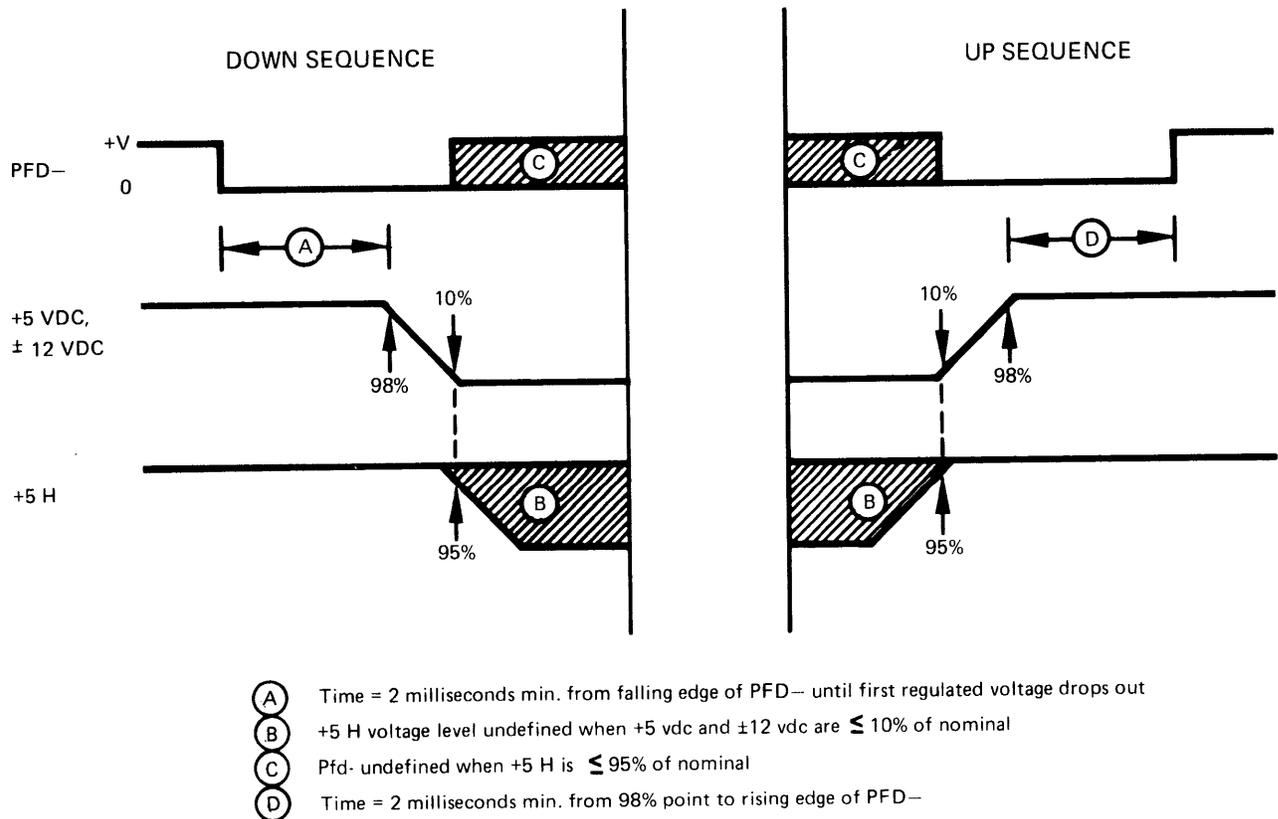
Figure 10-2. Power Monitor Timing Requirements.
