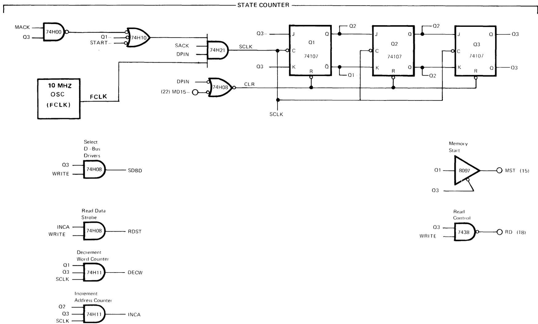
Figure 6-7. State Counter and Decoder
