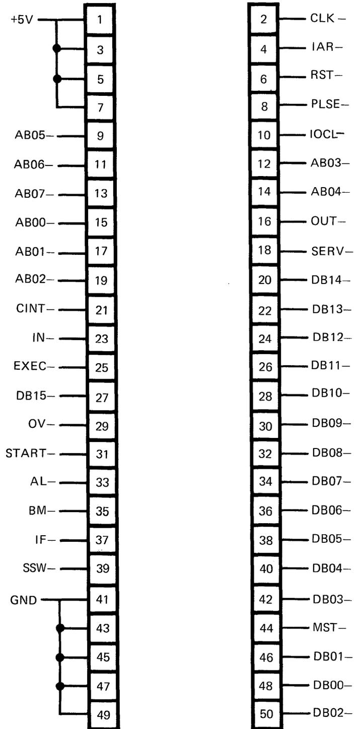
Figure 9-7. Motherboard/ Console Connector (J1) Pin Assignments
