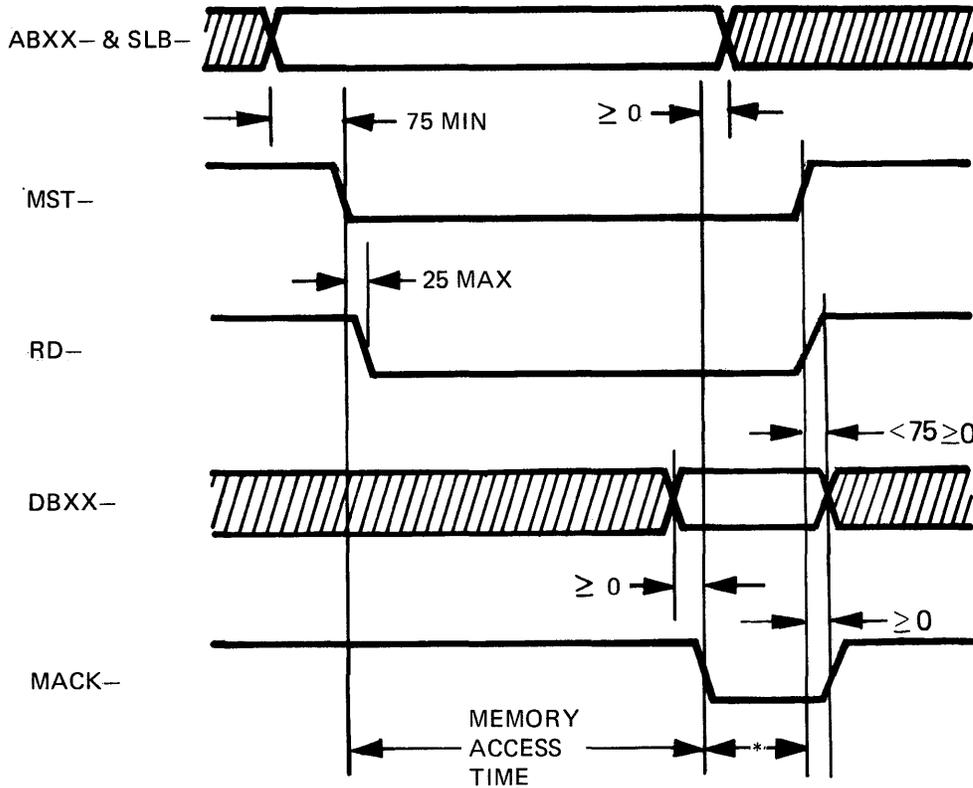
\* INTERVAL DETERMINED BY CONTROLLER TO ACCEPT MEMORY DATA
