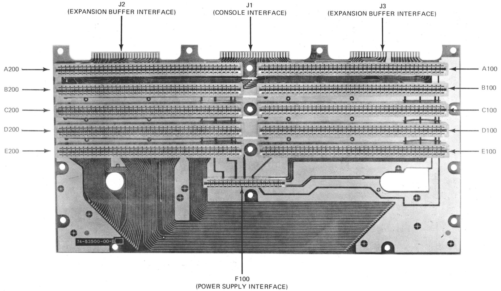
Figure 8-11. ALPHA LSI Motherboard Slot Organization (Rear View)
