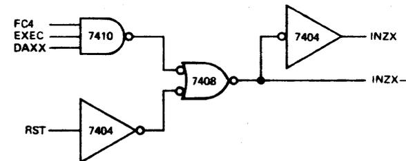
Figure 9-3. Initialization Circuit
