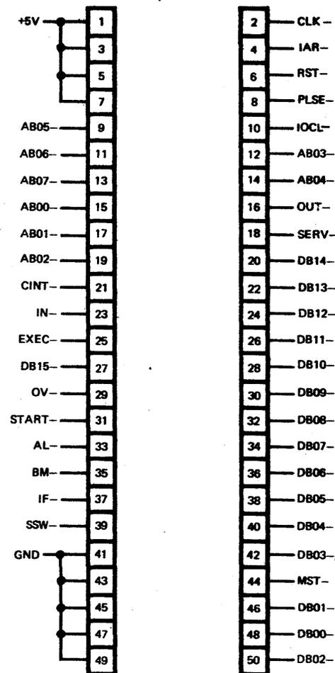
Figure 10-7. Motherboard/Console Connector (J1) Pin Assignments
