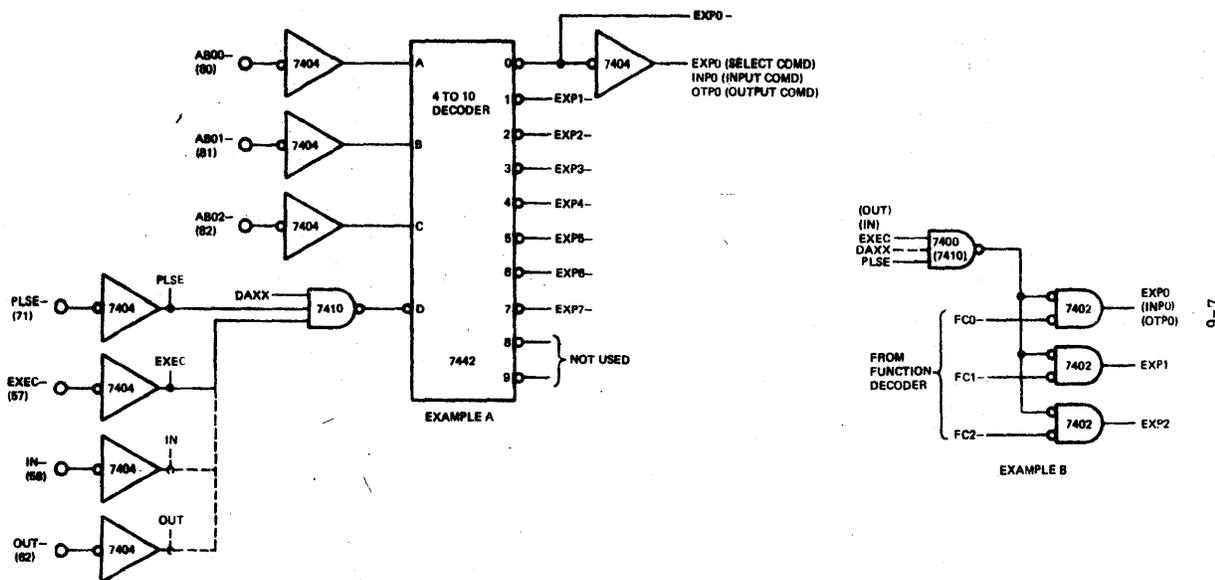
Figure 9-4. Select, Input, or Output Instruction Decode Configurations
