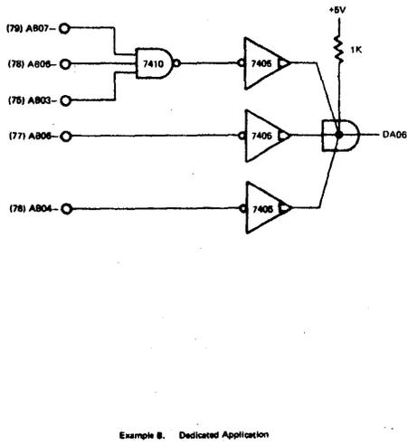
Figure 9-1. Device Address Decoding Techniques
