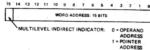
Figure 1-7. Indirect Address Pointer Format
