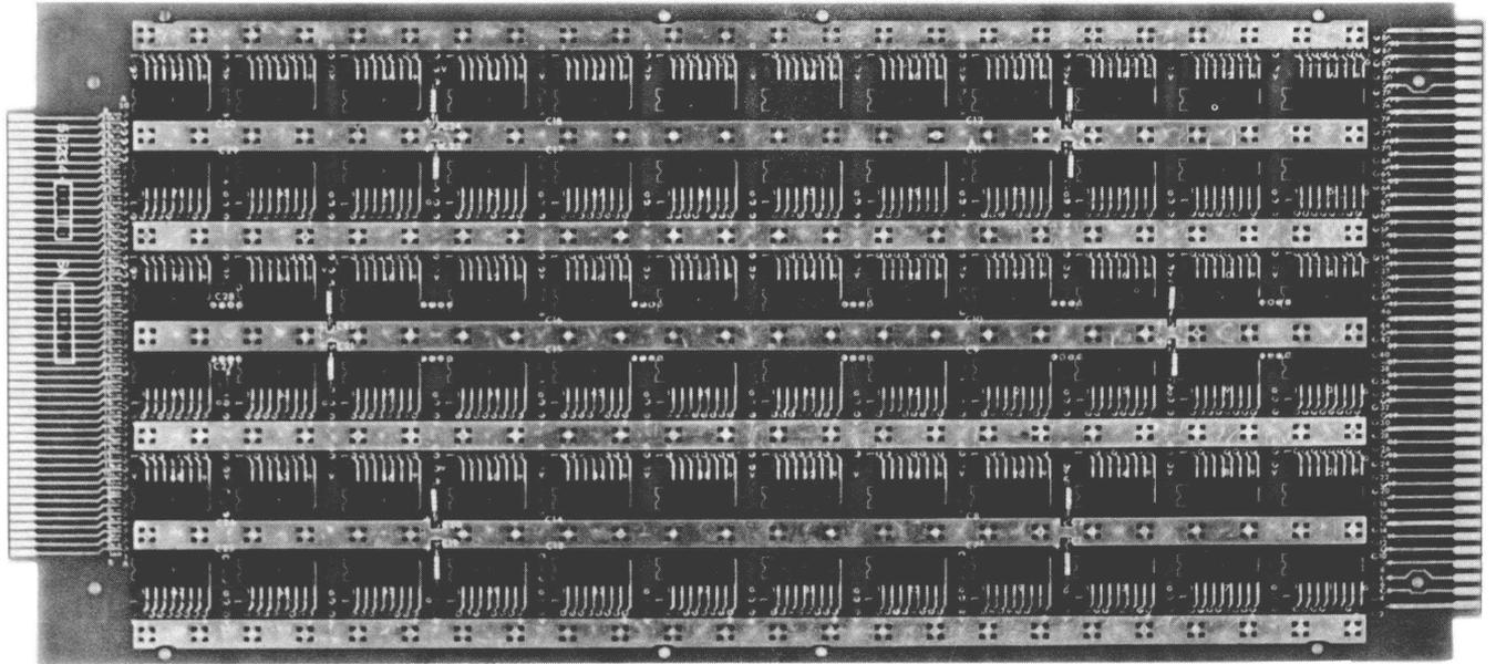
Figure 12-4. Wire-Wrap Breadboard PC Board
