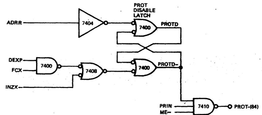
Figure 9-8. Reentrant Interrupt Implementation
