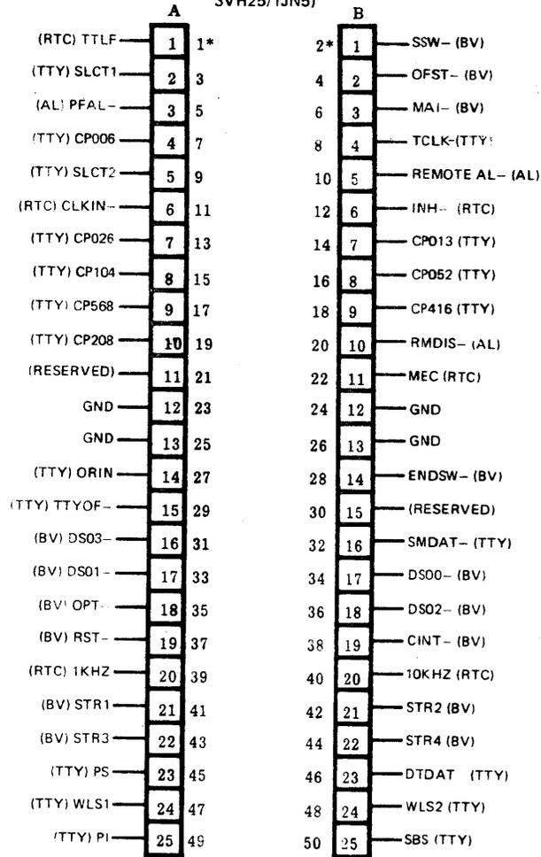
\*Pin numbering system if type 2VH25/1JN5 connector installed.
