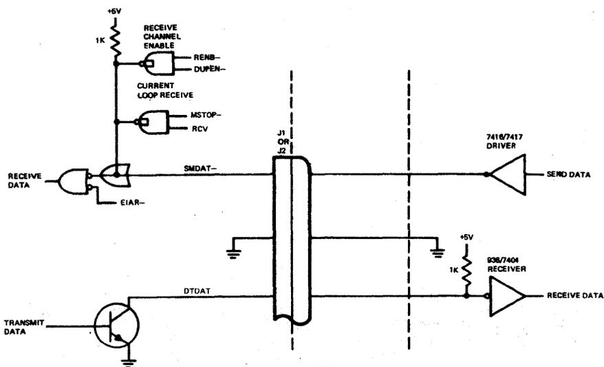
Figure 6-6. TTL/DTL Interface
