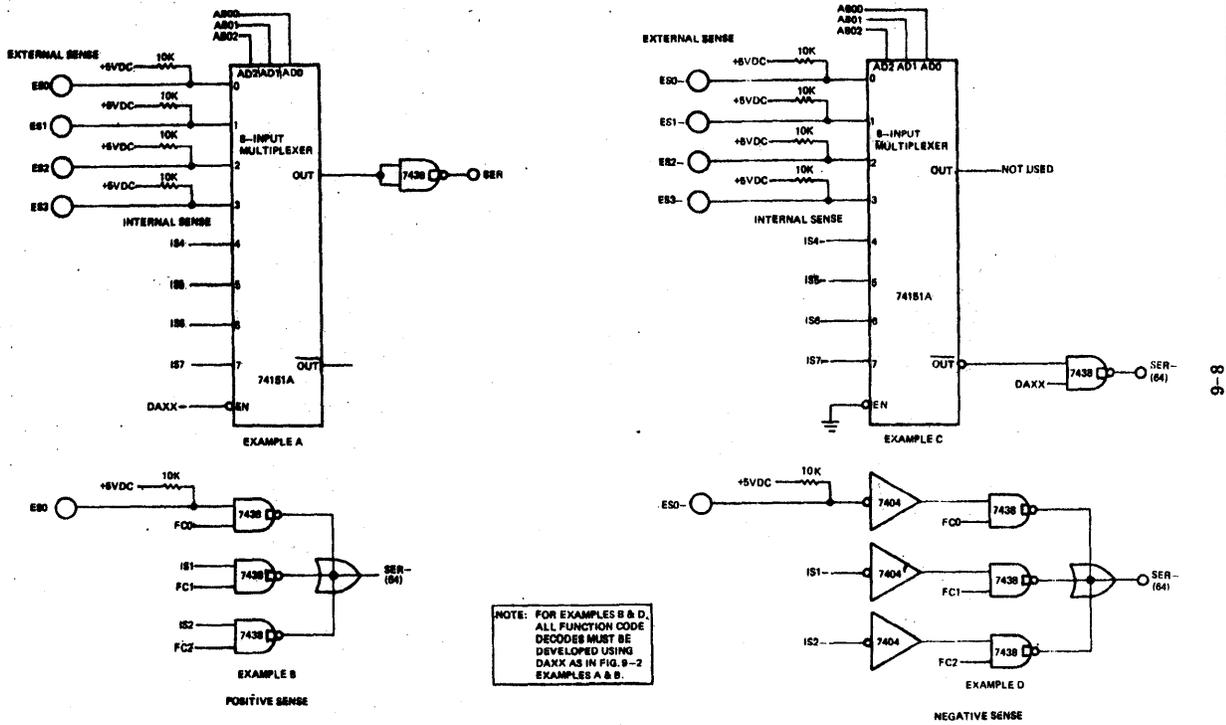
Figure 9-5. Positive and Negative Sense, Circuit Configurations
