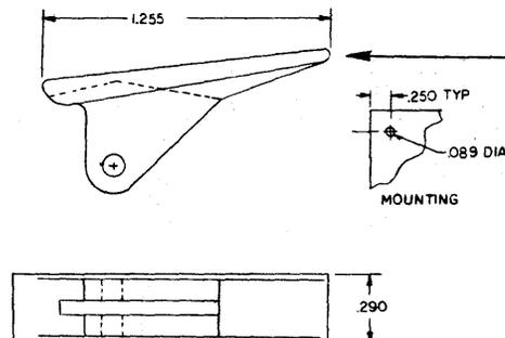
**NOTE:** The half-board card extractor (PN00-00296-00) is the same as the full-board extractor, except .130 inches of material are removed from the tip of the extractor.
