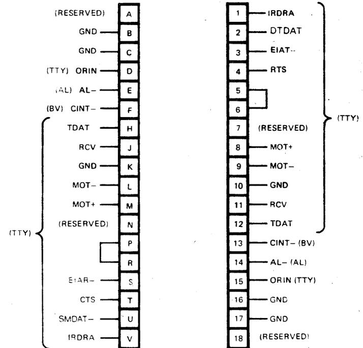
Figure 6-3. Option Board Connector J2 Pin Assignments
