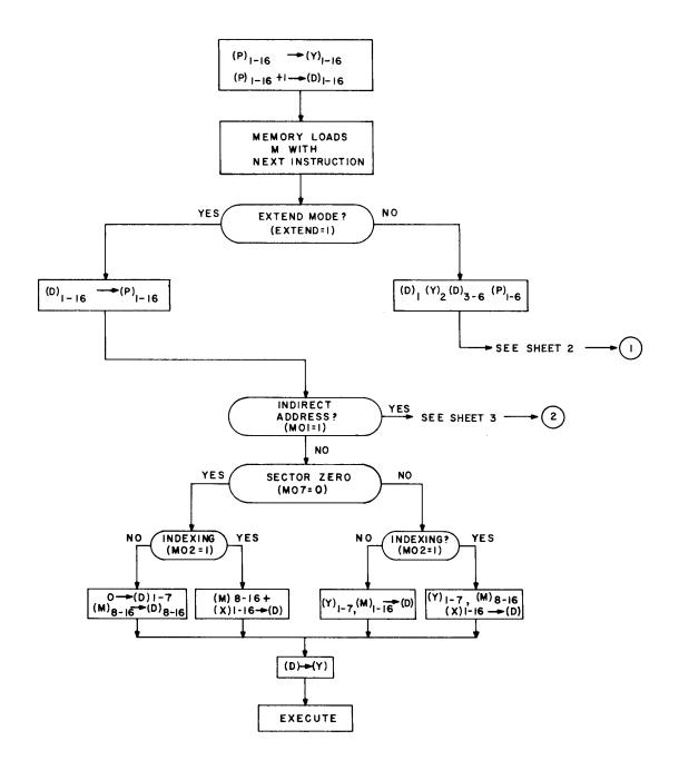
Figure 2-1. Operation of a System with Extended Addressing, Flow Diagram (Sheet 1 of 3)
