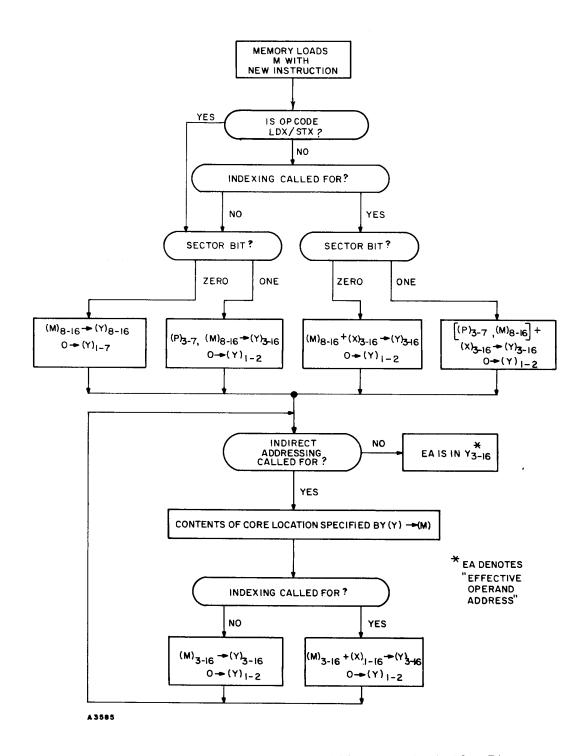
Figure 1-15. Fetch, Indexing, and Indirect Addressing, Logic Flow Diagram
