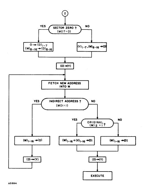
Figure 2-1. Operation of a System with Extended Addressing, Flow Diagram (Sheet 3 of 3)
