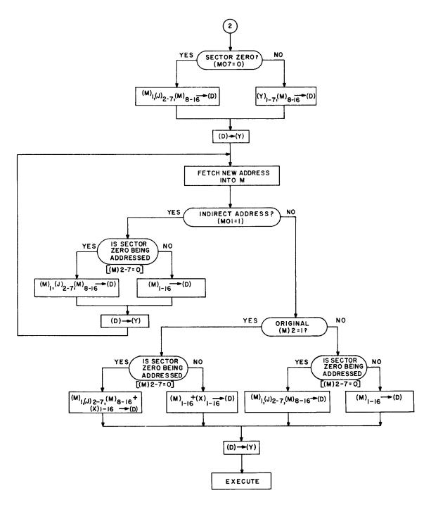
Figure 2-2. Operation of a System with Memory Lockout and up to 32K of Memory (Sheet 3 of 3)
