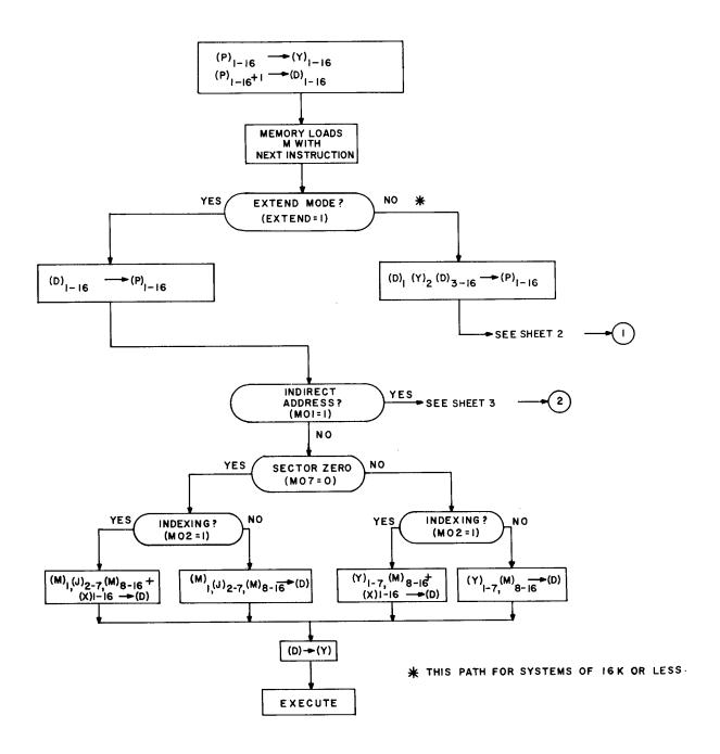
Figure 2-2. Operation of a System with Memory Lockout and up to 32K of Memory (Sheet 1 of 3)
