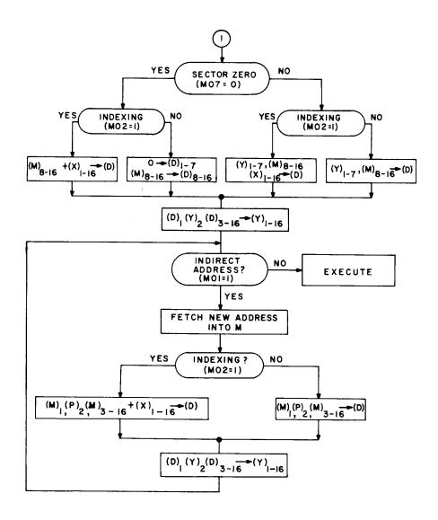
Figure 2-1. Operation of a System with Extended Addressing, Flow Diagram (Sheet 2 of 3)
