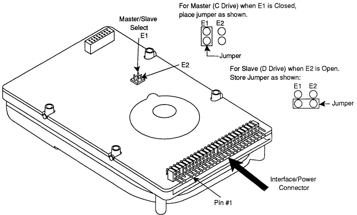
Figure 1. Master/Slave Jumper Configuration
