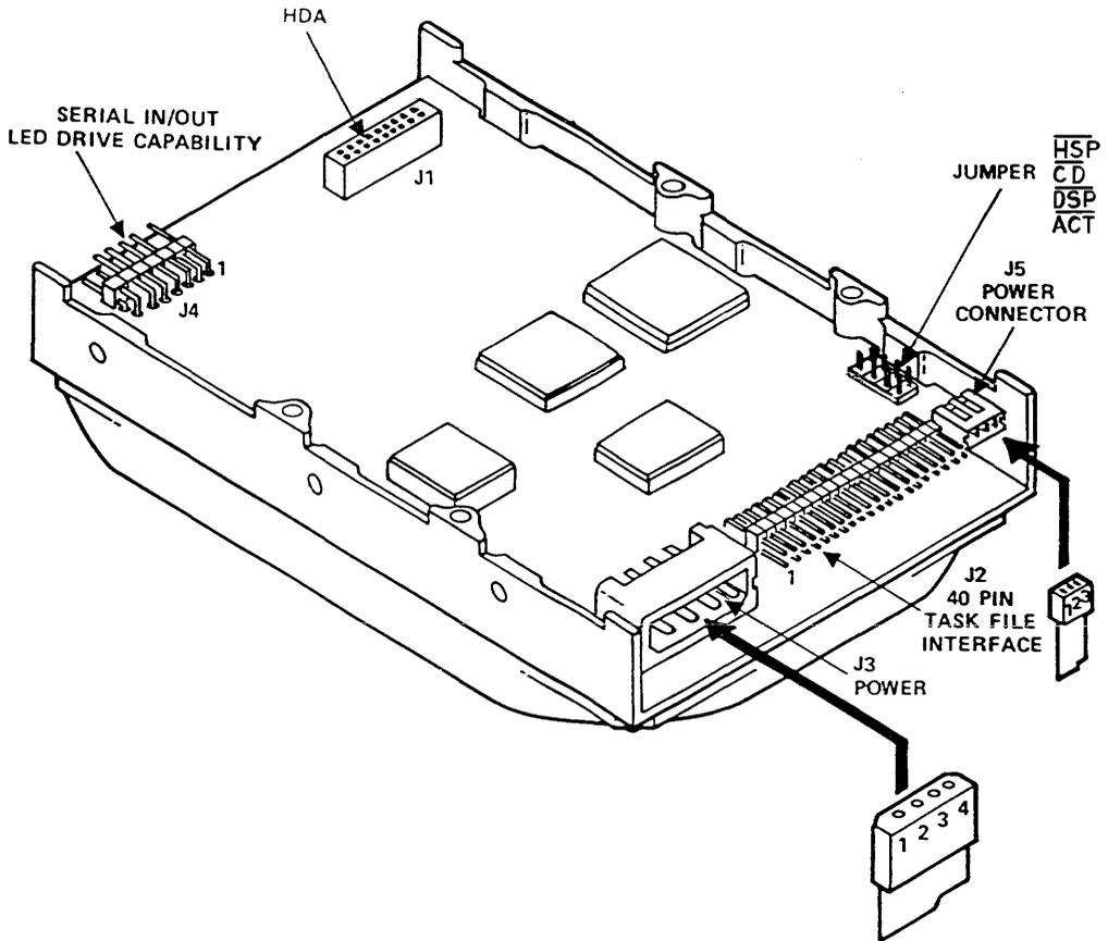
Figure 2. Connectors and Jumpers
