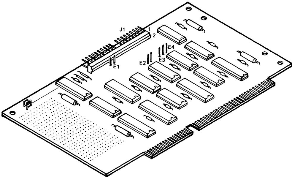
Figure A-2 AT Adapter Card Layout
