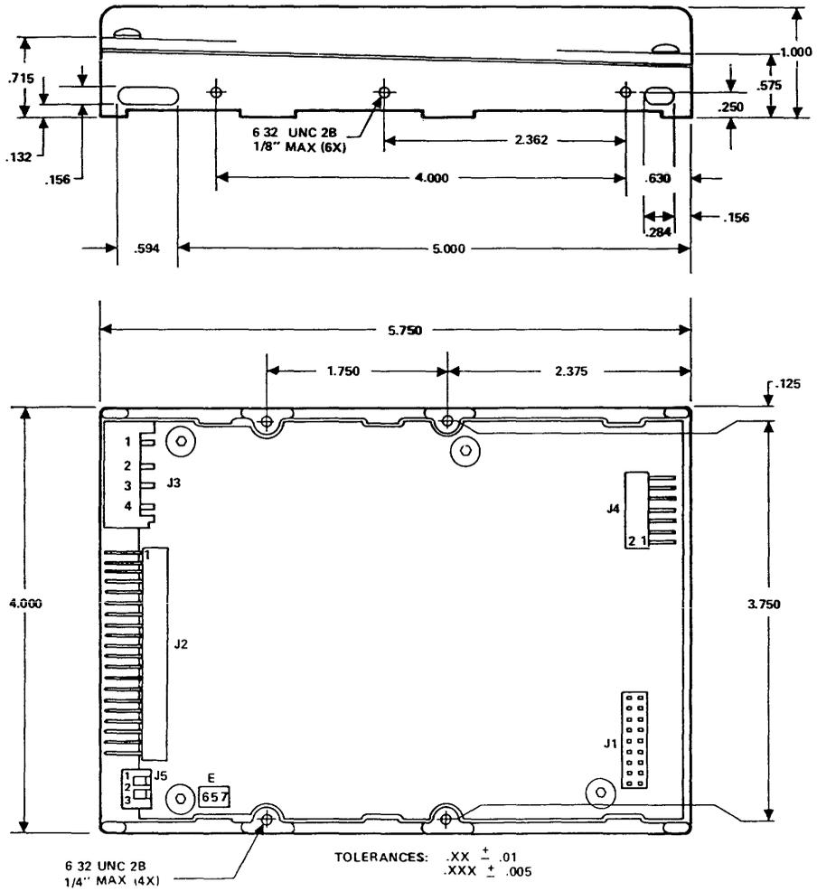
Figure 1. Mounting Configuration
