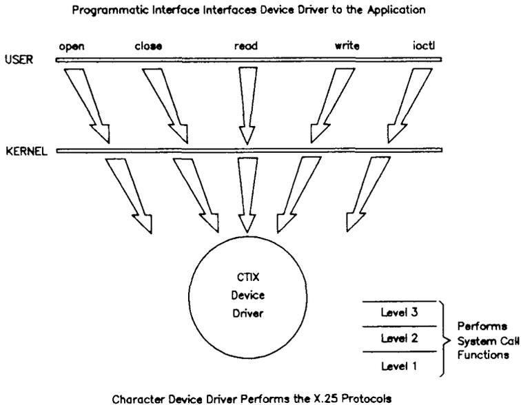
Figure 4-1. Relationship Between the Programmatic Interface and the Device Driver
