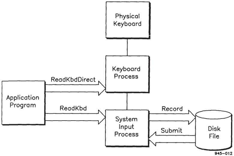
Figure 10-2. System Input Process
