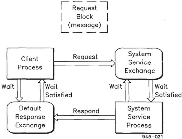
Figure 29-1. Interaction of Client and System Service Processes
