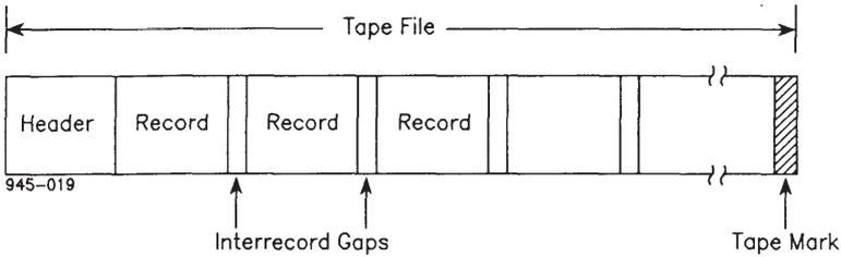
**Figure 18-5. Detail of a Half-Inch Tape File**
