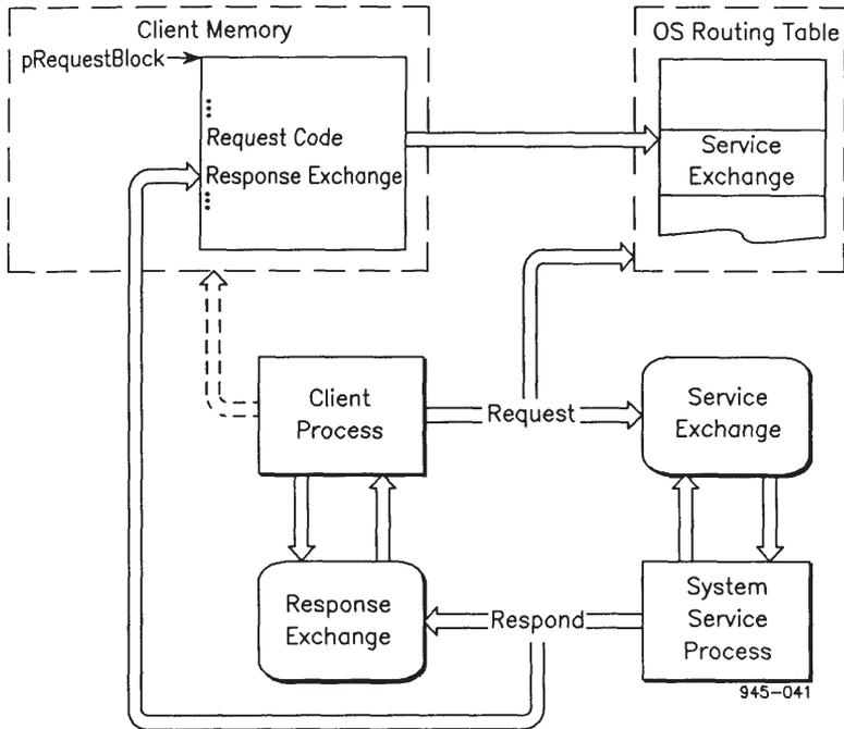
Figure 31-1. Interaction of Client and System Service Processes
