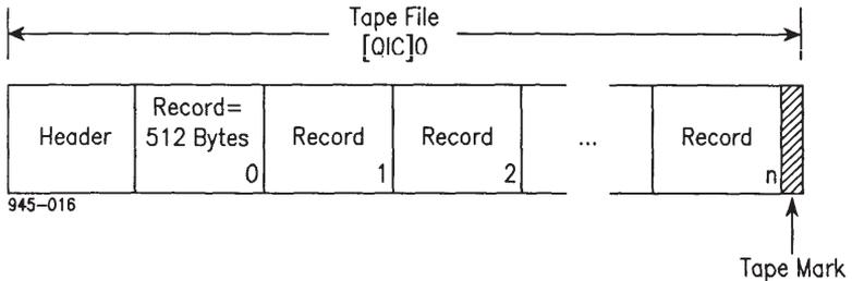
Figure 18-2. Detail of a QIC Tape File
