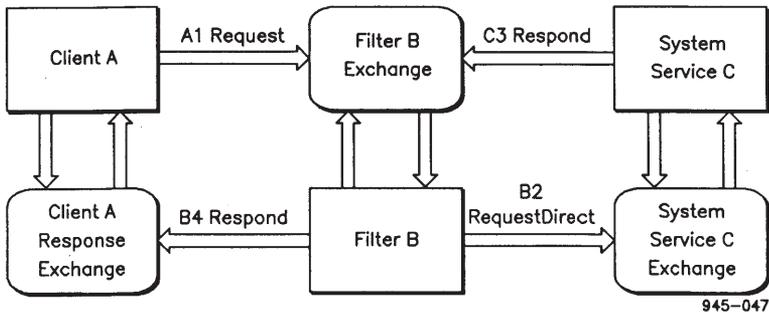
Figure 31-8. Two-Way Pass-Through Filter
