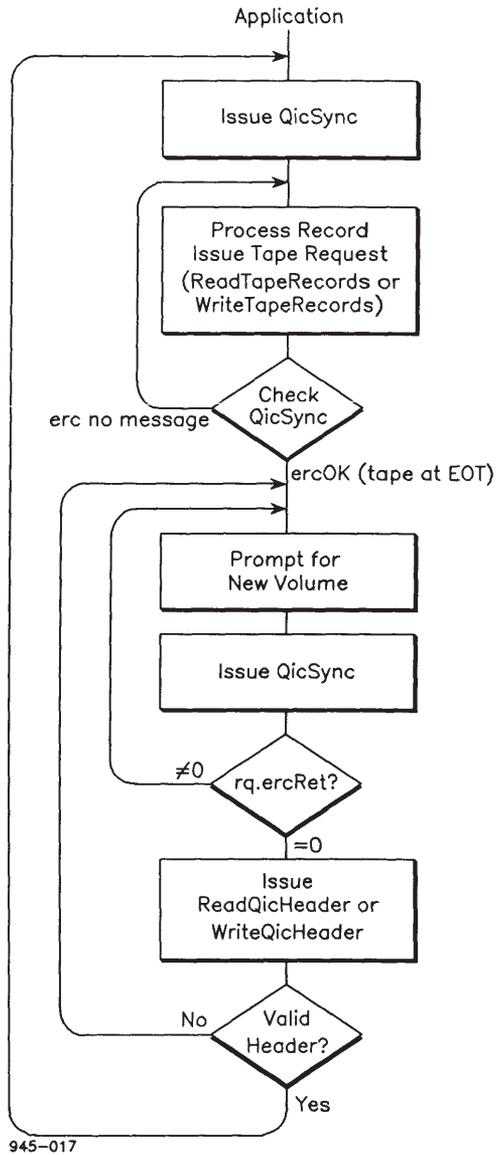
Figure 18-3. Multicartridge QIC Tape Operation Sequence
