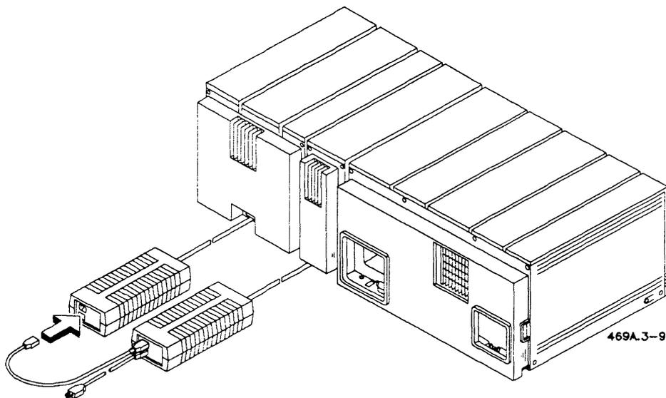
**Figure 3-9. Connecting Two Power Bricks**
