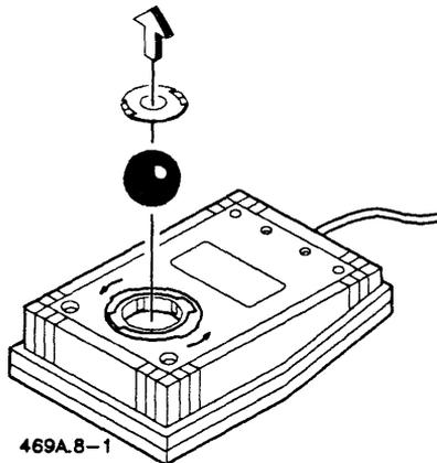
**Figure 8-1. Removing the Tracking Ball**
