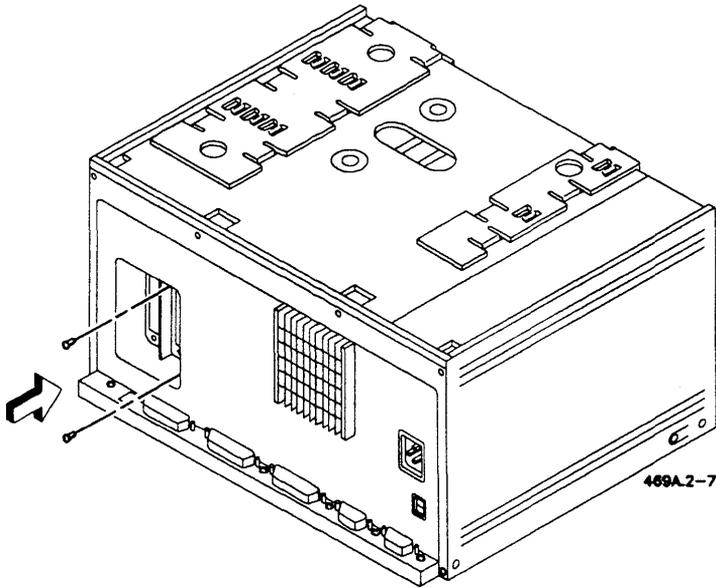
**Figure 2-7. Replacing the I/O Connector Screws**
