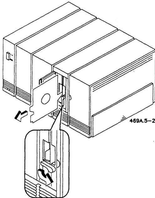
**Figure 5-2. Removing the Drive Protect Card**
