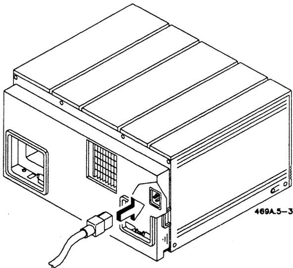
**Figure 5-3. Attaching the Power Cord**
