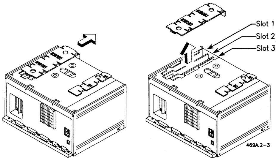
**Figure 2-3. Removing the Metal Cap (X-Bus Option Card)**
