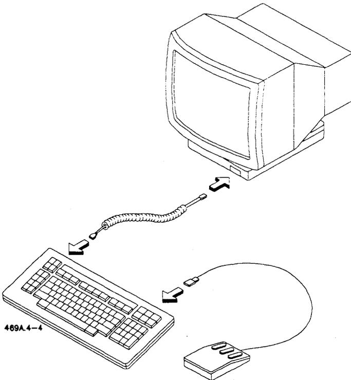
**Figure 4-4. Connecting the Keyboard and Mouse**
