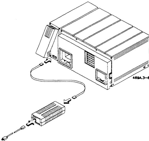
**Figure 3-8. Attaching a Power Brick**
