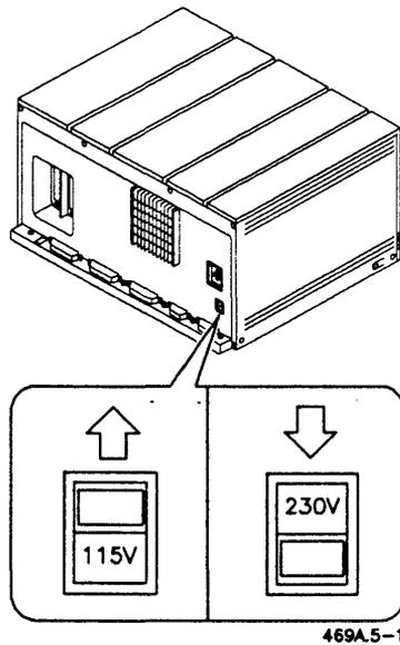
**Figure 5-1. Voltage Select Switch Settings**
