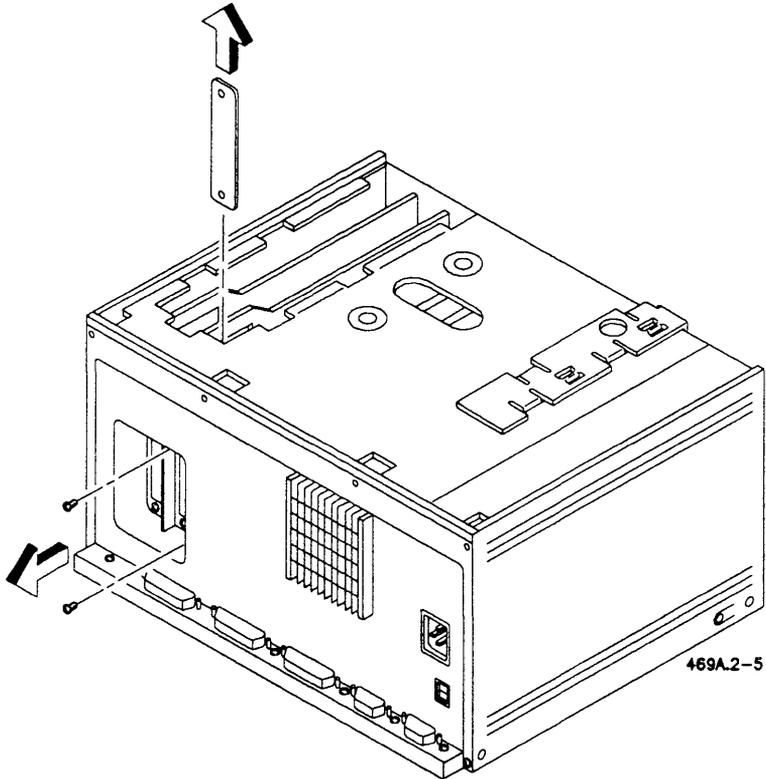
**Figure 2-5. Removing the I/O Cap**
