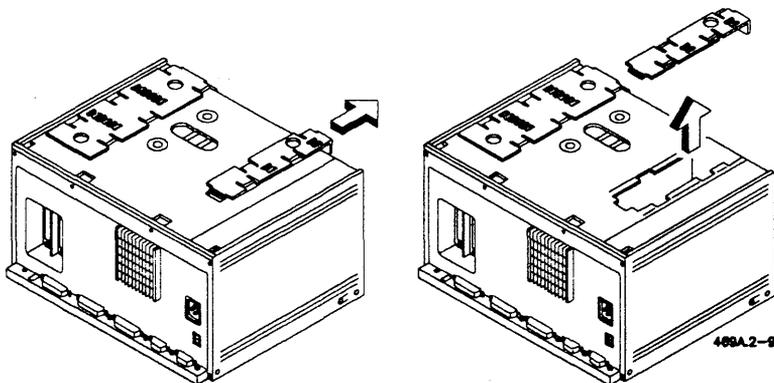
**Figure 2-9. Removing the Metal Cap (Memory Card)**
