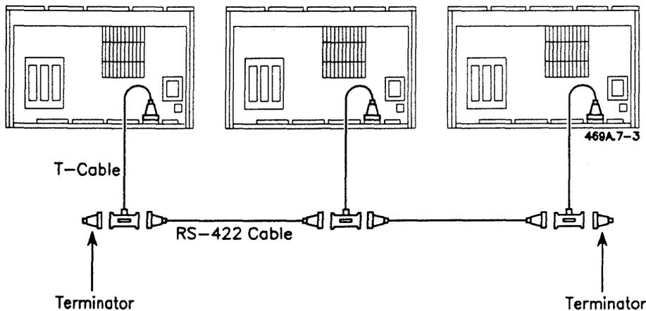
**Figure 7-3. RS-422 Cabling With T-Cables**
