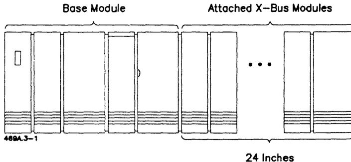
**Figure 3-1. Length of Attached X-Bus Modules**
