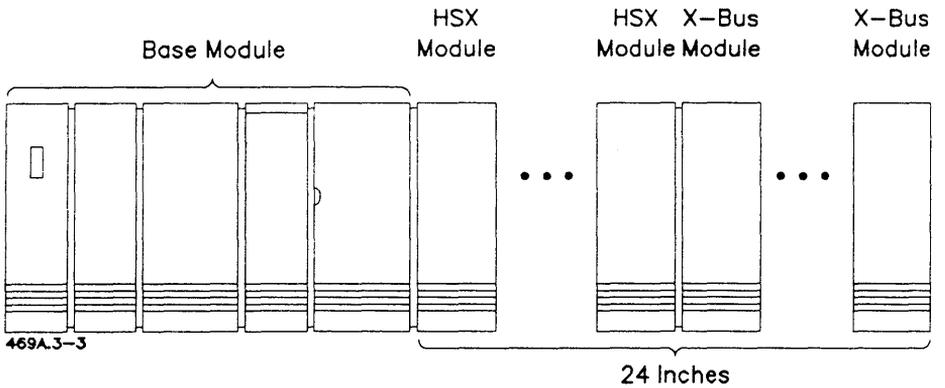
**Figure 3-3. Placement of HSX (SCSI) and X-Bus Modules Without an HSD Module**
