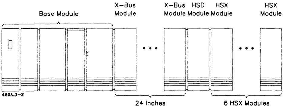
**Figure 3-2. Placement of HSX (SCSI) and X-Bus Modules With an HSD Module**
